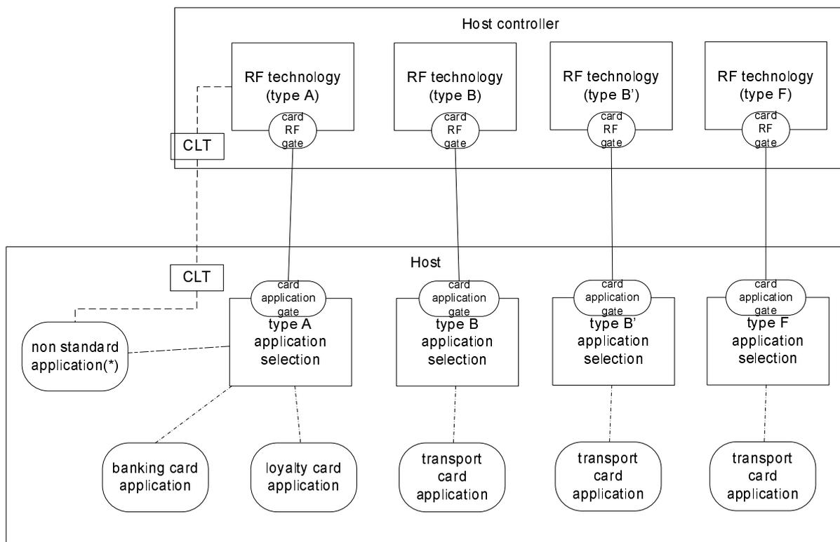
NOTE: Non-standard applications refer to type A contactless card applications that indicate "not compliant with ISO/IEC 14443-4 [7]" in the SAK according to ISO/IEC 14443-3 [6].
