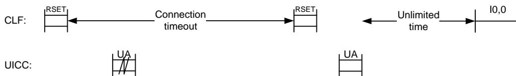
Figure 10.5: Link establishment restart after UA loss
