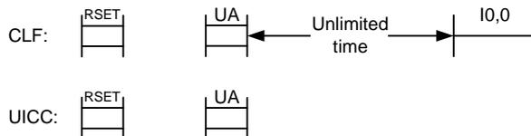
Figure 10.6: Link establishment with crossover RSET frames
