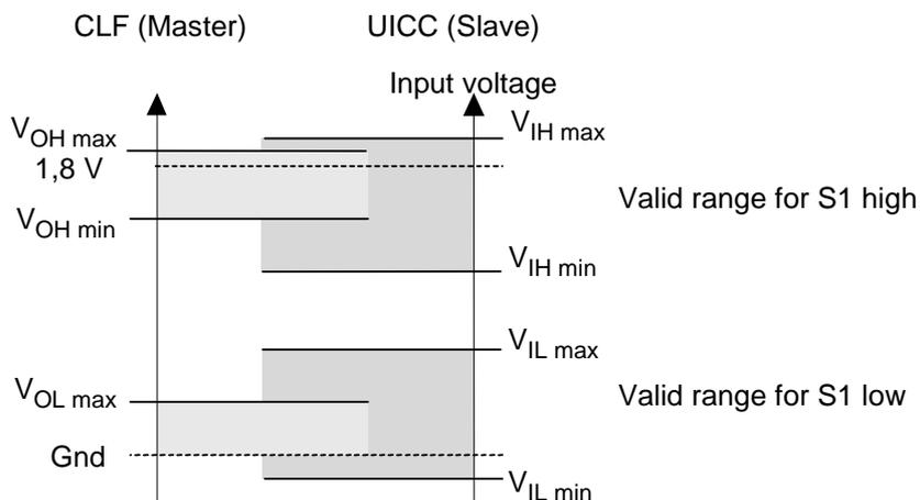
**Figure 7.1: Voltage definitions for the signal S1**
