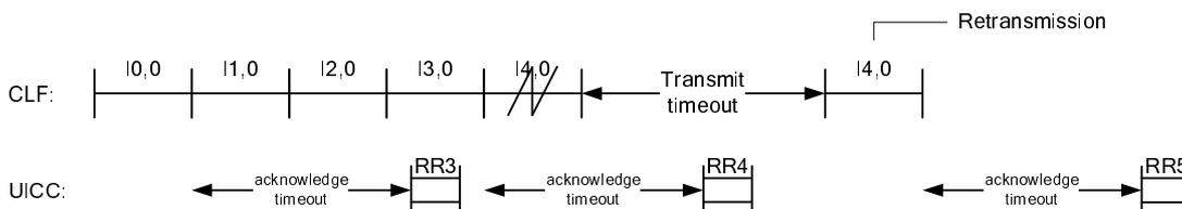
**Figure 10.16: Last frame loss in one way data flow**
