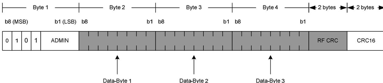
**Figure 11.4: ISO/IEC 18092 [8] 212 kbps/424 kbps passive mode byte arrangement in a CLT frame (example)**
