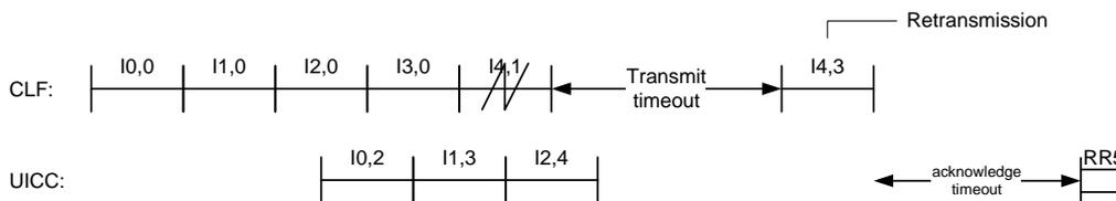
**Figure 10.15: Last frame loss in piggybacking situation**
