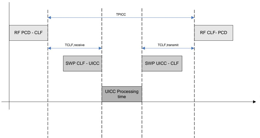
NOTE: SWP CLF-UICC and SWP UICC-CLF represent the time taken to transmit the data over SWP and are included in the  $T_{CLF,receive}$  and  $T_{CLF,transmit}$  times.
