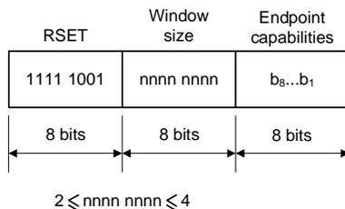
**Figure 10.2: RSET frame payload**
