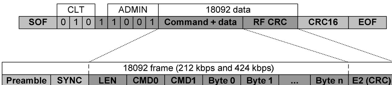
Figure 11.3: ISO/IEC 18092 [8], 212 kbps/424 kbps passive mode data in a CLT frame (example)
