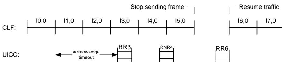
**Figure 10.17: Stop and resume traffic at UICC request**
