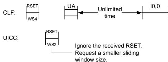
**Figure 10.7: Link establishment with sliding window size of 2**
