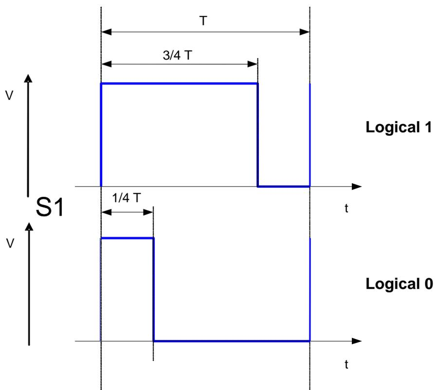
**Figure 8.1: Bit-coding of S1**
