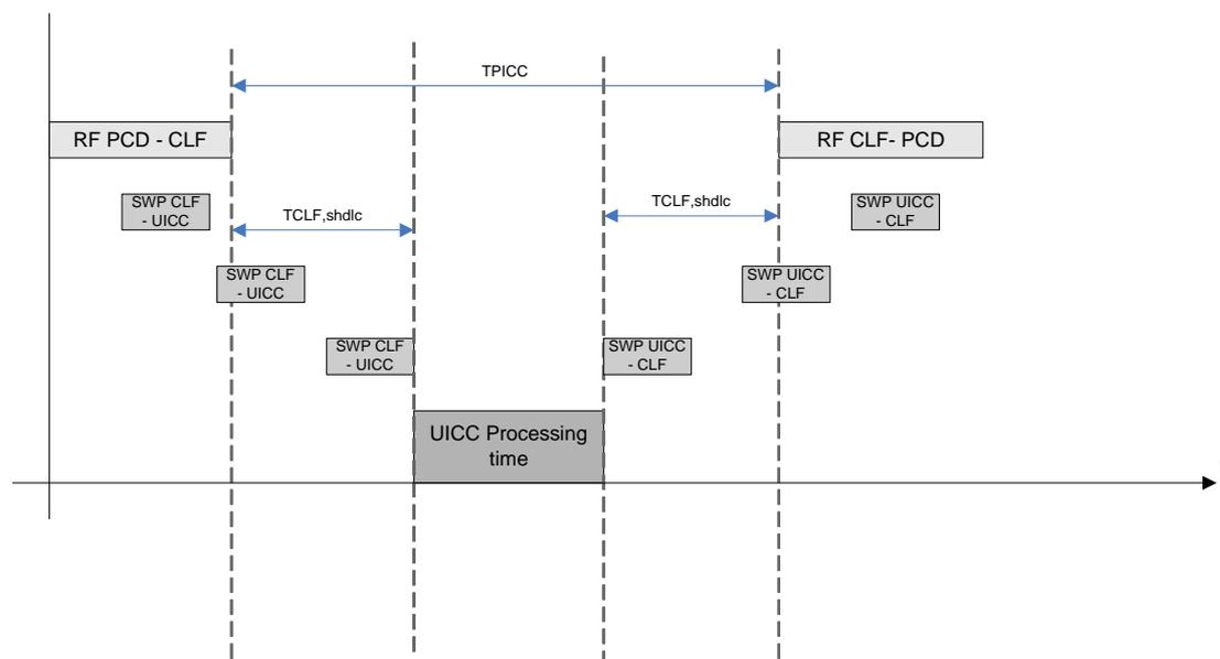
Figure 12.5: SHDLC transmission timings
