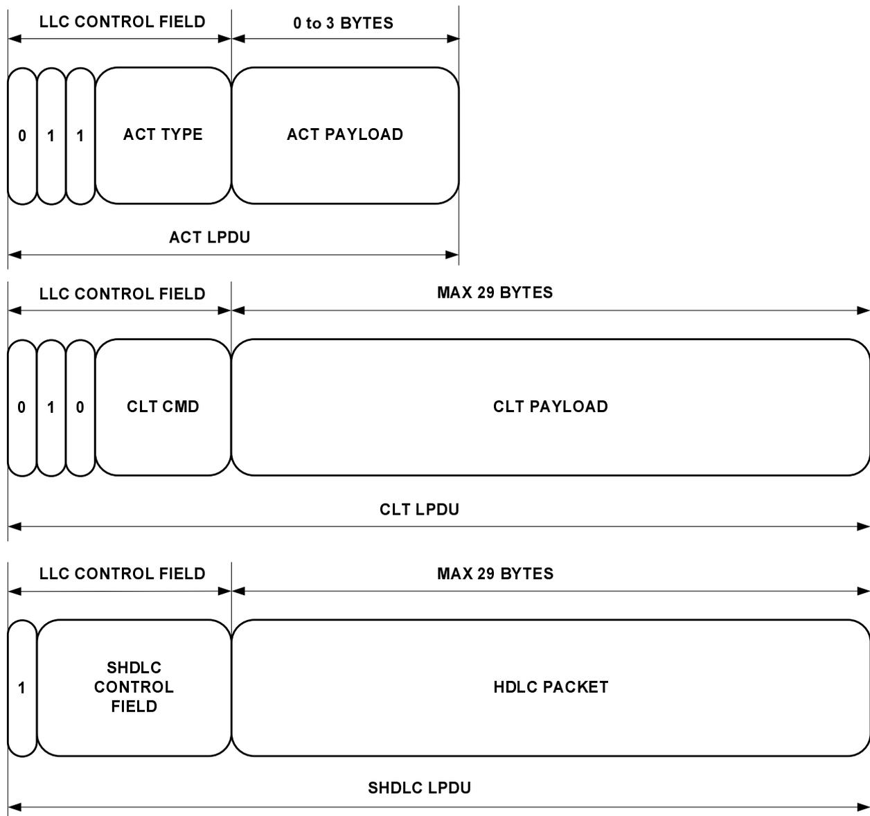
Figure 9.5: LPDU structure of the 3 defined LLC layers
