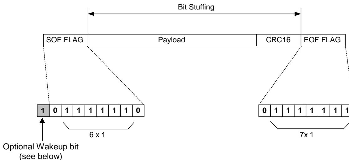
**Figure 9.3: Frame structure sent by slave**
