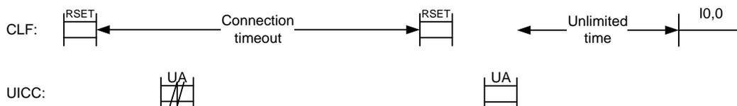
Figure 10.5: Link establishment restart after UA loss
