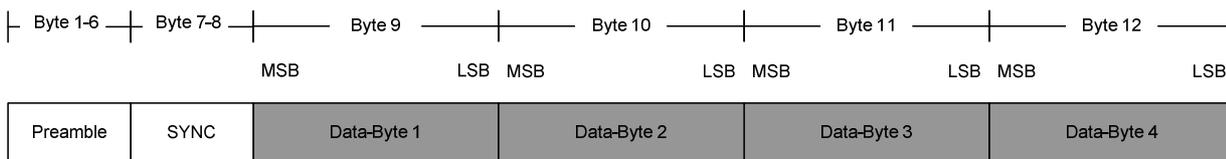
**CLT LPDU via SWP in "ISO/IEC 18092 [8] 212/424 kbps passive mode based frame" structured:**
