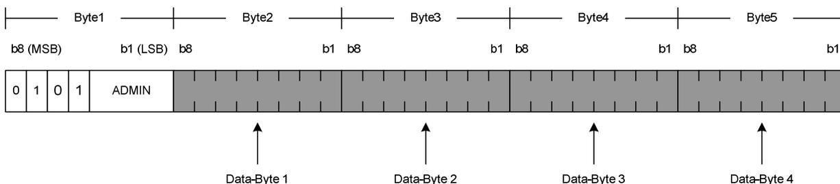
Figure 11.4: Type F byte alignment in CLT frame
