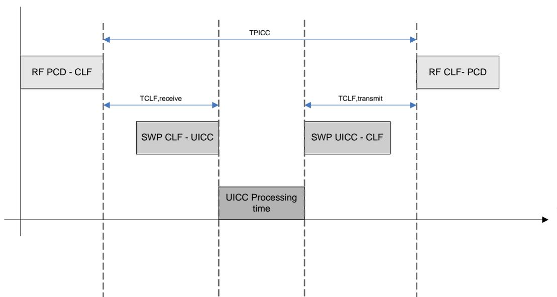
NOTE: *SWP CLF-UICC* and *SWP UICC-CLF* represent the time taken to transmit the data over SWP and are included in the  $T_{\text{CLF,receive}}$  and  $T_{\text{CLF,transmit}}$  times.
