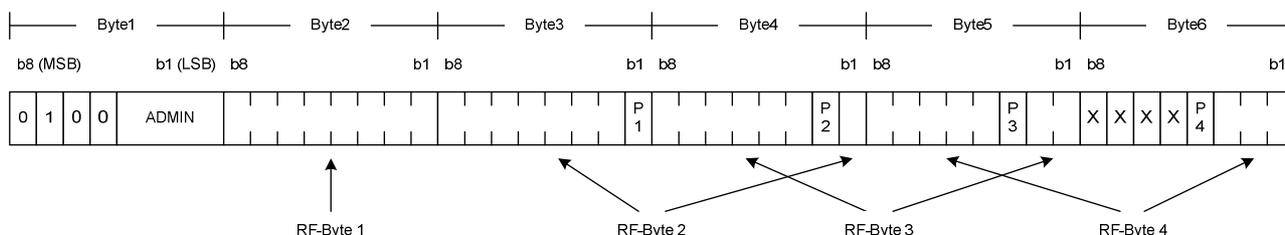
**Figure 11.2: Examples for a "Type A structured" CLT frame**
