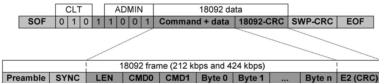
Figure 11.3: Type F structured CLT frame
