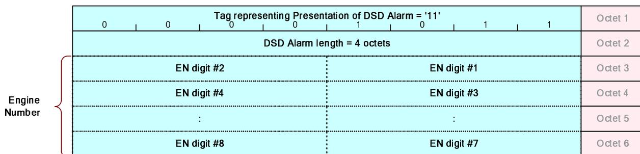
Figure 10: DSD alarm tag layout
