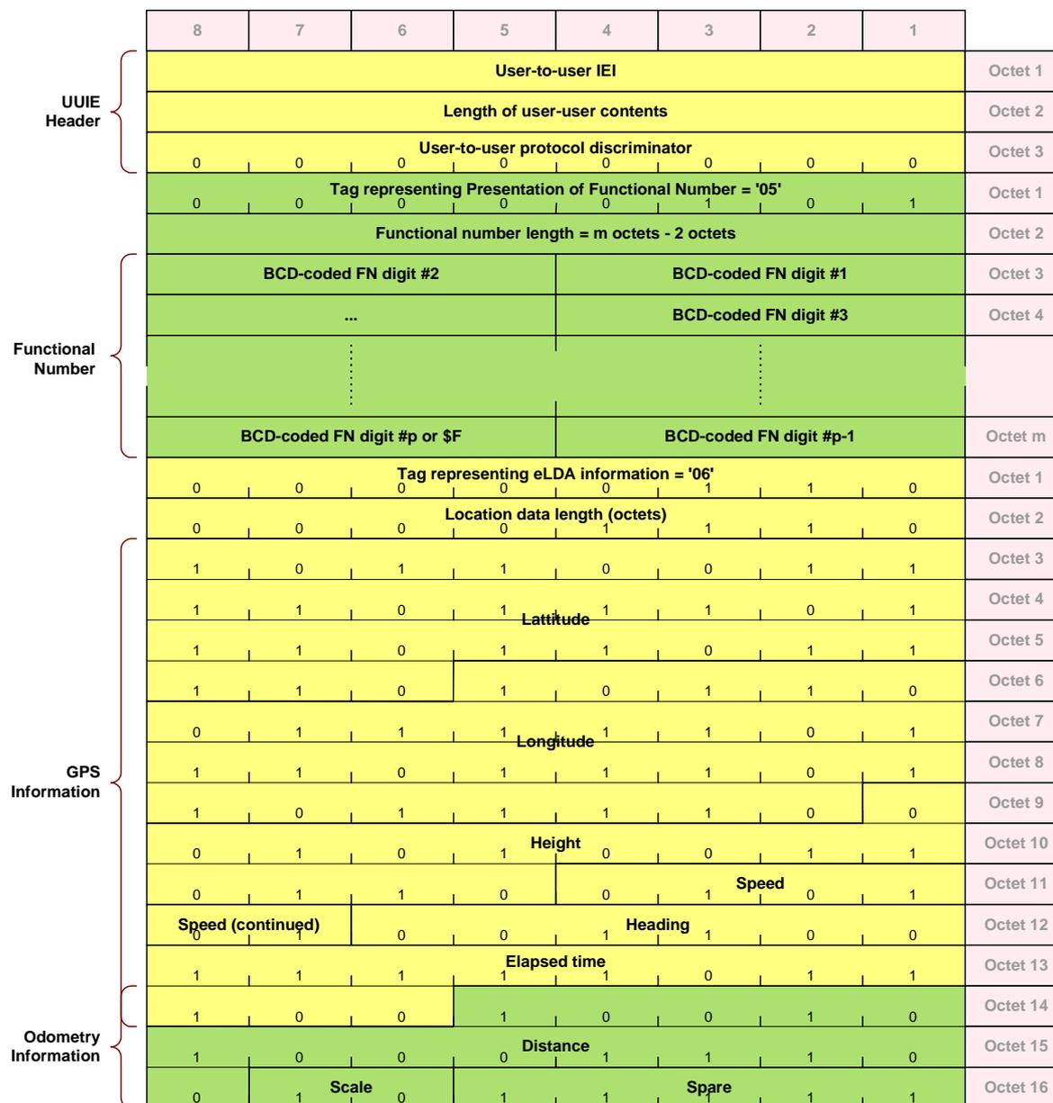
Figure 15: Arrangement of tags for train-based eLDA
