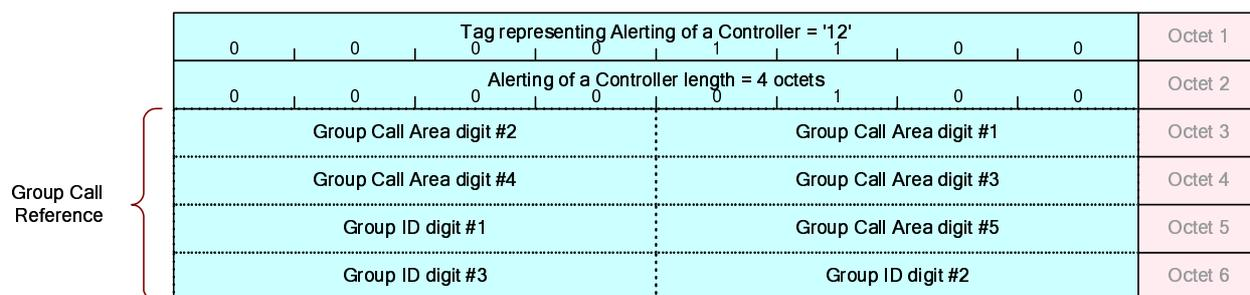
Figure 11: Alerting of a controller tag layout
