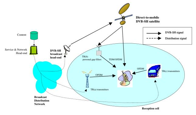
Figure 1: Overall DVB-SH system architecture
