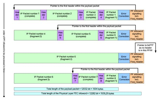
Figure 3: Description of IP packet encapsulation
