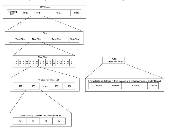
Figure 8 shows the sub-partitioning of a C-TS frame into its smaller units and into logical content.
