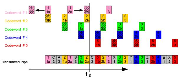
Figure 11: Other example of disperser reconfiguration
