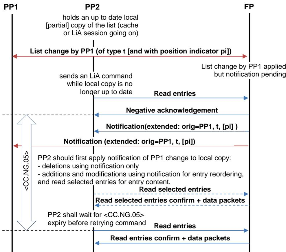
**Figure I.2: Solution to the problem of Use case 1a: the FP sends a negative acknowledgement to the read entries command and broadcasts pending notification(s)**
