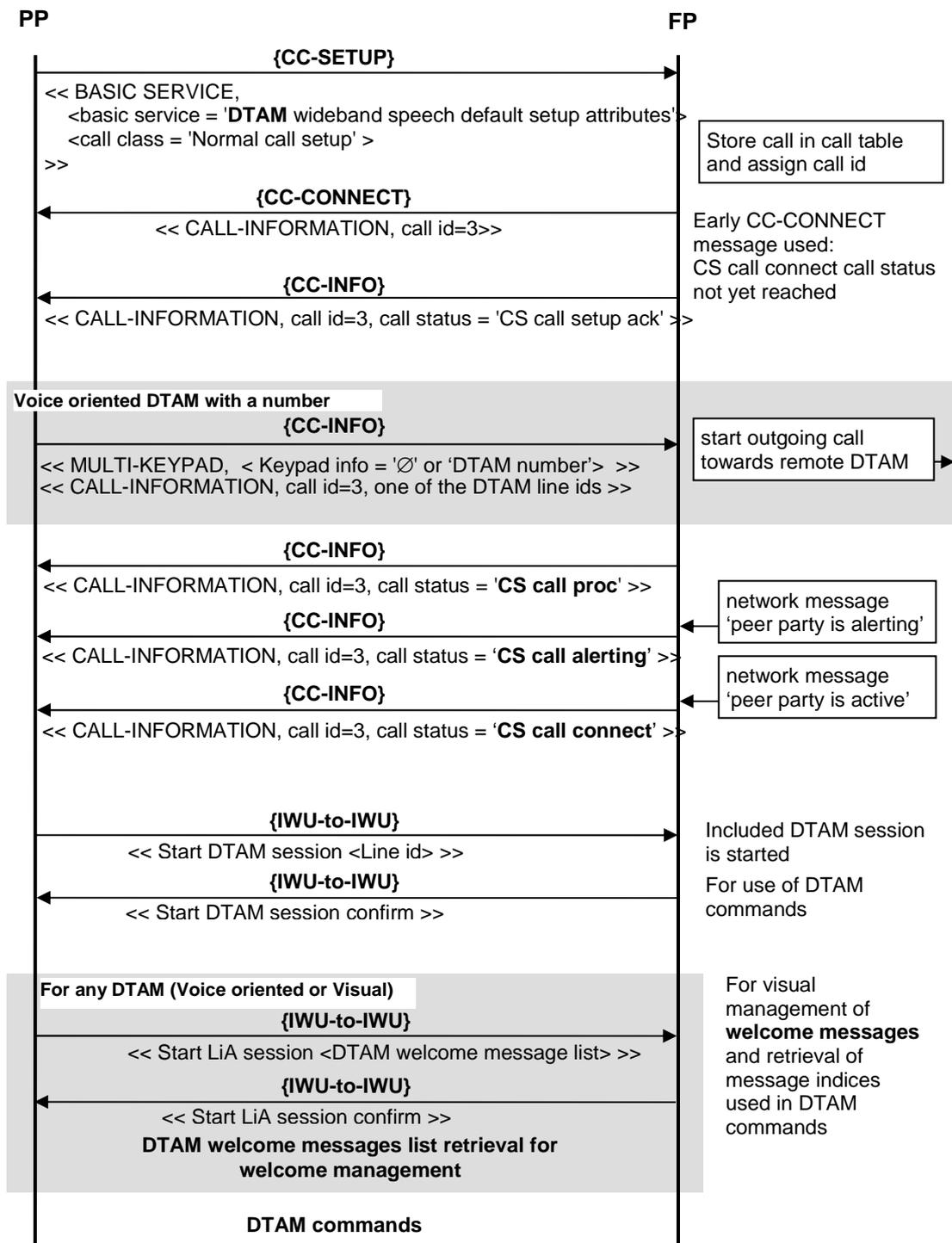
Figure G.2: Voice oriented remote DTAM (with a DTAM number)
