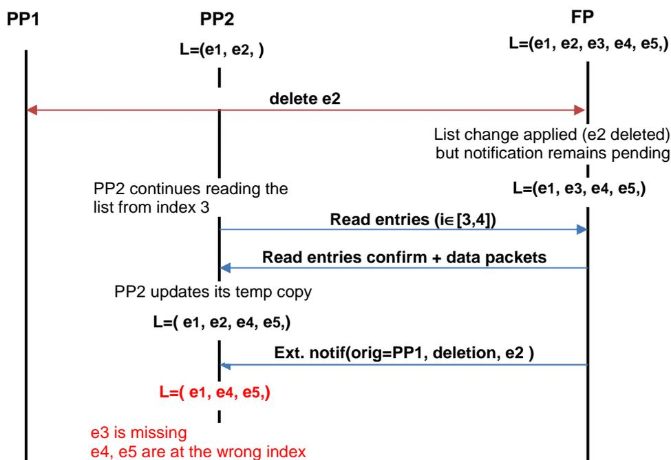
Figure I.1: Problem of PP2 reading entries while a notification for a change in the list (by PP1) is pending on FP side
