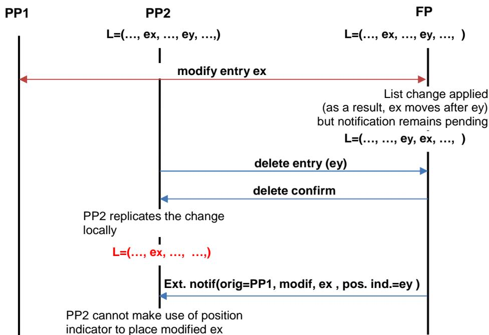
**Figure I.4: Problem of PP2 deleting an entry while a notification for a change in the list (by PP1) is pending on FP side**
