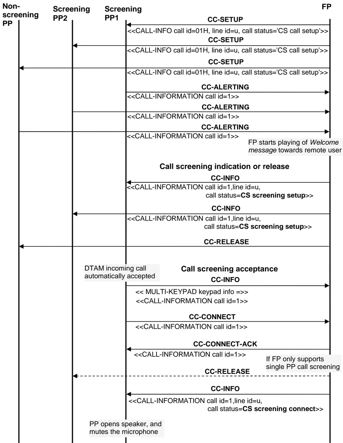
Figure 80-13: Call screening with screening and non-screening PPs
