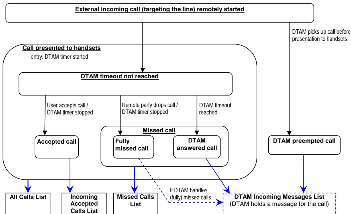
NOTE 1: Blue arrows indicate which type of call goes in which call list. They do not represent transitions (in particular because a call can belong to several lists) . A blue arrow starting at a high-level state indicates that calls from all included substates go into the pointed list.
