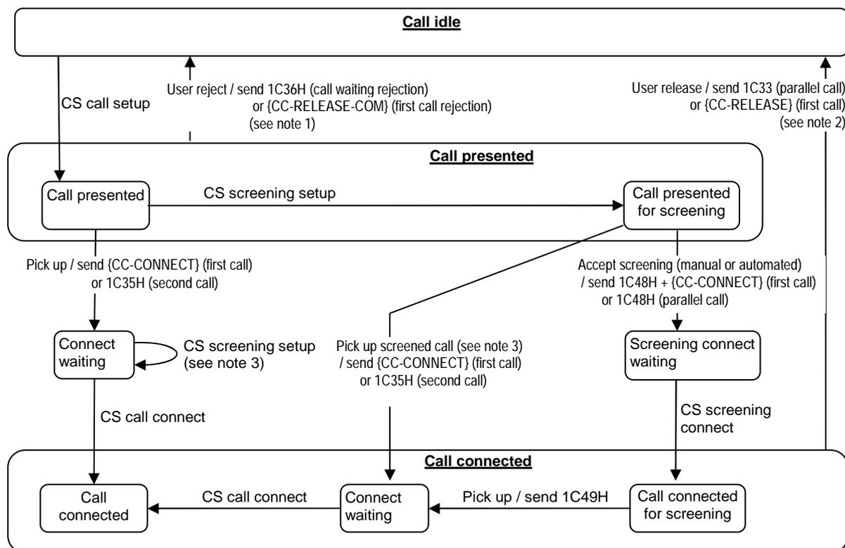
NOTE 1: Call waiting rejection (1C36H) can still be used if a parallel call is presented for screening ('CS screening setup' has been received).
