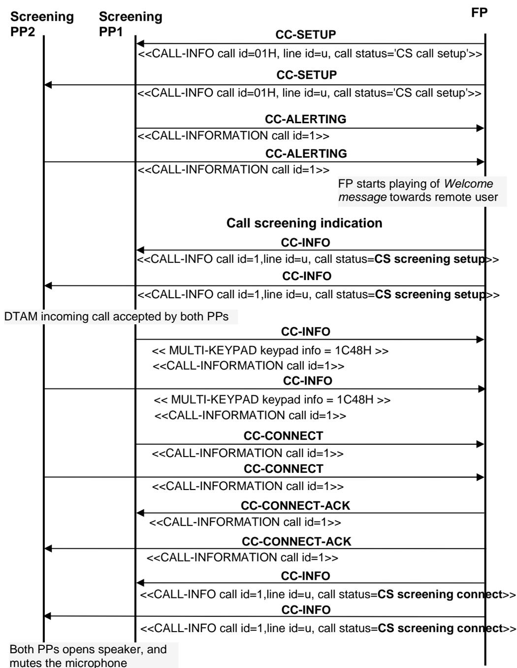
Figure 80-14: Call screening acceptance by multiple PPs
