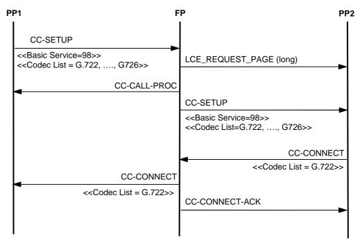
Figure 28: Internal call with codec list at call setup
