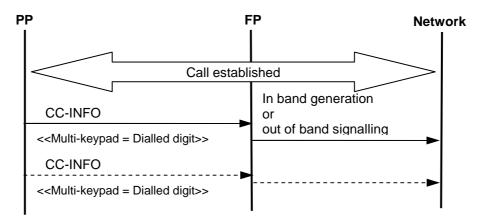
Figure 67: Sending DTMF when a call is established
