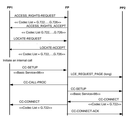
Figure 27: Internal call with no codec list at call setup
