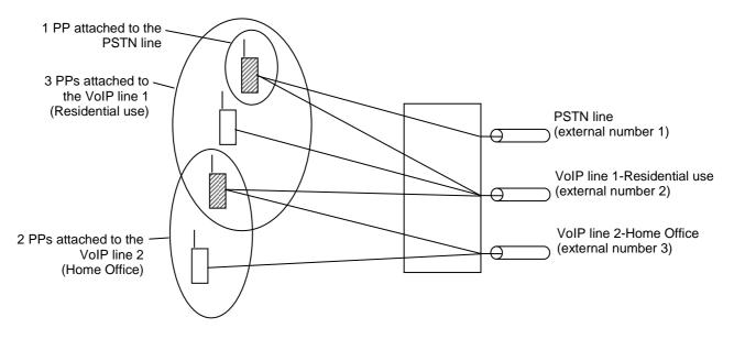
Figure 52: A multiple-call line with three simultaneous calls
