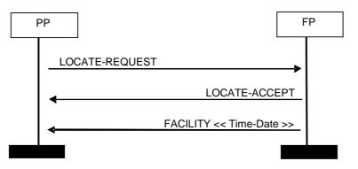
Figure B.8: Date-time synchronization when the PP is switched on
