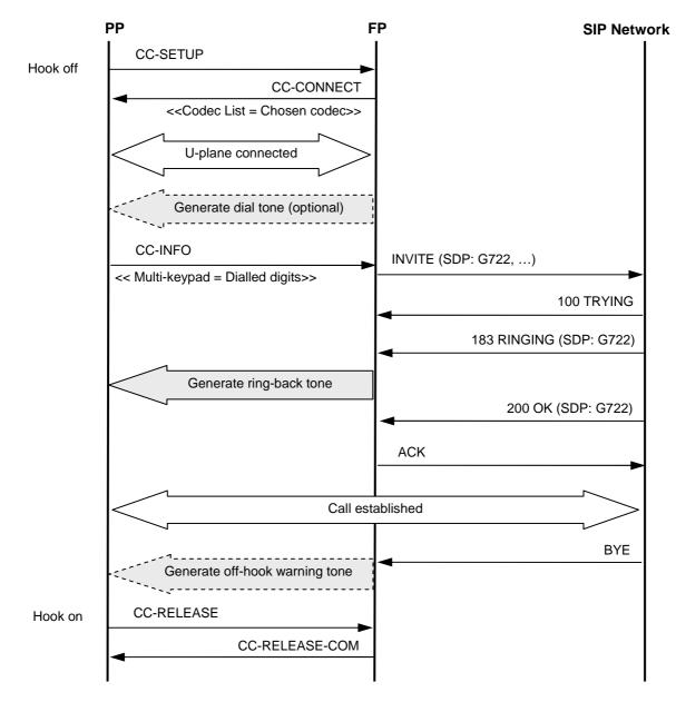
Figure 74: FP provides tones during external call using {CC-CONNECT}
