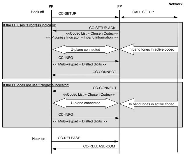
Figure 77: Network provides tones during PSTN external call
