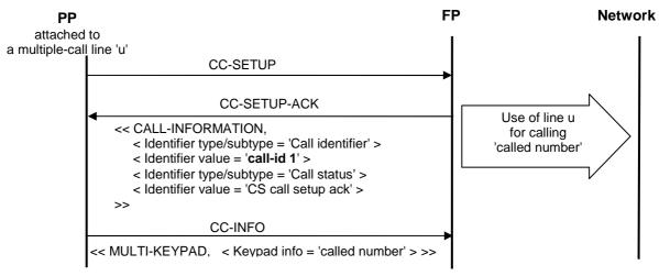
Figure C.9: First outgoing call on the line or system
