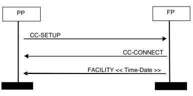
Figure B.9: Date-time synchronization using call connection
