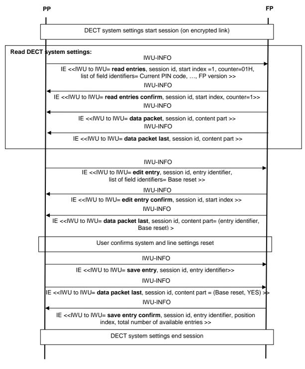
Figure C.32: Resetting the base
