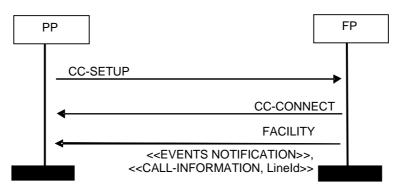
Figure B.4: Event notification using call connection
