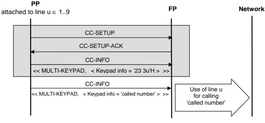
Figure 36: Line identification for a first external outgoing call, using the << MULTI-KEYPAD>> method
