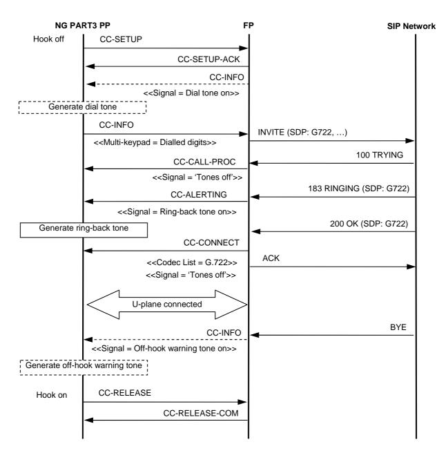
Figure 71: NG PART3 PP provides tones during SIP external call
