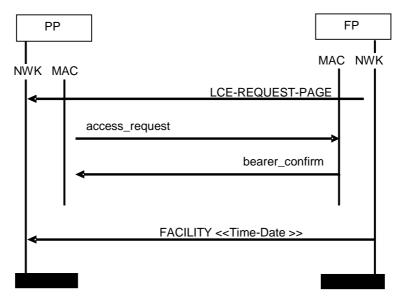
Figure B.6: Date-time synchronization when there is no existing connection
