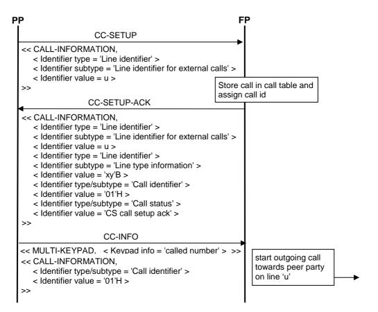
Figure 33: Line identification in {CC-SETUP}
