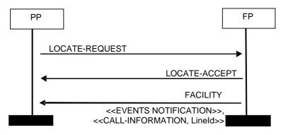
Figure B.3: Event notification when the PP is switched on
