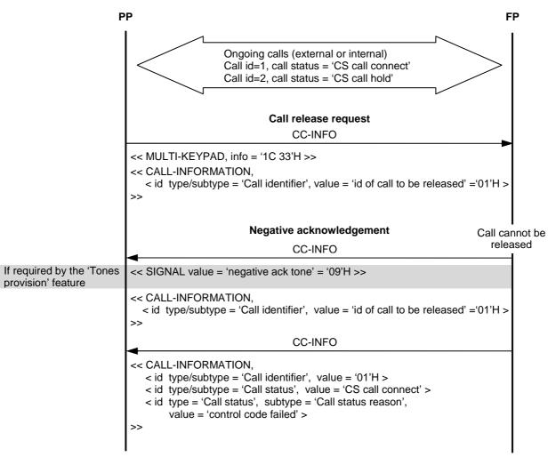
Figure 9: Failing call release request from the PP
