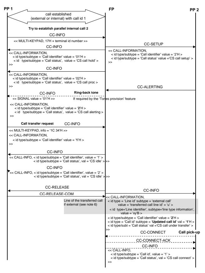
Figure 18: Unannounced call transfer (example with internal target PP2): "call transfer request" *before* {CC-CONNECT}
