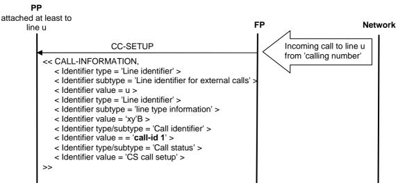
Figure C.4: First incoming call, PP attached to several lines
