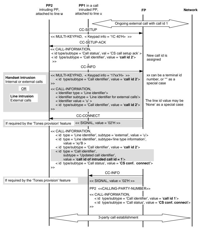
Figure 26: Successful explicit call intrusion with intrusion target in {CC-INFO}
