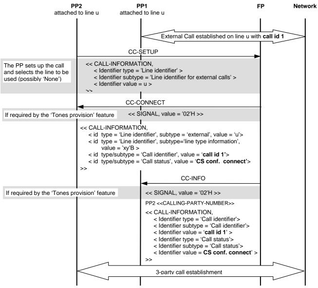
Figure 24: Successful implicit call intrusion with PP line selection in the {CC-SETUP}
