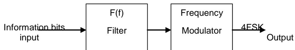
**Figure 13: 4FSK Modulator**
