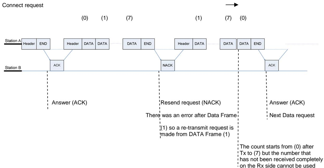
**Figure 5: Packet retransmissions**
