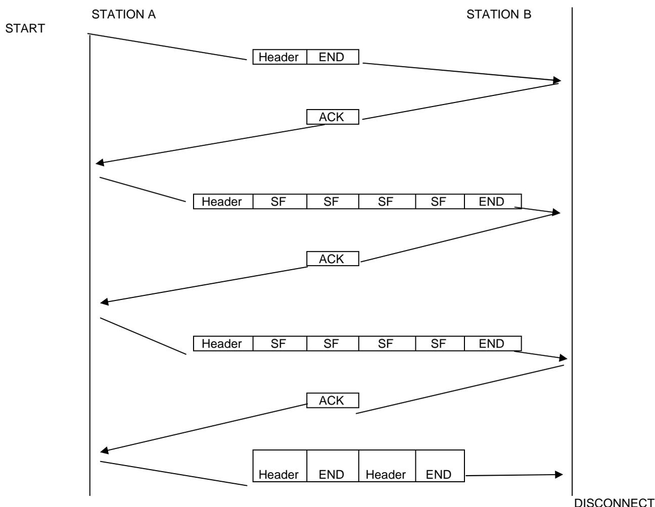
**Figure 2: Individual data call exchanges - CSF radios**
