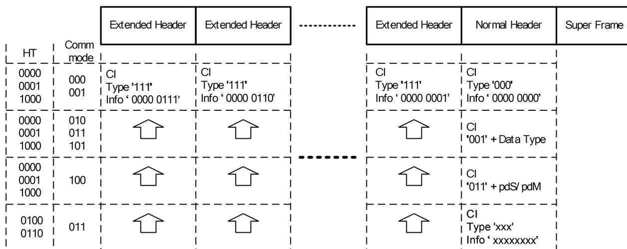
Figure 12: Extended header coding
