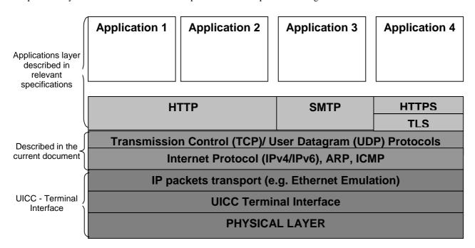
Figure 5: TCP/IP over UICC-Terminal Interface protocol stack
