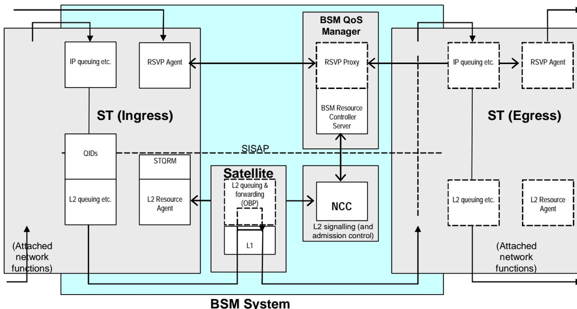
Figure 5.3: BSM Centralised RSVP Architecture (Dynamic SD Resources)
