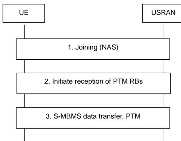
**Figure 8.2: Joining with continuation of PTM**
