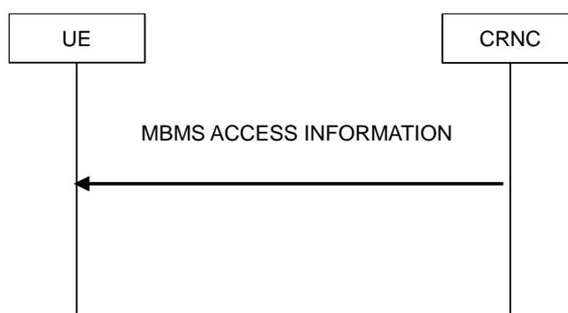
**Figure 8.16: S-MBMS Access Information signalling flow**
