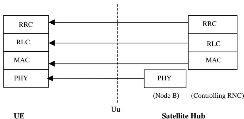
**Figure 5.5: Protocol stack for MCCH and MSCH**
