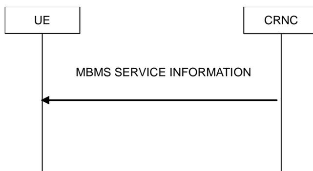
**Figure 8.14: S-MBMS service information signalling flow**
