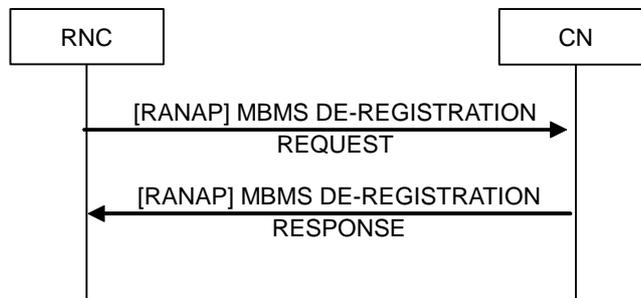
**Figure 8.8: RNC S-MBMS De-Registration procedure**
