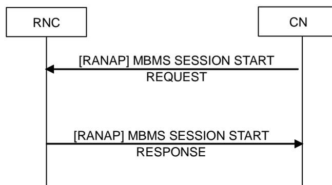
**Figure 8.4: S-MBMS Session Start procedure. Successful operation**
