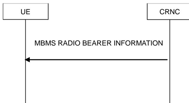
**Figure 8.15: S-MBMS radio bearer information signalling flow**
