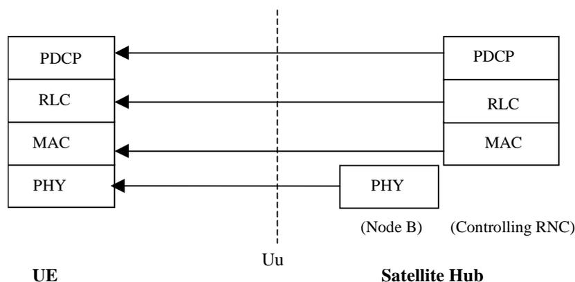
**Figure 5.4: Protocol stack for MTCH**
