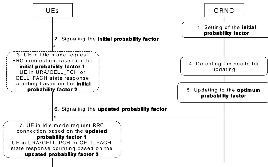
**Figure 11.1: S-MBMS Access Control Procedure**
