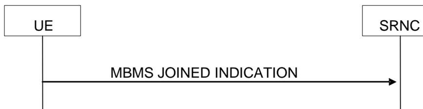
**Figure 8.18: S-MBMS joined indication signalling flow**
