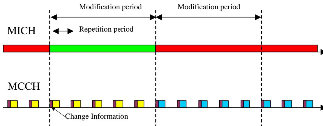
Figure 5.2: Illustration of MICH timing relative to Modification period
