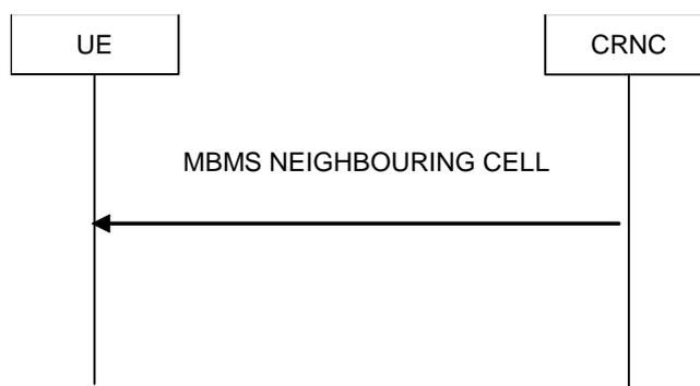
**Figure 8.17: S-MBMS Neighbouring Spot/IMR Cell Information signalling flow**
