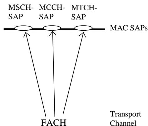
**Figure 6.1: Mapping of logical channels onto transport channels; UE side**
