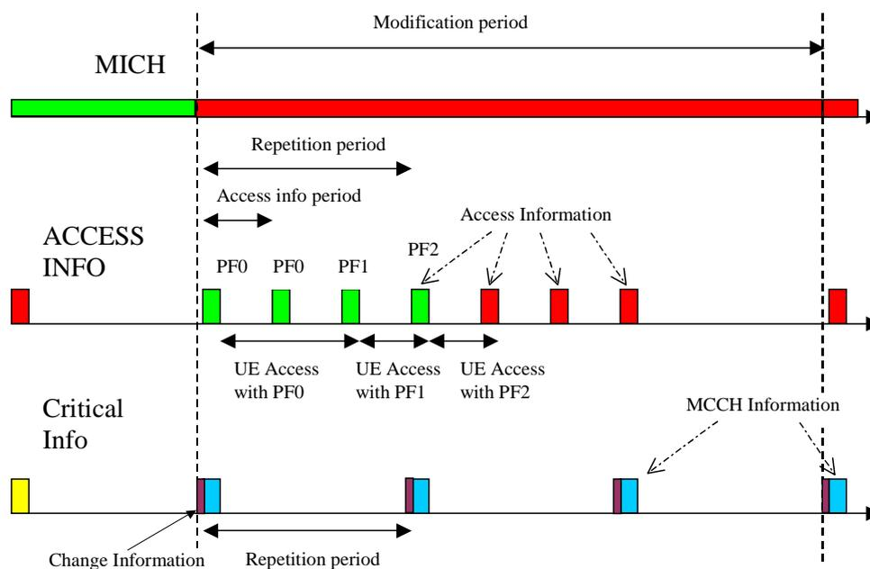
**Figure 5.3: Illustration of Access Info period during S-MBMS counting**
