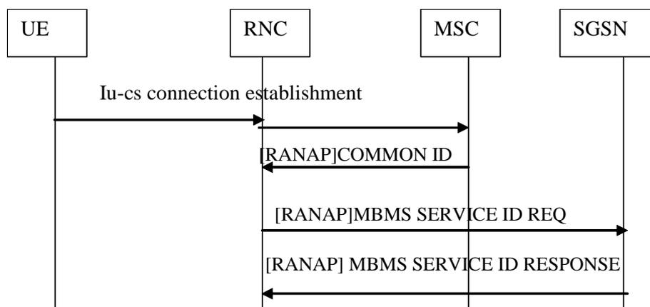
Figure 8.12: S-MBMS Service Id list over Iu signalling flow
