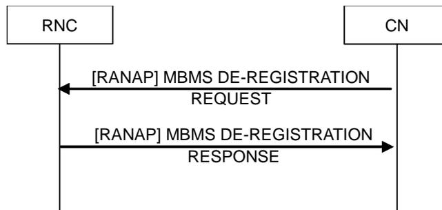
**Figure 8.9: CN S-MBMS De-Registration procedure**
