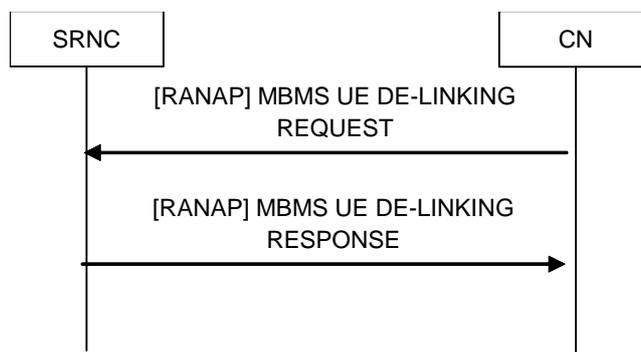
Figure 8.11: S-MBMS UE De-linking signalling flow
