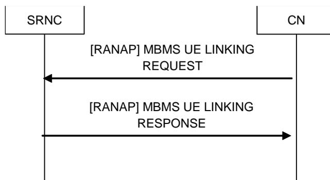
**Figure 8.10: S-MBMS UE linking signalling flow**
