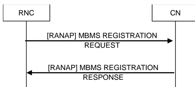
**Figure 8.7: S-MBMS Registration procedure**
