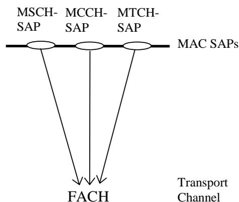
**Figure 6.2: Mapping of logical channels onto transport channels; USRAN side**
