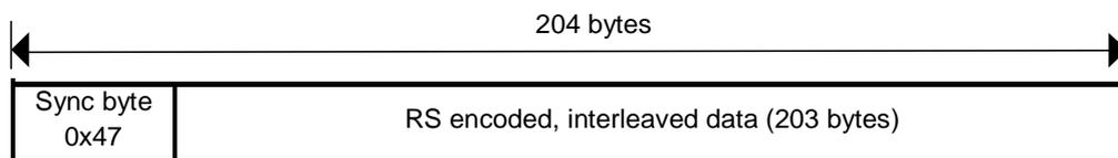
**Figure 5: Interleaved packet**
