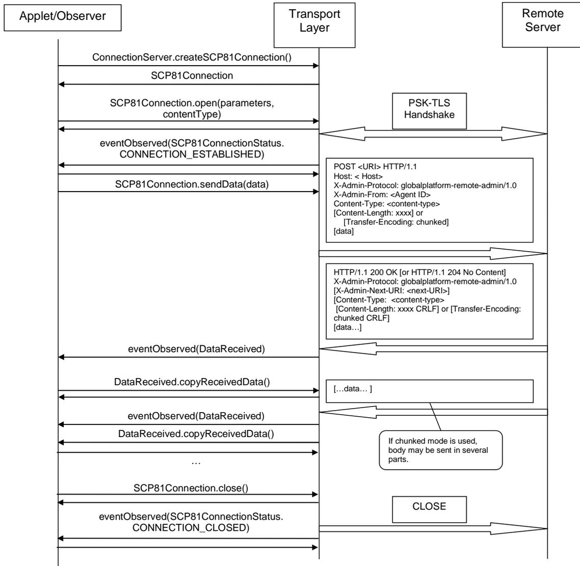
**Figure 5: SCP81Connection sequence diagram**
