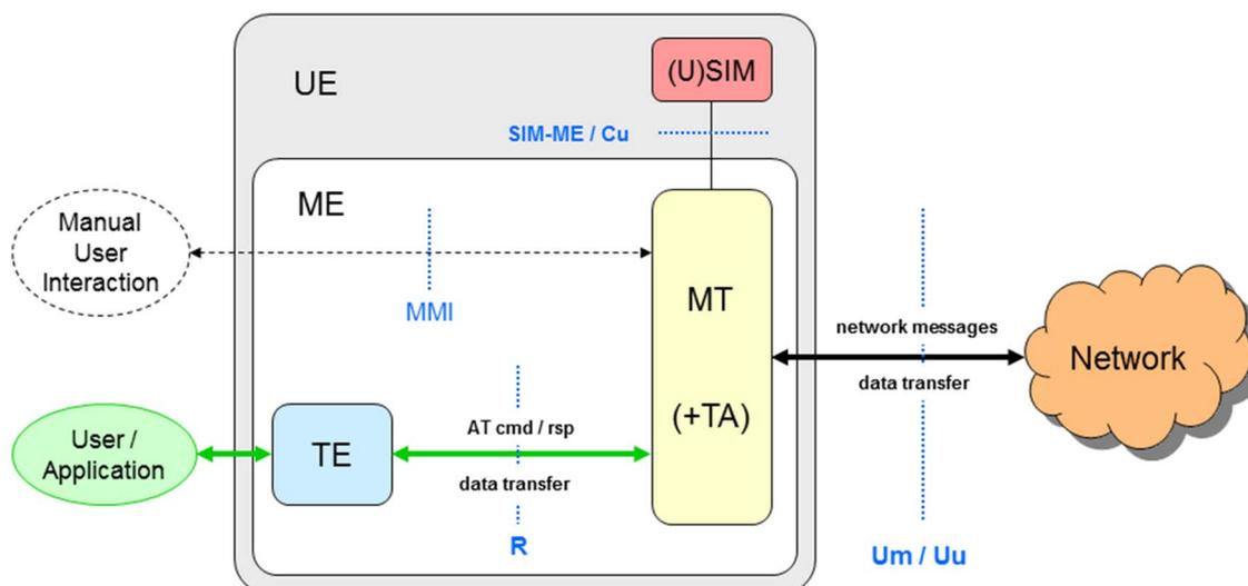
Figure 7.1: Standard 2G/3G/4G network access model
