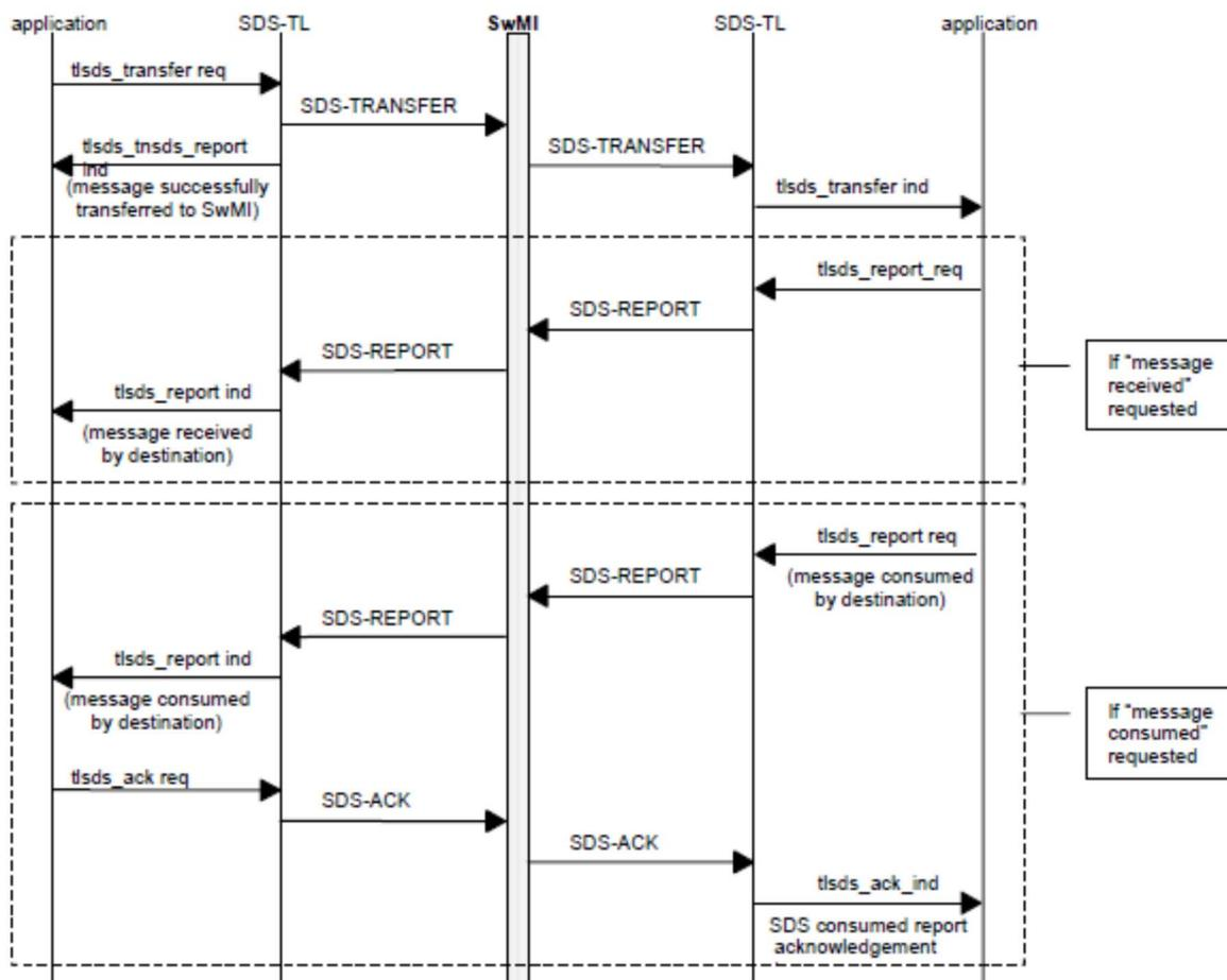
**Figure 72: SDS signalling flow chart for SDS type 4 via SDS-TL protocol according to ETSI EN 300 392-2 [27], clause 29.3.3 with transparent SwMI transport (SwMI store-and-forward functionality uses additional SDS-REPORT and SDS-ACK messages)**
