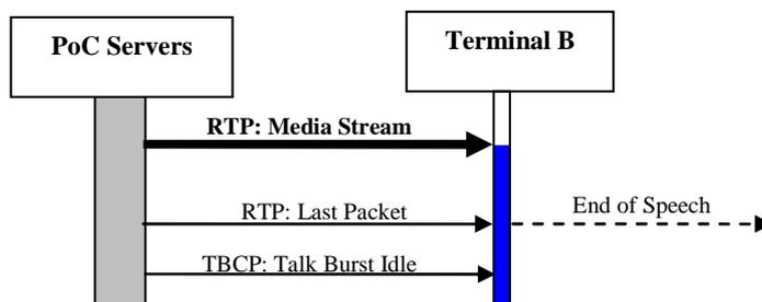
c) Last Media Stream from User B to User A via PoC Network (without Media Buffering), including Talk Burst Request of User B.
