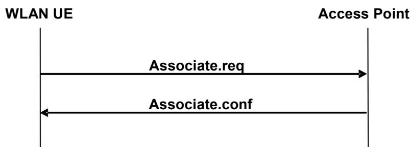
Figure 44: WLAN RE-ASSOCIATION Signal Flow
