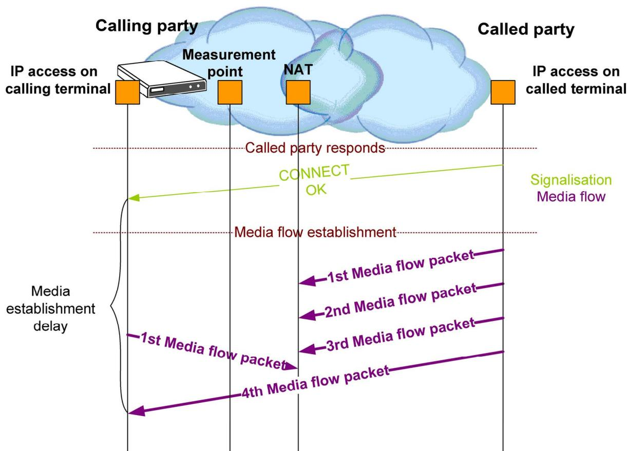
Figure 59: Media setup delayed due to NAT devices
