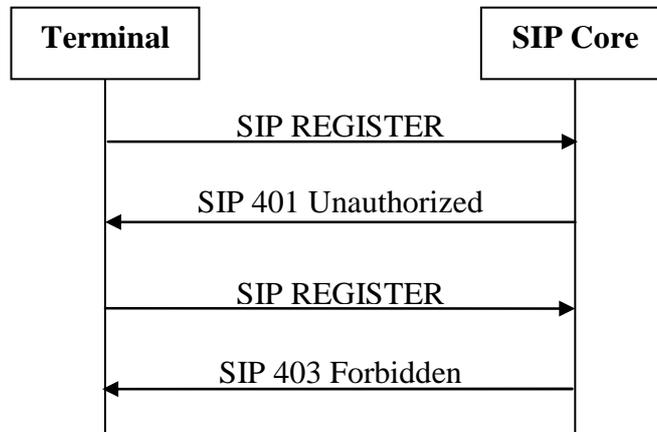
NOTE: This figure shows an example for an unsuccessful PoC registration. After the first "SIP REGISTER" request the terminal has to answer to a WWW- authentication challenge (see [16]). If the terminal does not answer correctly to this challenge, the SIP core will send a "SIP 403 Forbidden" message.
