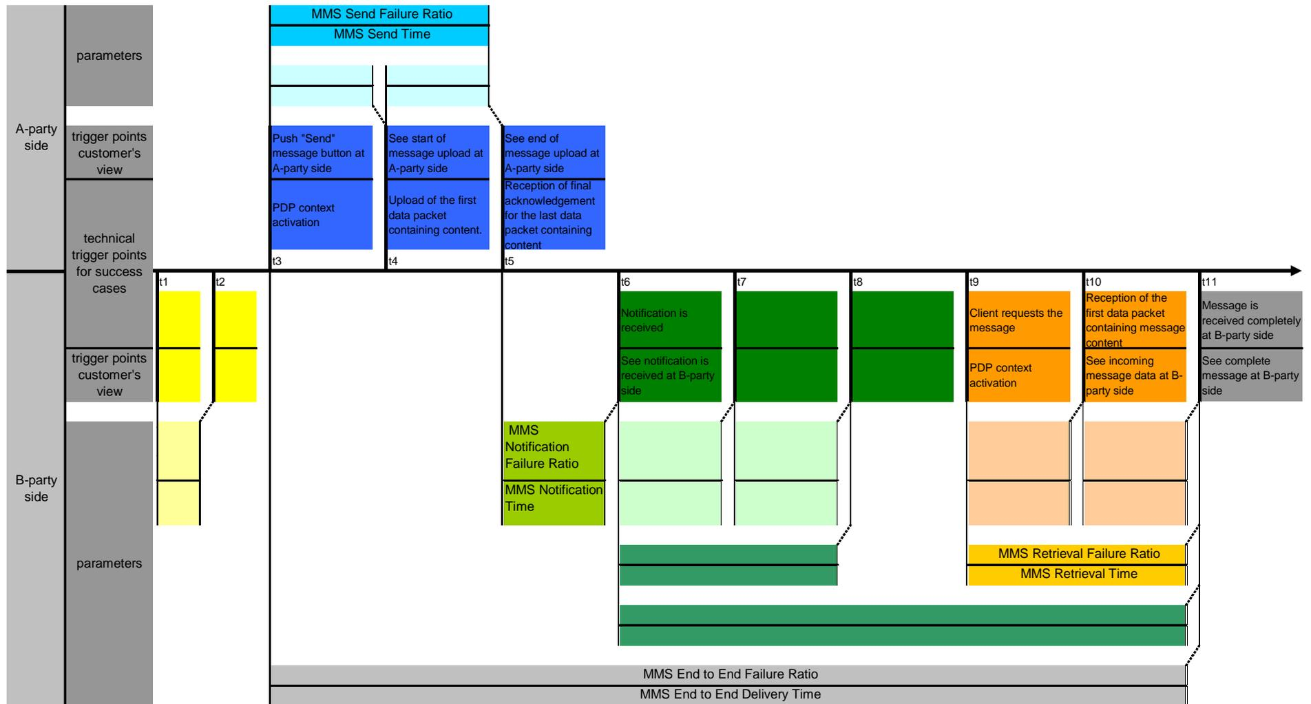
Figure 66: MMS Parameter Overview with Trigger Points
