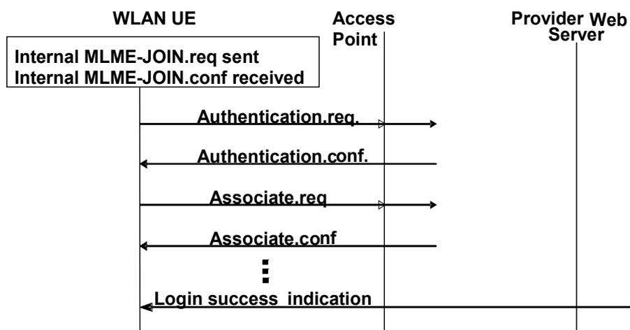
Figure 38: WLAN PS Data Service Provisioning Signal Flow
