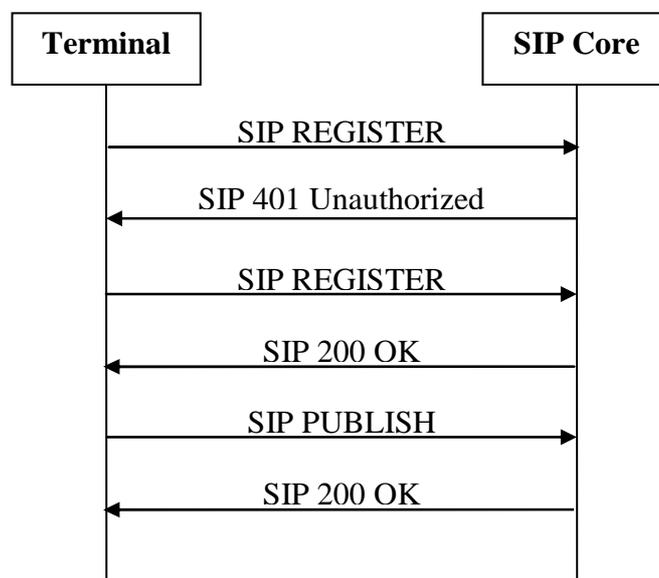
Figure 11: Example for a successful PoC Registration (long)
