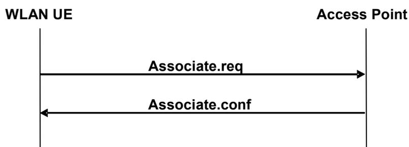
Figure 43: WLAN RE-ASSOCIATION Signal Flow
