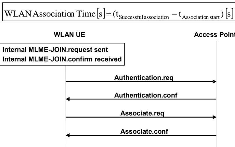
Figure 42: WLAN ASSOCIATION Signal Flow
