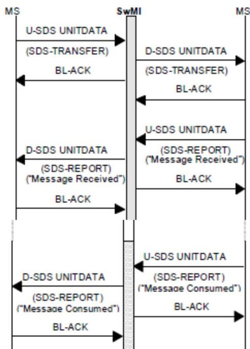
Figure 70: SDS signalling flow chart
