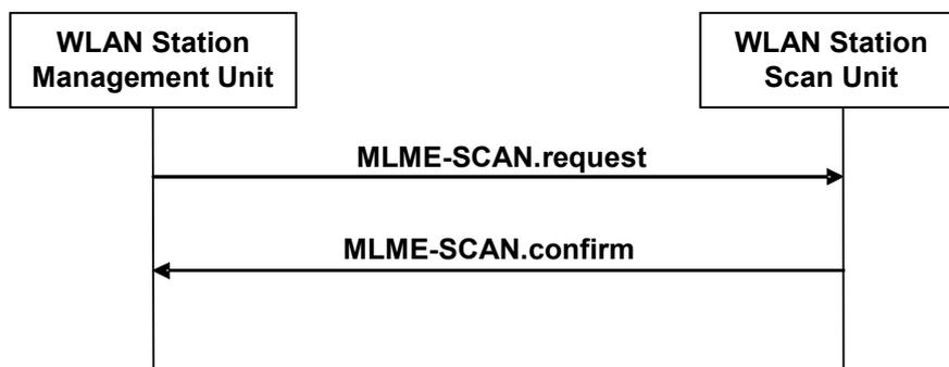
Figure 35: SCAN Signal Flow
