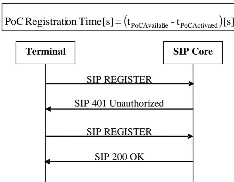
NOTE: This figure shows an example of a successful PoC registration (see [16]). In contrast to Figure 13, the terminal answered correctly to the authentication challenge (the second "SIP REGISTER" message).
