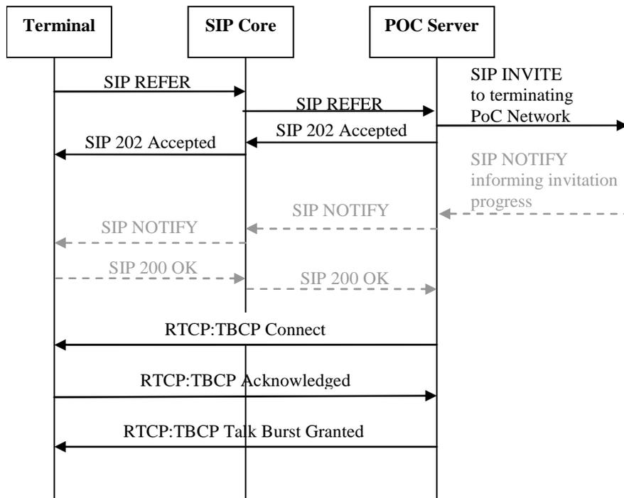
NOTE: The dashed arrows in this figure only occur in case of a confirmed, manual answer invitation. In this case the time period between the "SIP INVITE" message and the reception of the "Talk Burst Granted" message depends on how fast an invited user on the terminating side answers to the invitation. Furthermore, the "SIP NOTIFY" message is defined as optional (see [15]) and might not be sent by the server at all. For this reason the automatic answer mode shall be used during measurements.
