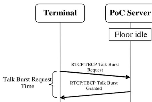
Figure 20: Example for a successful talk burst request
