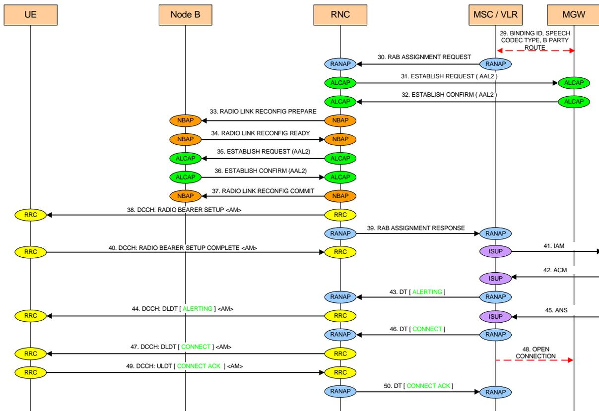
Figure 25: 3G telephony signalling flow chart: mobile originated call establishment procedure
