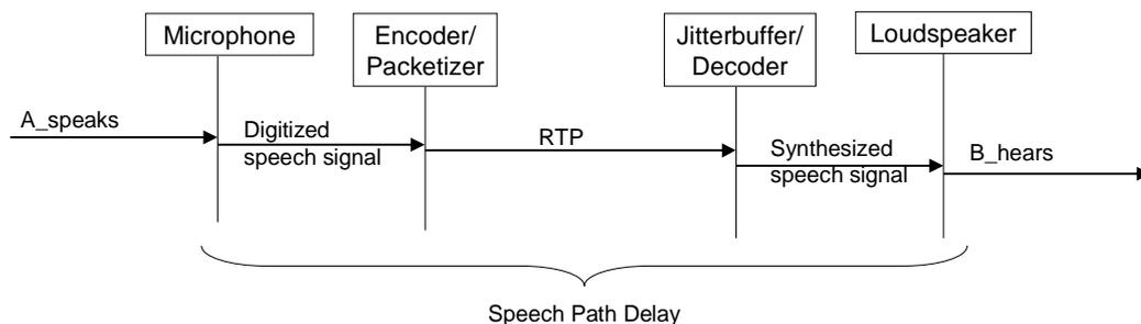
NOTE: Since the delay can vary during a call, it is not statistically sufficient to measure the delay only once.
