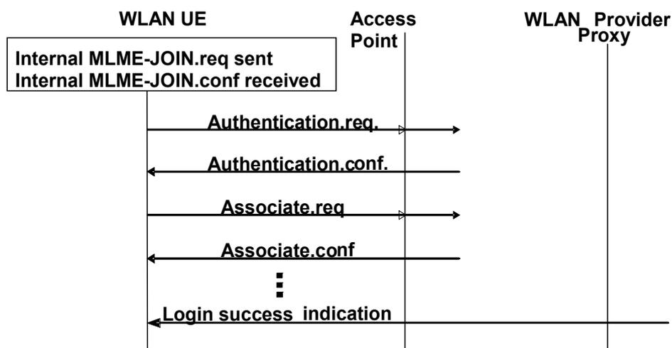
Figure 40: WLAN PS Data Service Provisioning Signal Flow
