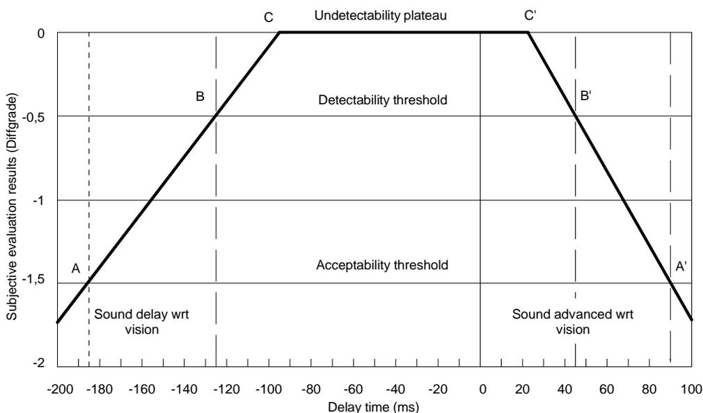
**Figure 56: The impact of audio video de-synchronization on perceived quality**
