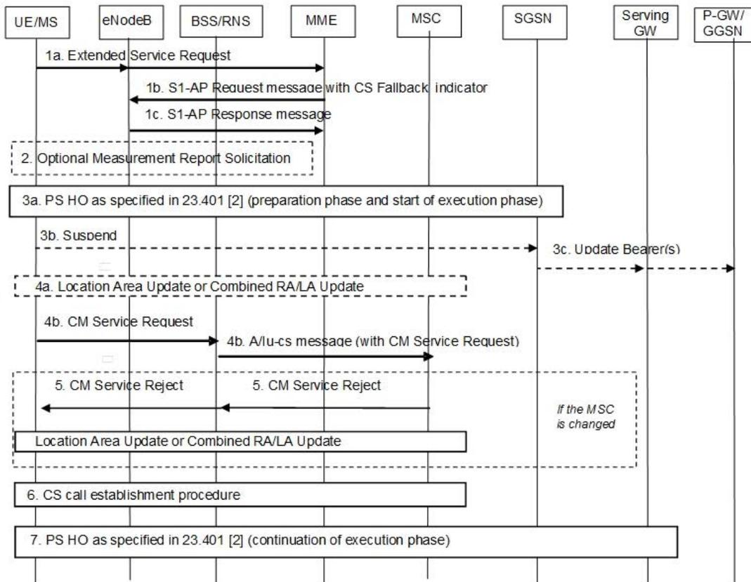
NOTE: This figure describes the mainly procedures of CSFB, the specific procedure such as CS call establishment please refer to the call establishment procedure in 2G/3G.
