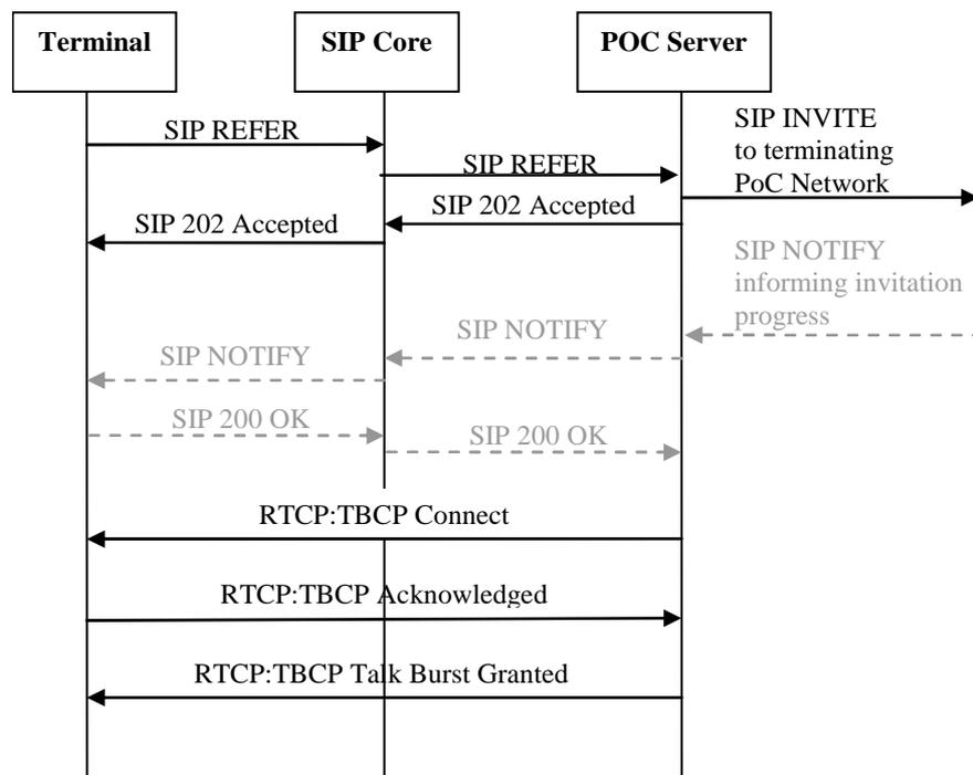
NOTE: The dashed arrows in figure 12 only occur in case of a confirmed, manual answer invitation. In this case the time period between the "SIP INVITE" message and the reception of the "Talk Burst Granted" message depends on how fast an invited user on the terminating side answers to the invitation. Furthermore, the "SIP NOTIFY" message is defined as optional (see [15]) and might not be sent by the server at all. For this reason the automatic answer mode shall be used during measurements.
