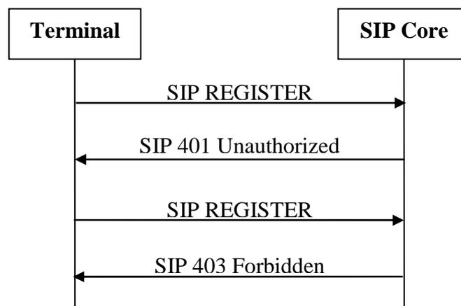
NOTE: Figure 6 shows an example for an unsuccessful PoC registration. After the first "SIP REGISTER" request the terminal has to answer to a WWW- authentication challenge (see [16]). If the terminal does not answer correctly to this challenge, the SIP core will send a "SIP 403 Forbidden" message.
