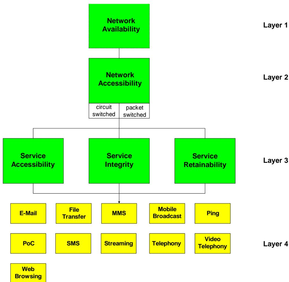
Figure 1: QoS aspects and the corresponding QoS parameters
