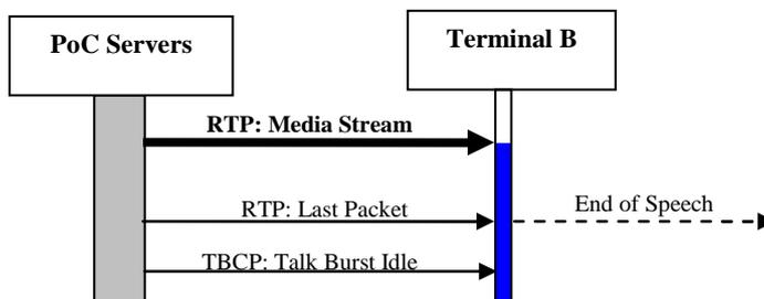
c) Last Media Stream from User B to User A via PoC Network (without Media Buffering), including Talk Burst Request of User B.
