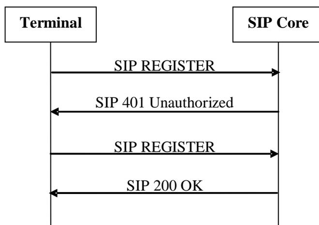
NOTE: Figure 7 shows an example of a successful PoC registration (see [16]). In contrast to figure 11, the terminal answered correctly to the authentication challenge (the second "SIP REGISTER" message).
