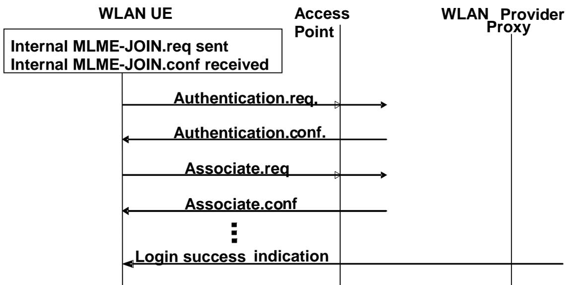
Figure 32: WLAN PS Data Service Provisioning Signal Flow
