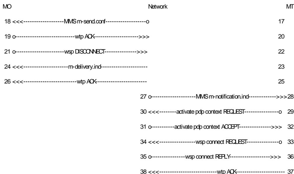
Figure 9: MMS Transaction flow
