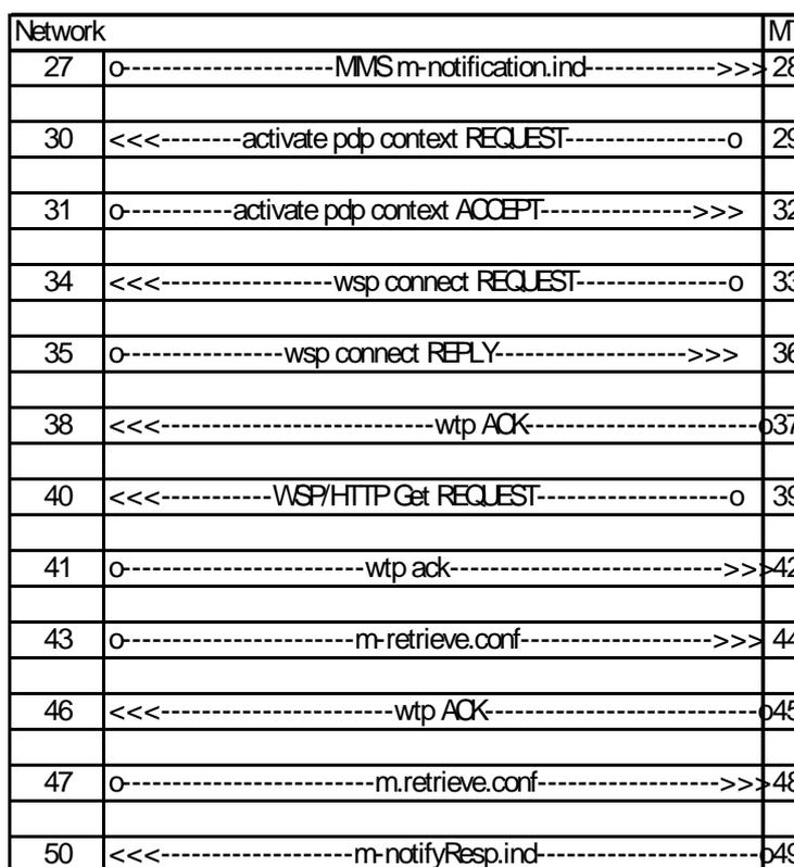
Figure 7: MMS Transaction flow
