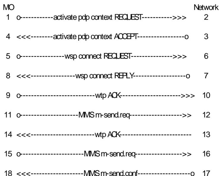
**Figure 4: MMS Transaction flow**
