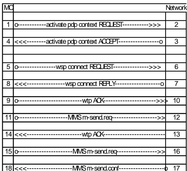
Figure 6: MMS Transaction flow
