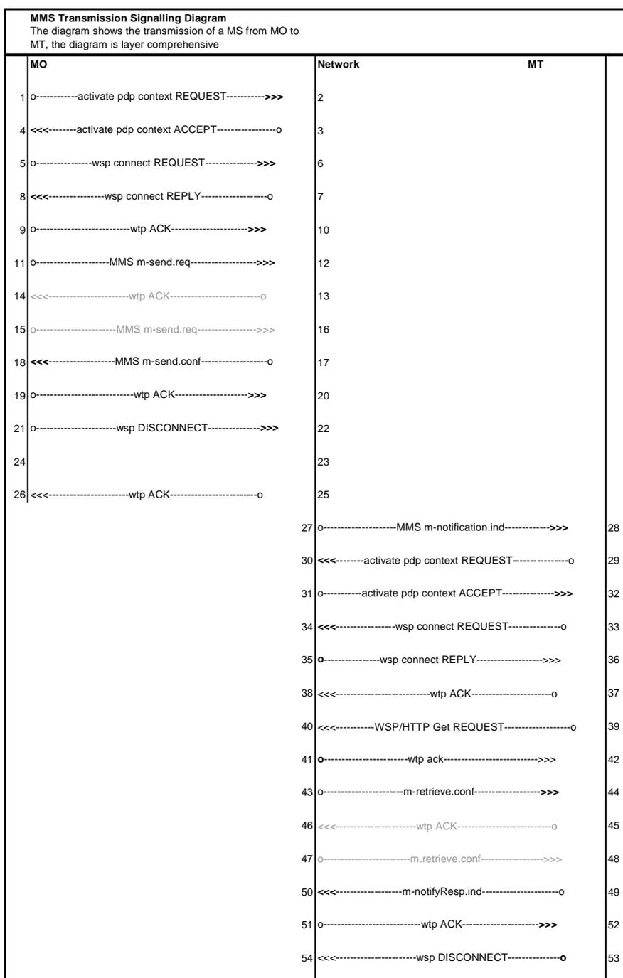
**Figure 10: MMS transaction flow**
