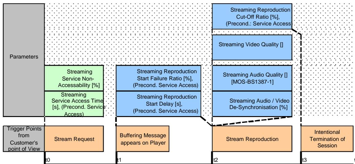
Figure 13: Parameter overview with trigger points
