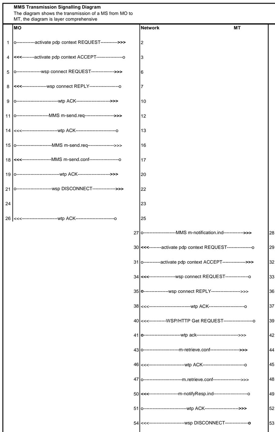
Figure 11: MMS Signalling Diagram
