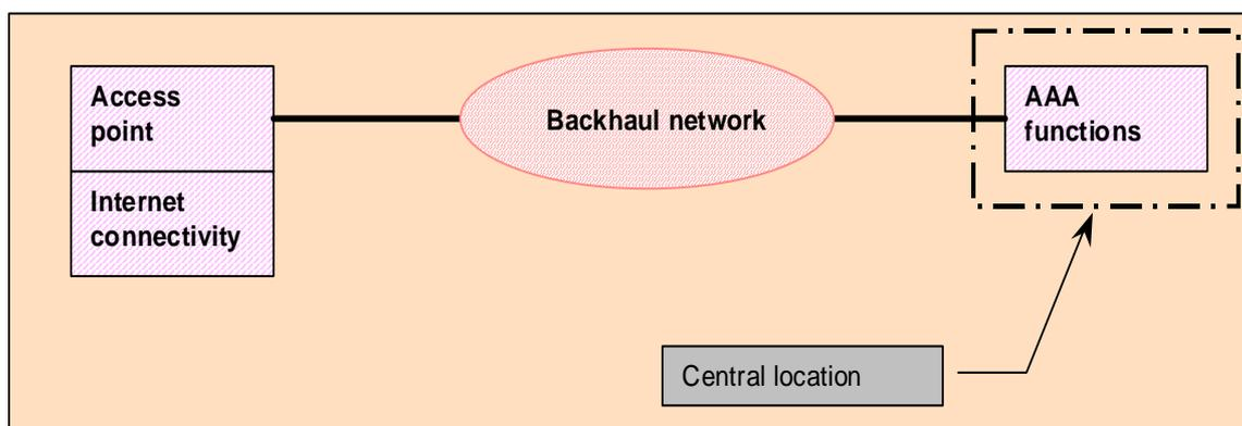
Figure 5: Reference scenario for Wireless LAN access
