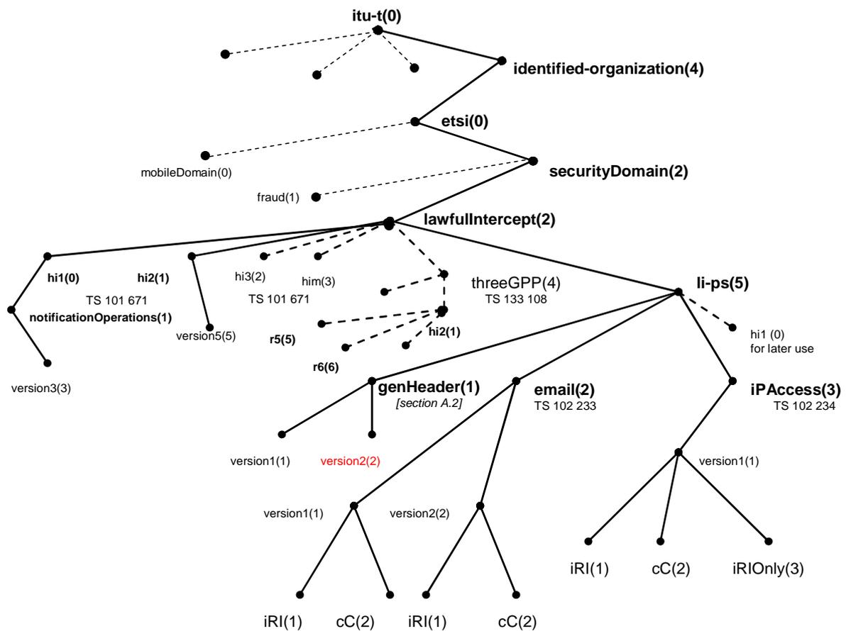
Figure A.1: Object identifier tree
