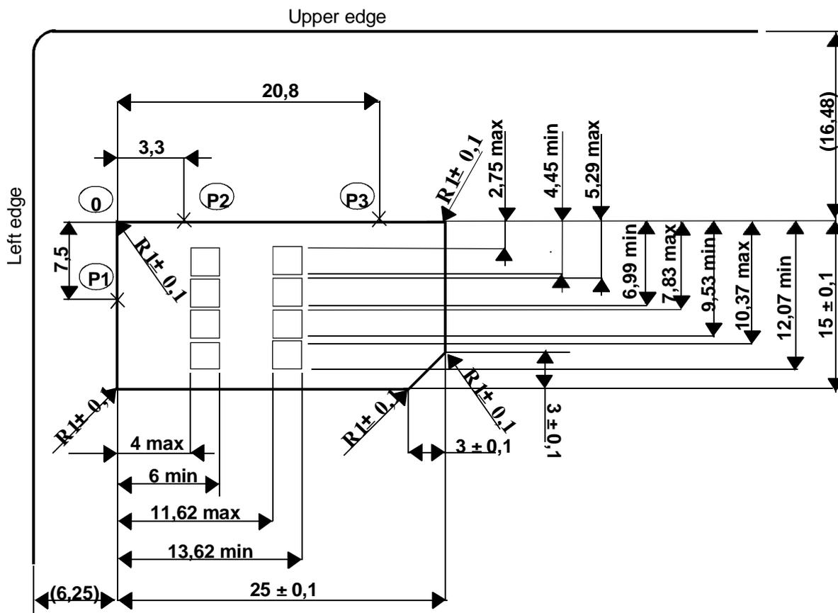
Figure 4.1: Plug-in UICC
