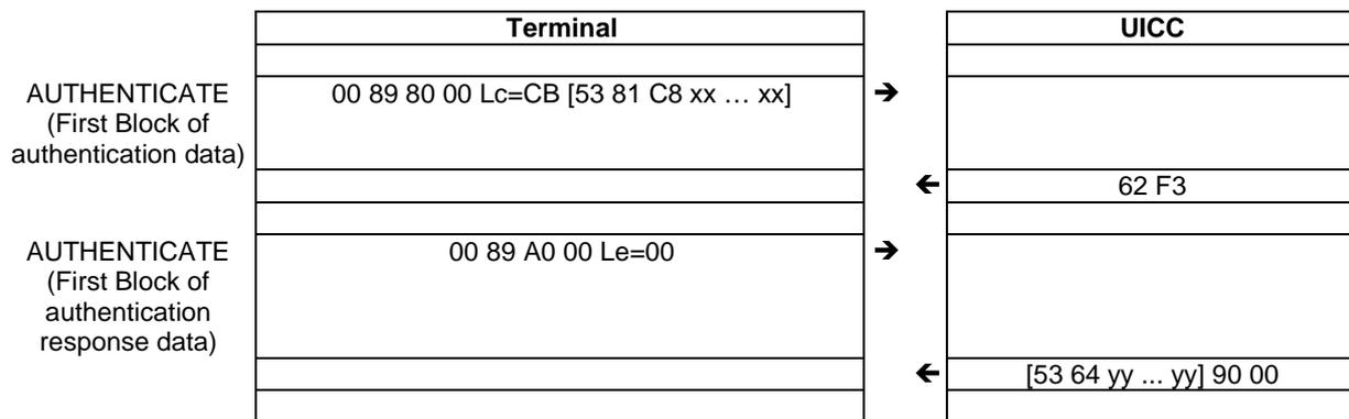
In the second example the length of the challenge data is 700 bytes ('02BC' hex) and the length of the response data is 600 bytes ('0258' hex).
