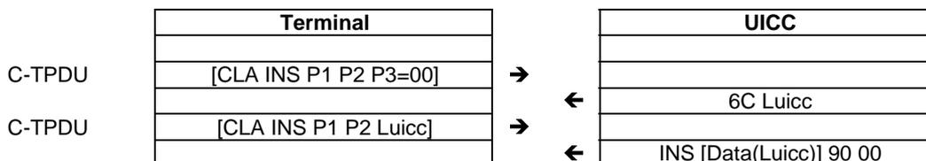
An R-APDU of {[Data(Luicc)] 90 00} is returned from the UICC to the terminal.
