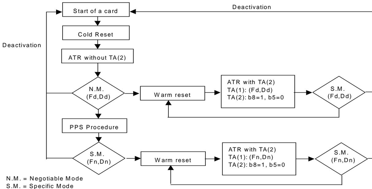
**Figure I.2: Modes of operation of a "Type 2 UICC"**
