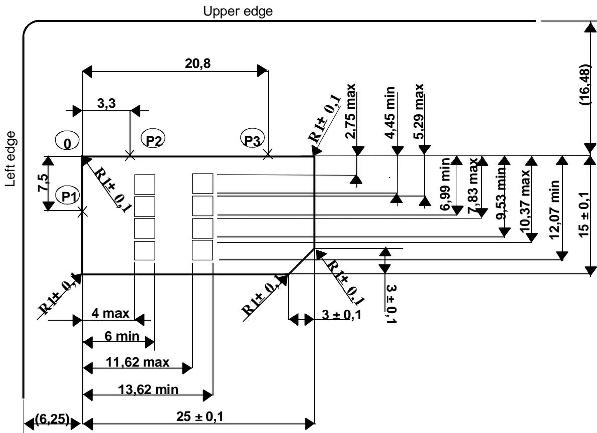
Figure 4.1: Plug-in UICC
