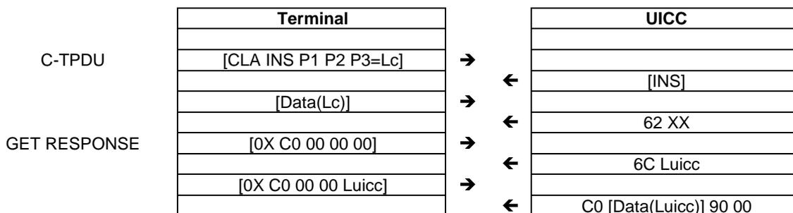
An R-APDU of {[Data(Luicc)] 62 XX} is returned from the UICC to the terminal containing the data returned together with the warning status bytes.
