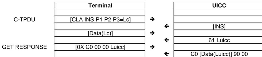
An R-APDU of {[Data(Luicc)] 90 00} is returned from the UICC to the terminal.
