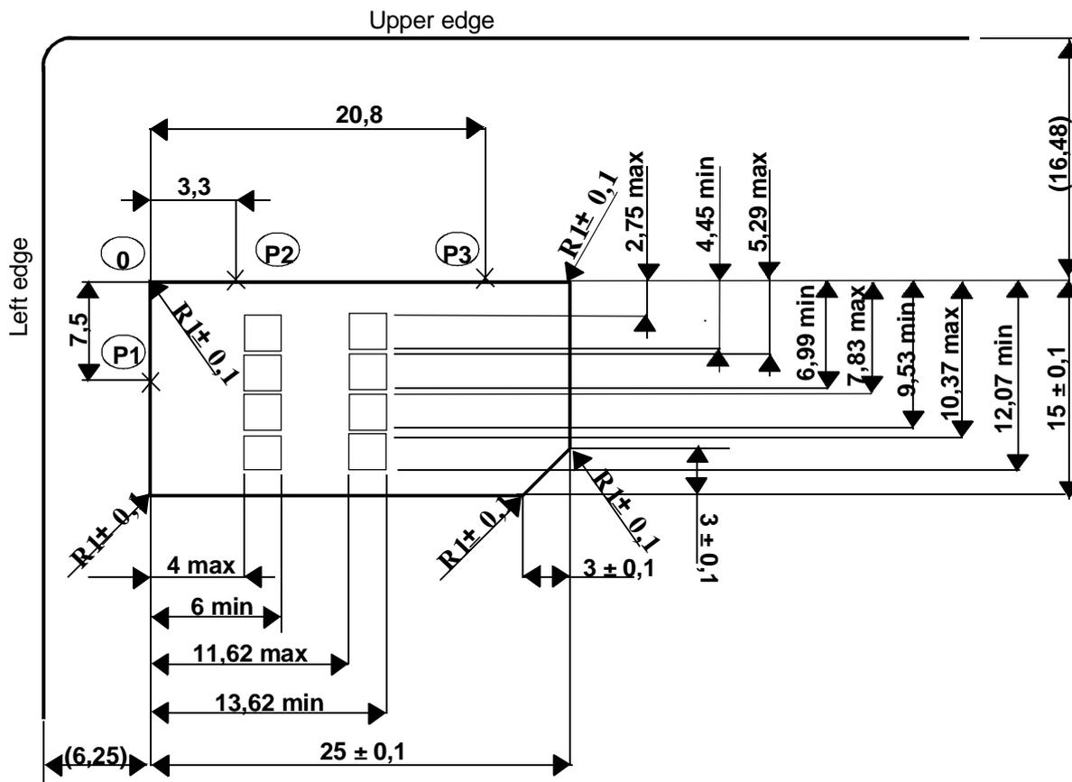
Figure 4.1: Plug-in UICC
