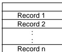
**Figure 8.2: Structure of a linear fixed file**
