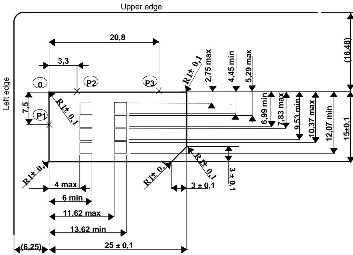
Figure 4.1: Plug-in UICC
