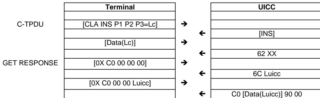
An R-APDU of {[Data(Luicc)] 62 XX} is returned from the terminal to the UICC containing the data returned together with the warning status bytes.
