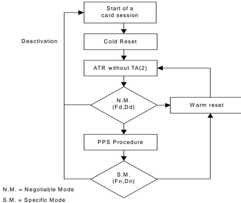
**Figure I.1: Modes of operation of a "Type 1 UICC"**
