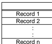
**Figure 8.2: Structure of a linear fixed file**
