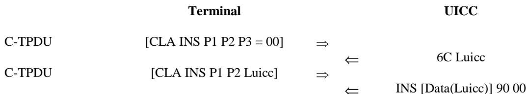
An R-APDU of {[Data(Luicc)] 90 00} is returned from the UICC to the terminal.
