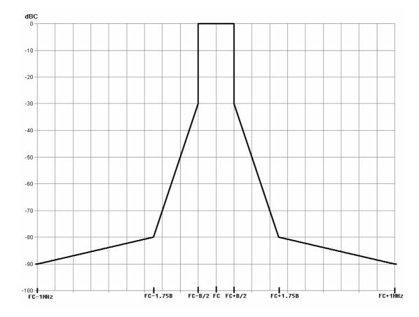
The transmitter output spectrum shall be within the mask defined in figure 8.2
