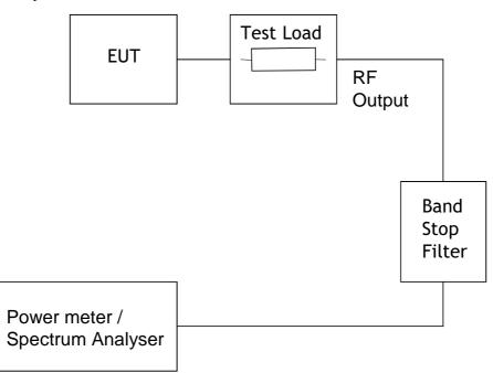
Figure 8.1: Method for measuring the relative suppression of a digital system
