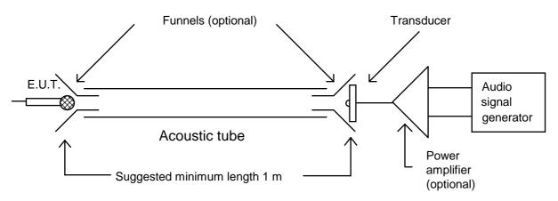
Figure 12.3: Example of acoustic coupling jig
