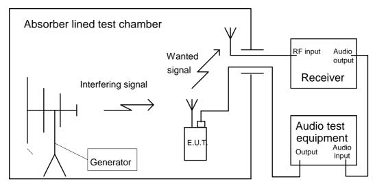
Figure 12.1: Test configuration for integral antenna; transmitter operation - electrical input
