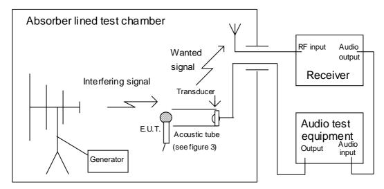
Figure 12.2: Test configuration for integral antenna; transmitter operation - acoustic input
