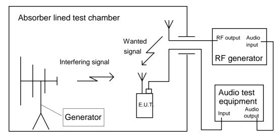
NOTE: The RF generator may be a companion transmitter sited inside the test chamber if necessary.
