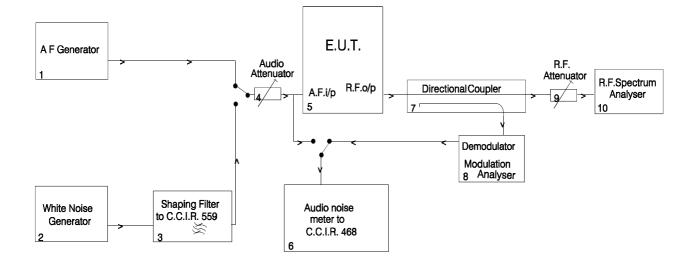
NOTE: If the EUT incorporates ancillary coding or signalling channels, for example, pilot tone, etc. these should be switched on prior to measuring the transmitter RF output spectrum.
