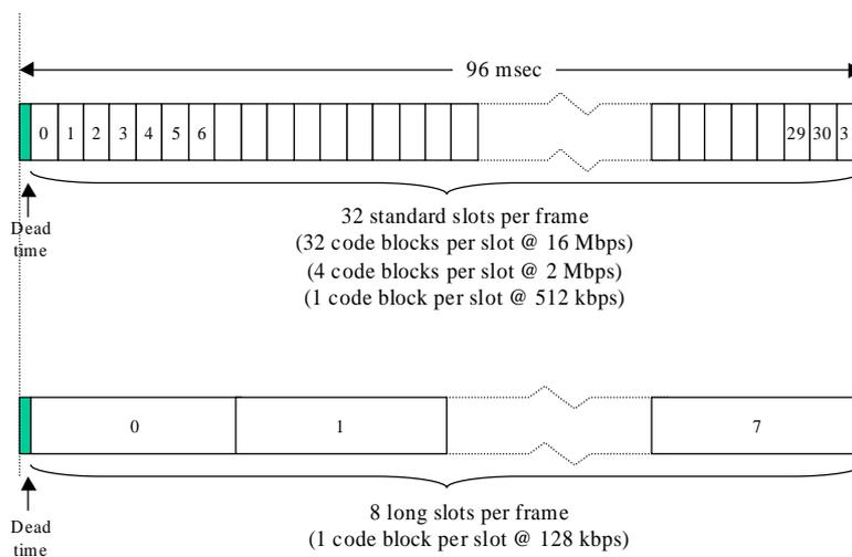
**Figure 5.3.2.4: Uplink frame structure**
