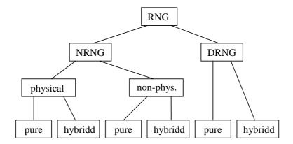
Figure E.1: Schematic classification of random number generators according to ISO/IEC FCD 18031 [i.14]
