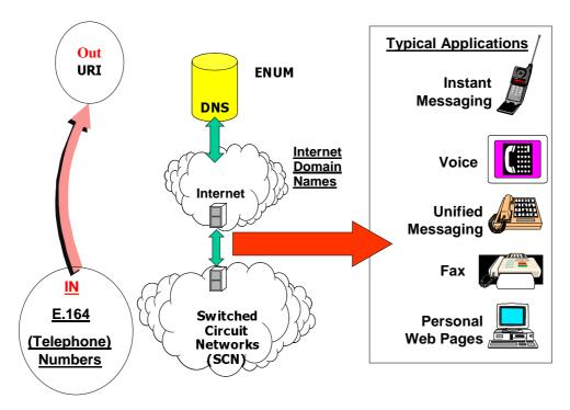
Figure 1: Typical applications enabled through ENUM
