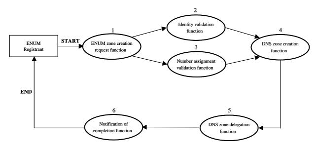
Figure 6: Functional model for Registration
