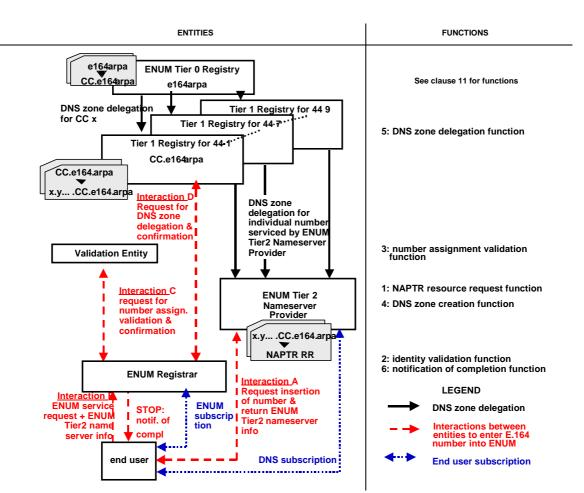
Figure A.2: Multiple Tier 1 Registries and separate ENUM Tier 2 Nameserver Provider and Registrar - Entering an E.164 number and NAPTR records in ENUM database
