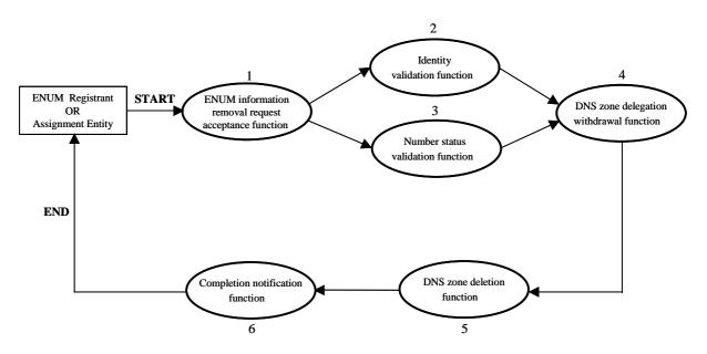
Figure 8: Functional model for removal of E.164 numbers from ENUM databases
