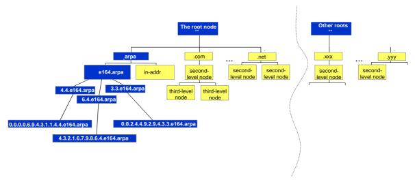
Figure 4: shows how ENUM fits into the DNS structure
