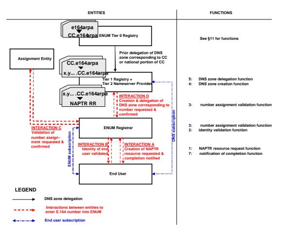
Figure A.3: Combined ENUM Tier 1 and 2 and separate ENUM Registrar - Entering an E.164 number and NAPTR records in ENUM database
