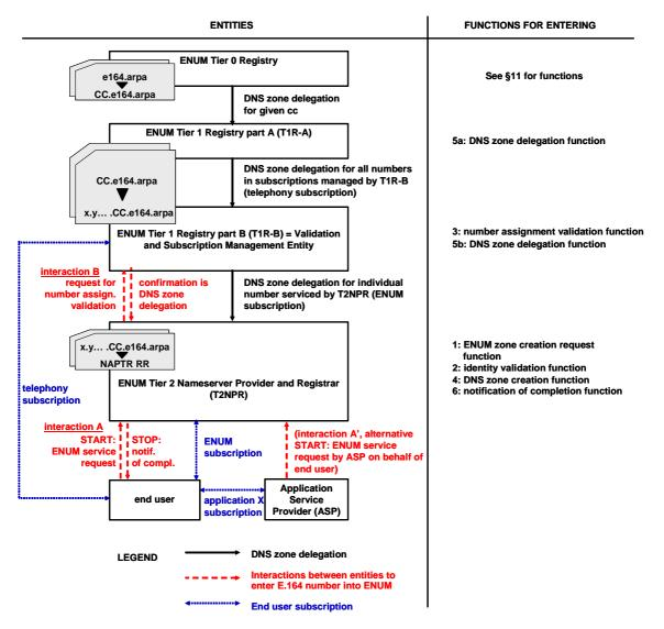
Figure A.4: Two-stage Tier 1 with combined ENUM Tier 2 Nameserver Provider and Registrar - Entering an E.164 number and NAPTR records in ENUM database
