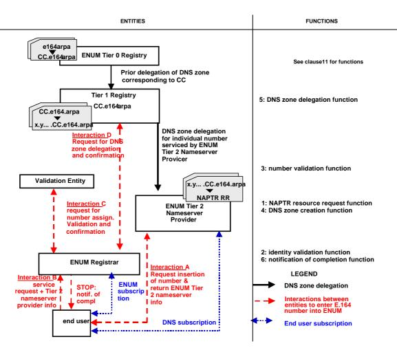
Figure A.1: Single Tier 1 Registry and separate ENUM Tier 2 Nameserver provider and Registrar - Entering an E.164 number and NAPTR records in ENUM database
