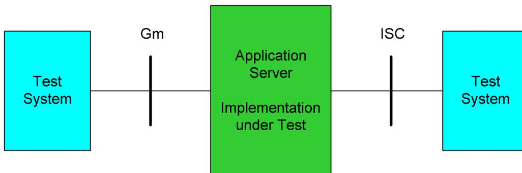
**Figure 4-1: Applicable interface to test AS functionalities**
