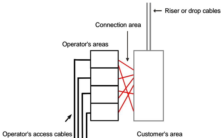
**Figure 3: Illustration of a Distribution Point**
