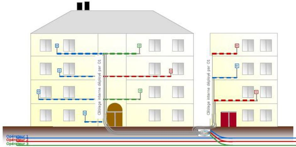
**Figure 2: Shared optical building cabling for all operators
