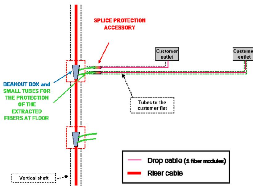
**Figure 5: Example of a Distribution System**
