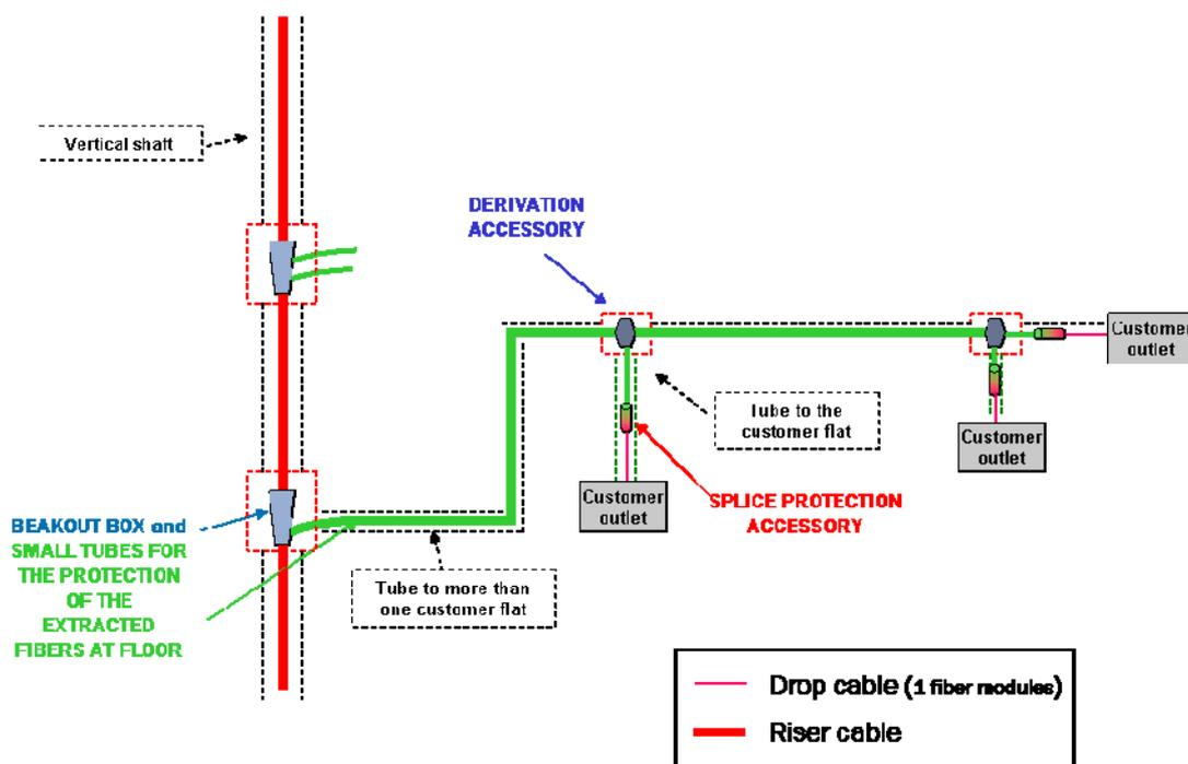
Figure 6: Example of a floor distributor System + derivation accessory in the case of initial sharing of customer tube
