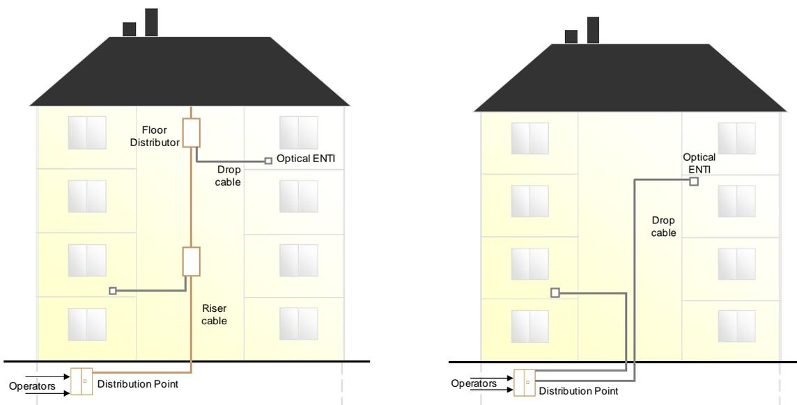
**Figure 4: Example of cabling solutions in buildings: The indoor cables may contain one or more fibres for each customer depending on the chosen architecture**
