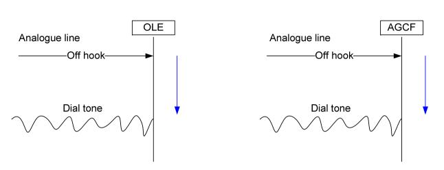
Figure 3: Local exchange analogue subscriber call request delay: overlap sending
