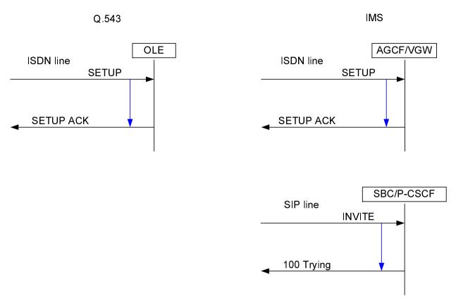
Figure 4: Local exchange ISDN subscriber call request delay: overlap sending
