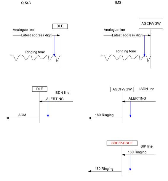
Figure 6: Local exchange Alerting sending delay for terminating traffic (in different locations)
