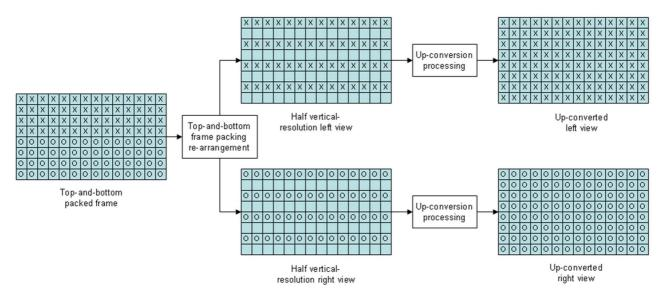
Figure A.2: Top-and-Bottom decoded video frame decomposition
