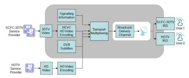
Figure 1: Scope of the service frame compatible plano-stereoscopic 3DTV specification
