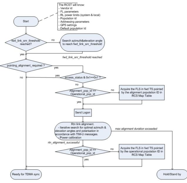
Figure 10.1: RCST antenna alignment and logon
