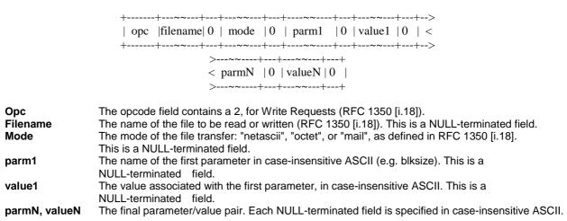
Figure C.5: SDDP parameters in WRQ packet
