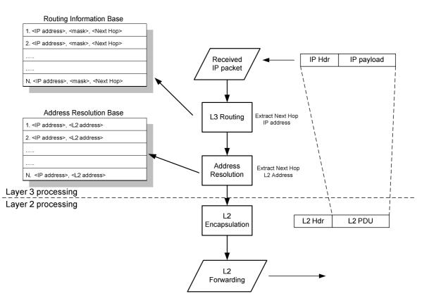
Figure 7.1: RCST Unicast IP packet forwarding
