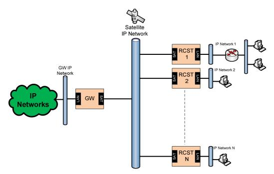
Figure 7.2: Example routing topology for a GW connecting N RCSTs
