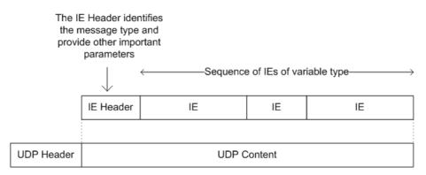
Figure D.3: DCP messages structure over UDP
