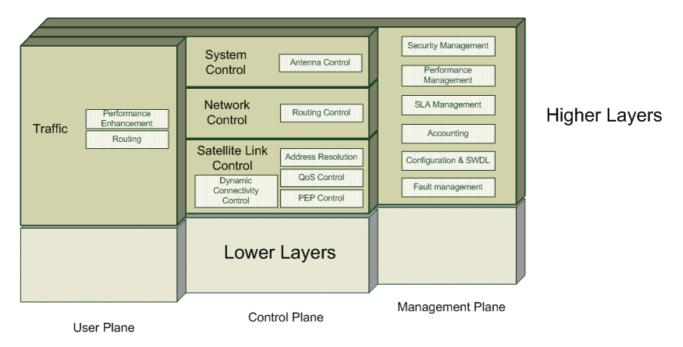
Figure 4.2: Higher layers functional modules
