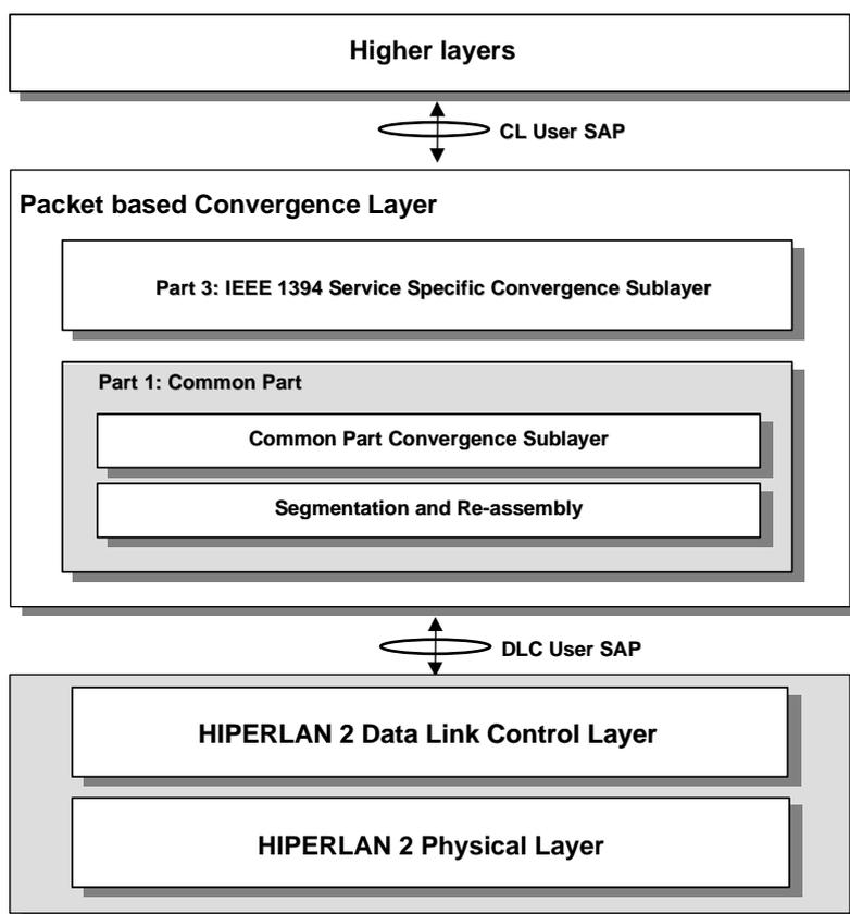
**Figure 1: IEEE 1394 [6] packet based convergence layer**
