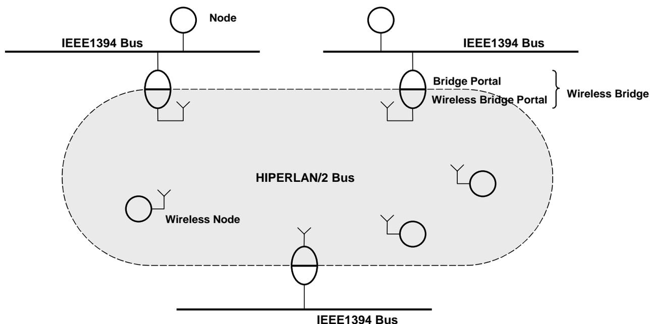
Figure 3: HL2 Bus connecting bridge and non-bridge 1394 devices
