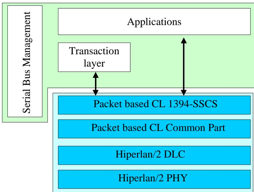
Figure 2: Protocol stack of a non-bridge wireless 1394 device
