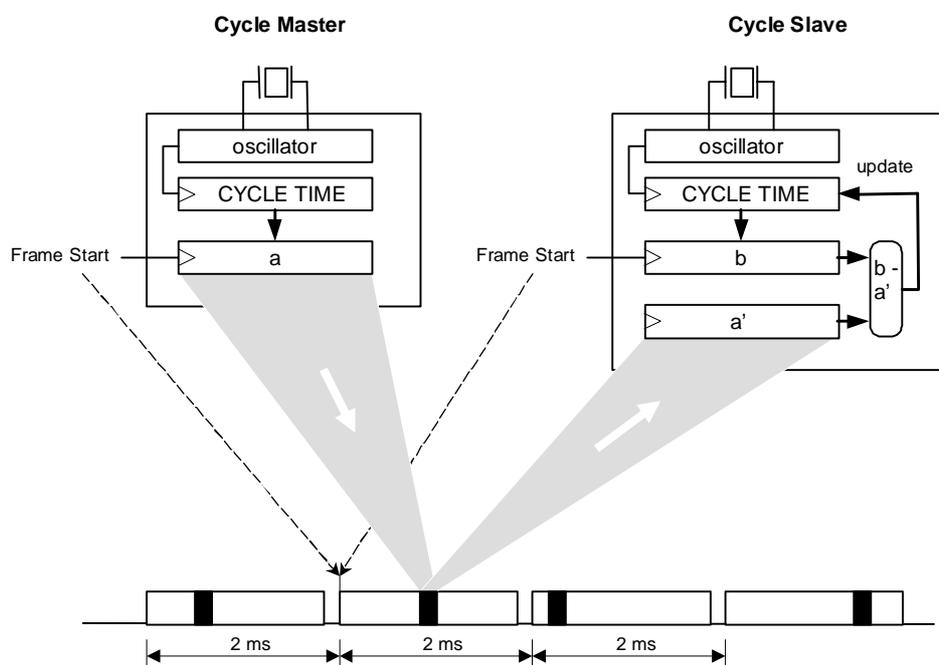
Figure 6: Synchronization principle of the CYCLE\_TIME register
