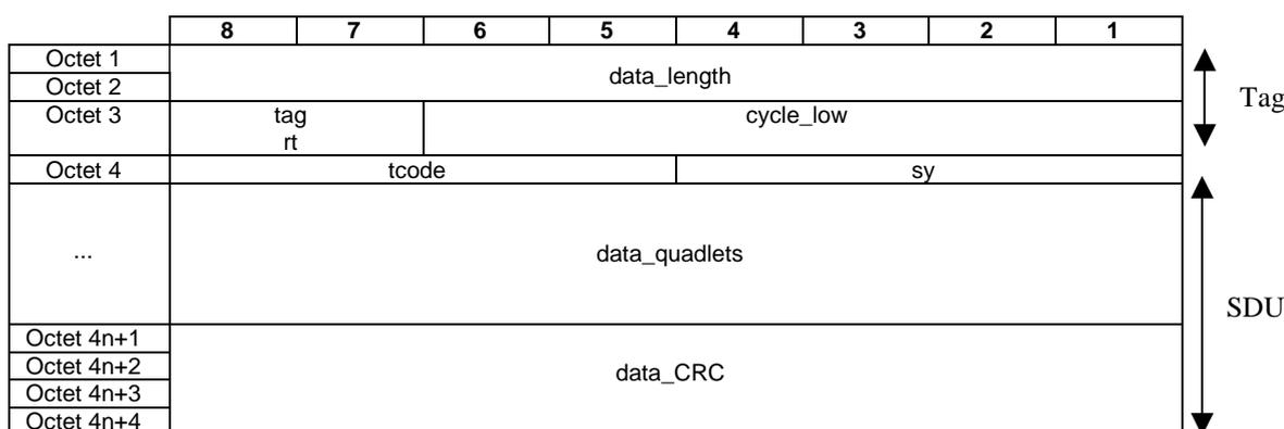
**Figure 10: Isochronous tagged SDU format**
