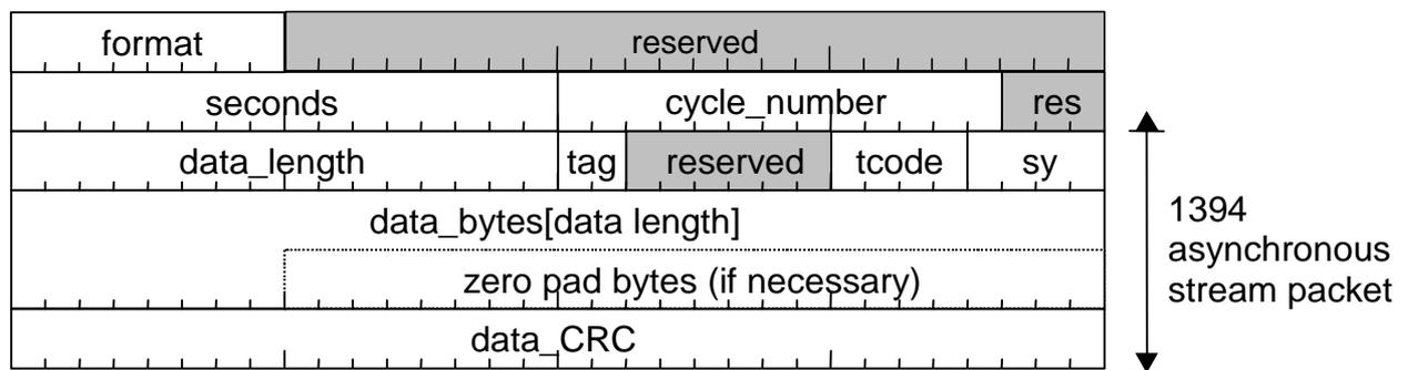
Figure B.4: Asynchronous stream PDU format
