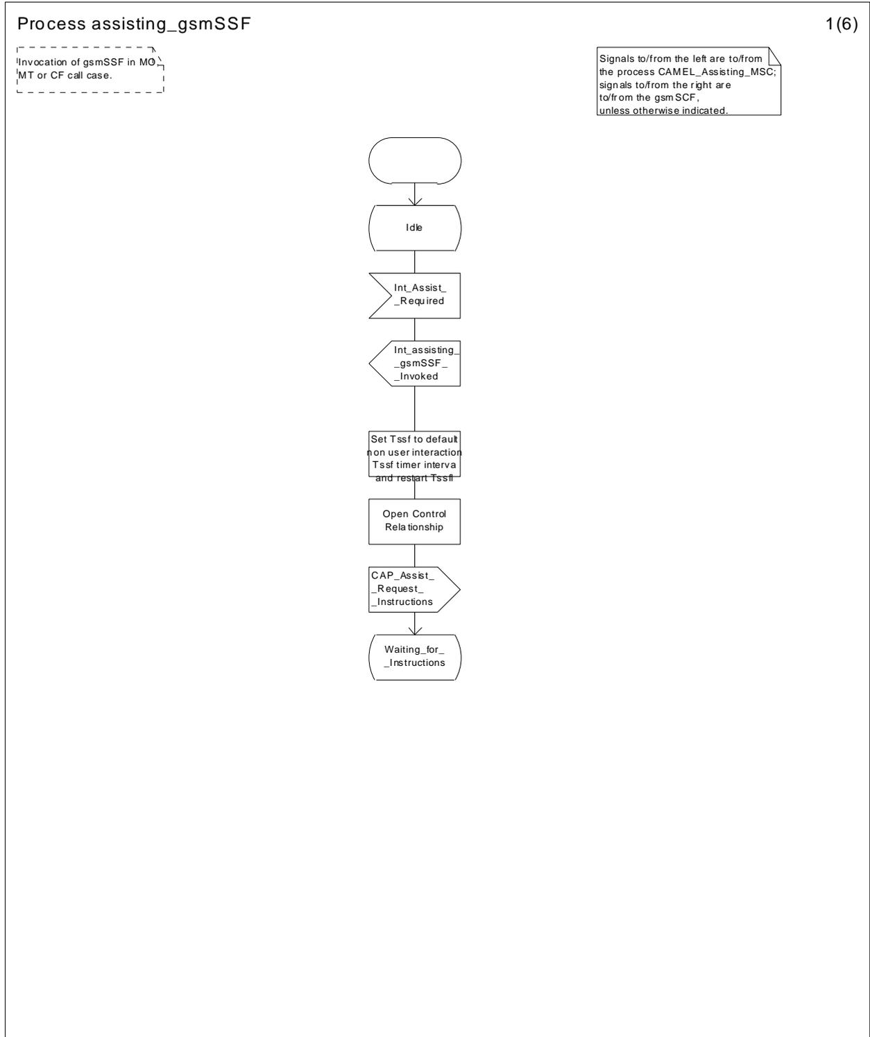
Figure 54a: Process Assisting\_gsmSSF (sheet 1)
