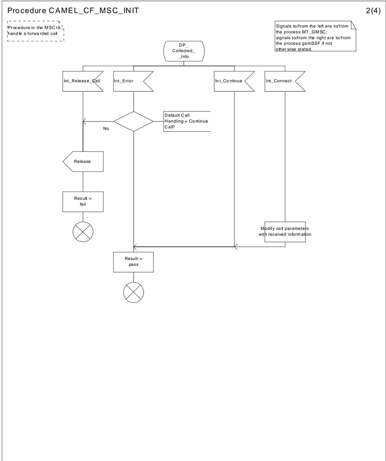
Figure 39b: Procedure CAMEL\_CF\_MSC\_INIT (sheet 2)
