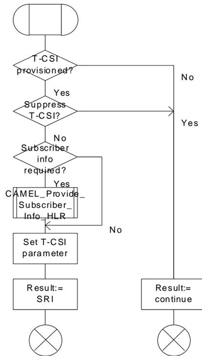
Figure 37a: Procedure CAMEL\_T\_CSI\_CHECK\_HLR (sheet 1)
