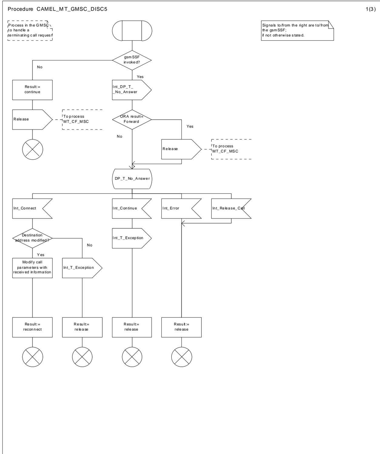
Figure 29a: Procedure CAMEL\_MT\_GMSC\_DISC5 (sheet 1)
