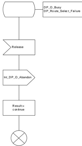
Figure 12b: Procedure CAMEL\_OCH\_MSC1 (sheet 2)
