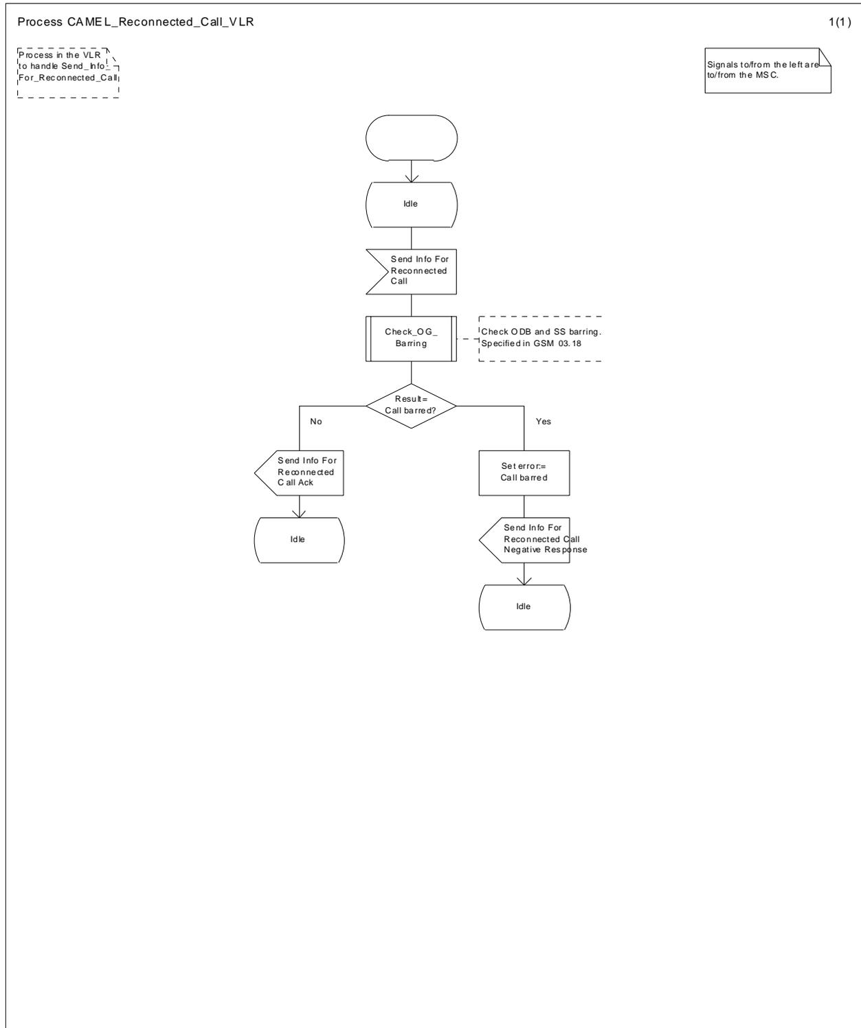
Figure 22a: Process CAMEL\_Reconnected\_Call\_VLR (sheet 1)
