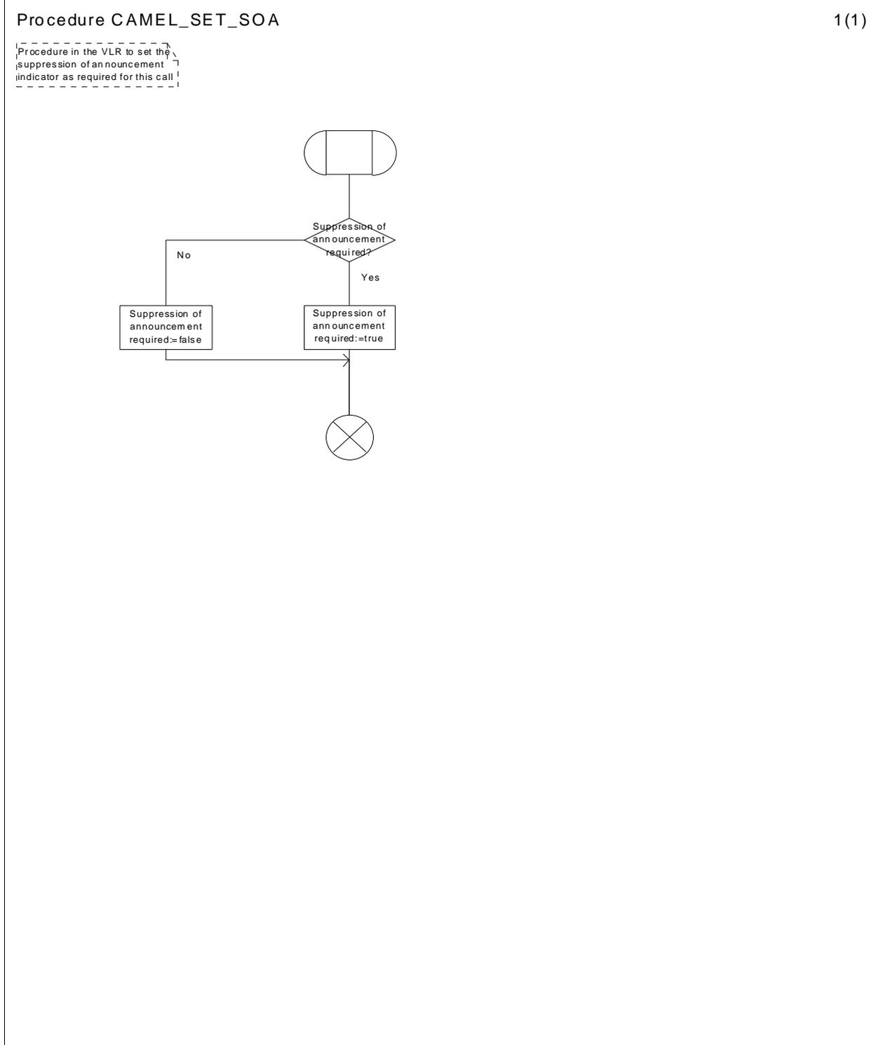
Figure 38a: Procedure CAMEL\_SET\_SOA (sheet 1)
