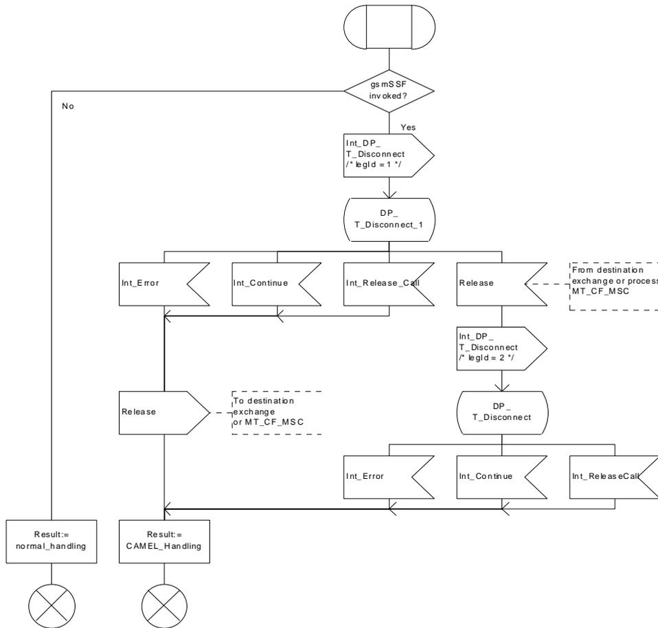
Figure 26a: Procedure CAMEL\_MT\_GMSC\_DISC1 (sheet 1)
