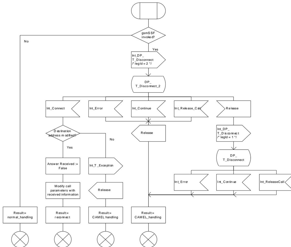
Figure 27a: Procedure CAMEL\_MT\_GMSC\_DISC2 (sheet 1)
