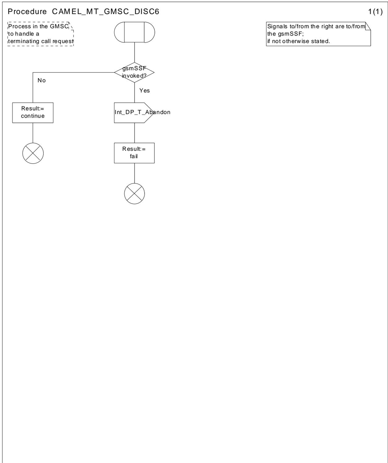
Figure 30a: Procedure CAMEL\_MT\_GMSC\_DISC6 (sheet 1)
