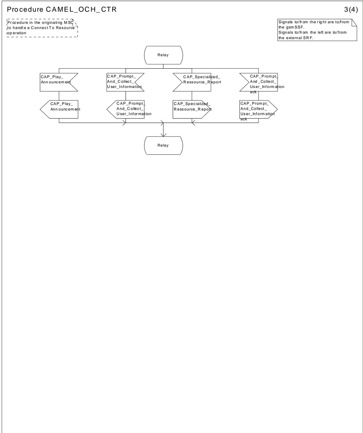
Figure 18c: Procedure CAMEL\_OCH\_CTR (sheet 3)
