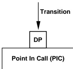
Figure 2: BCSM Components
