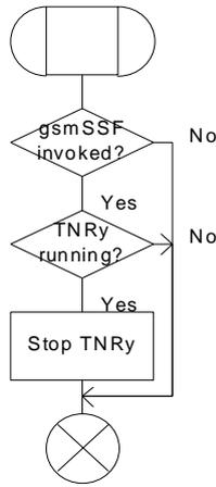
Figure 20a: Procedure CAMEL\_Stop\_TNRy (sheet 1)
