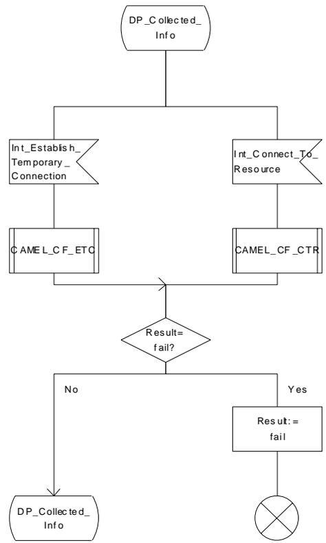
Figure 39c: Procedure CAMEL\_CF\_MSC\_INIT (sheet 3)
