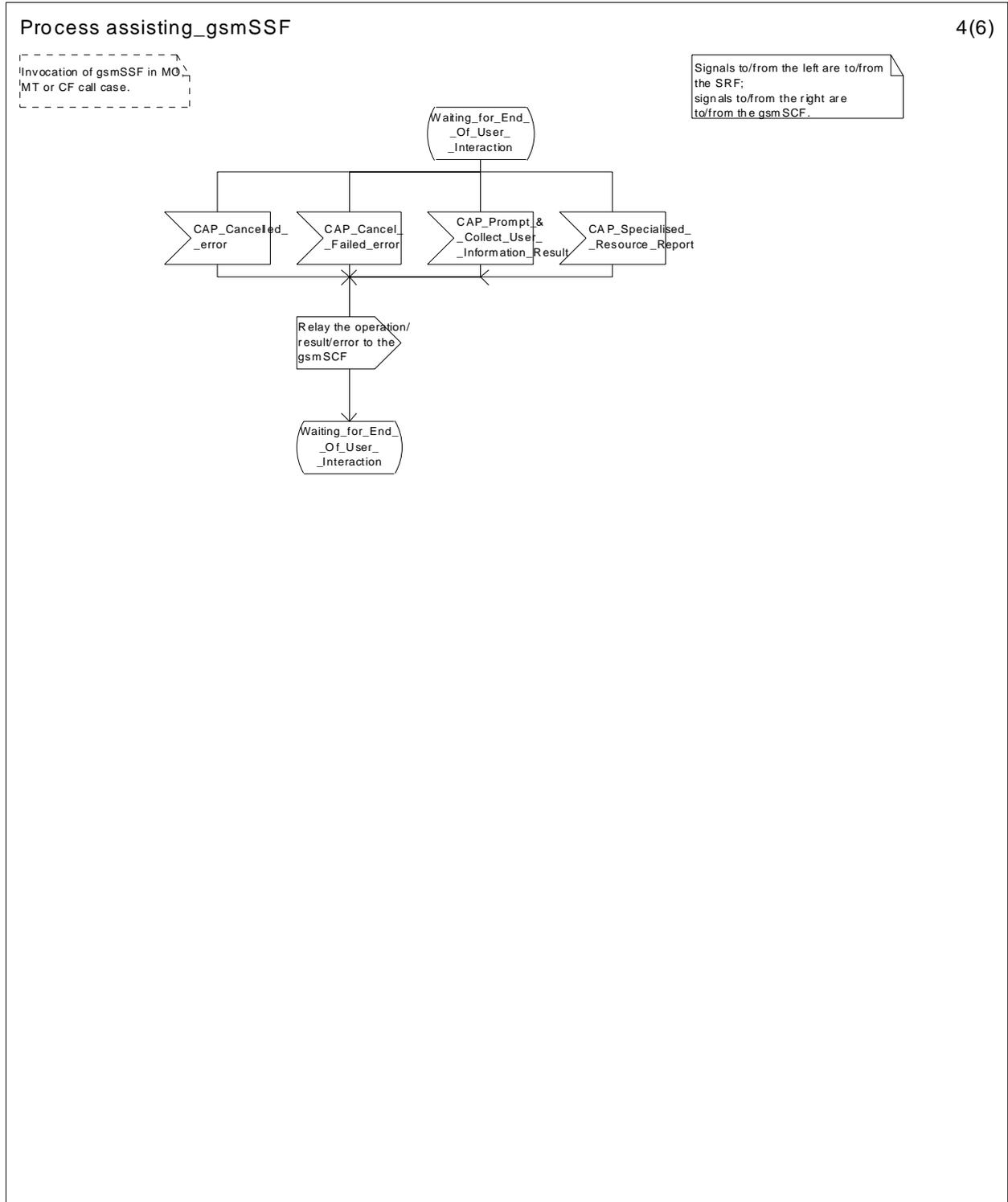
Figure 54d: Process Assisting\_gsmSSF (sheet 4)
