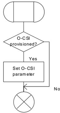
Figure 36a: Procedure CAMEL\_O\_CSI\_CHECK\_HLR (sheet 1)
