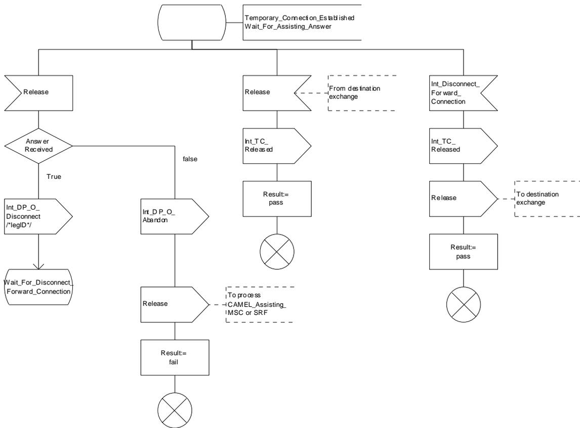
Figure 41c: Procedure CAMEL\_CF\_ETC (sheet 3)
