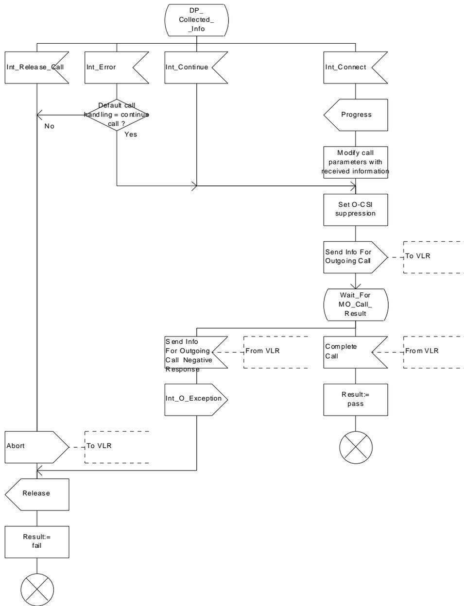
Figure 10b: Procedure CAMEL\_OCH\_MSC\_INIT (sheet 2)
