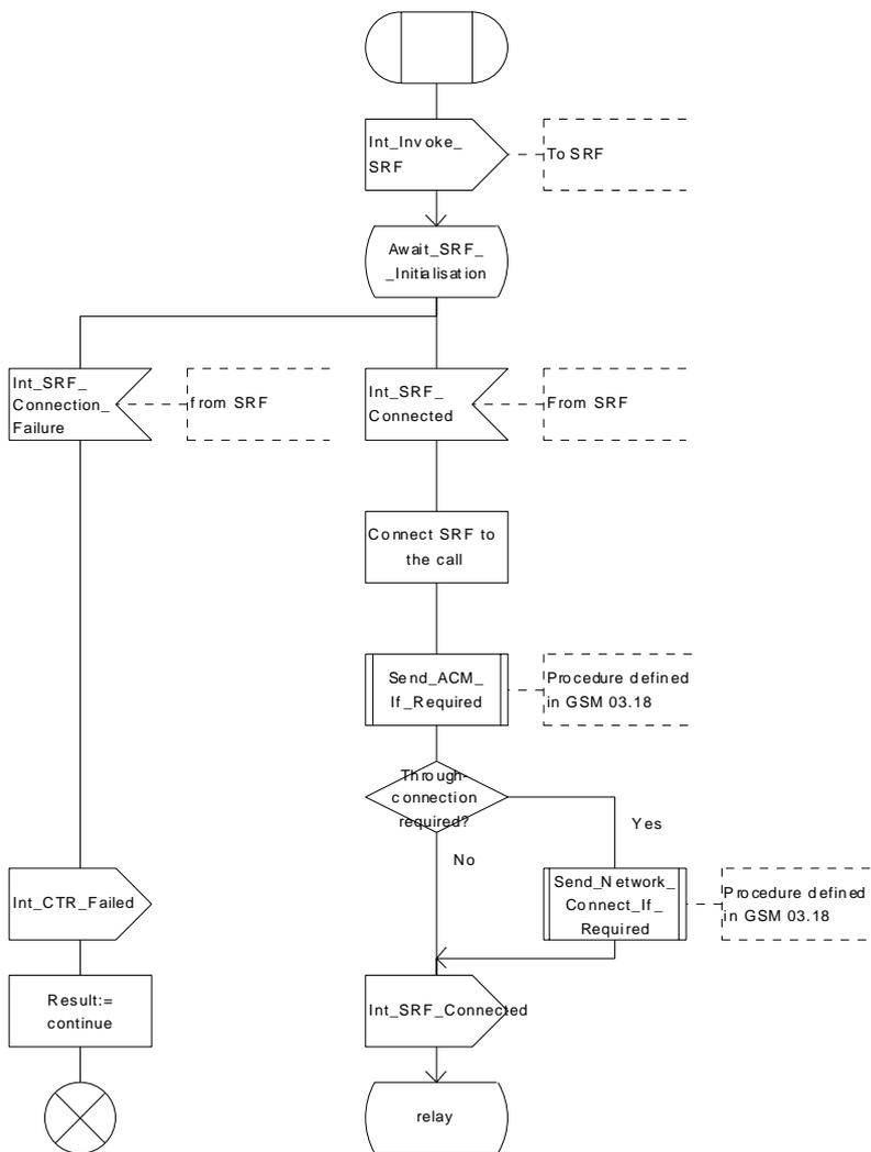
Figure 32a: Procedure CAMEL\_MT\_CTR (sheet 1)
