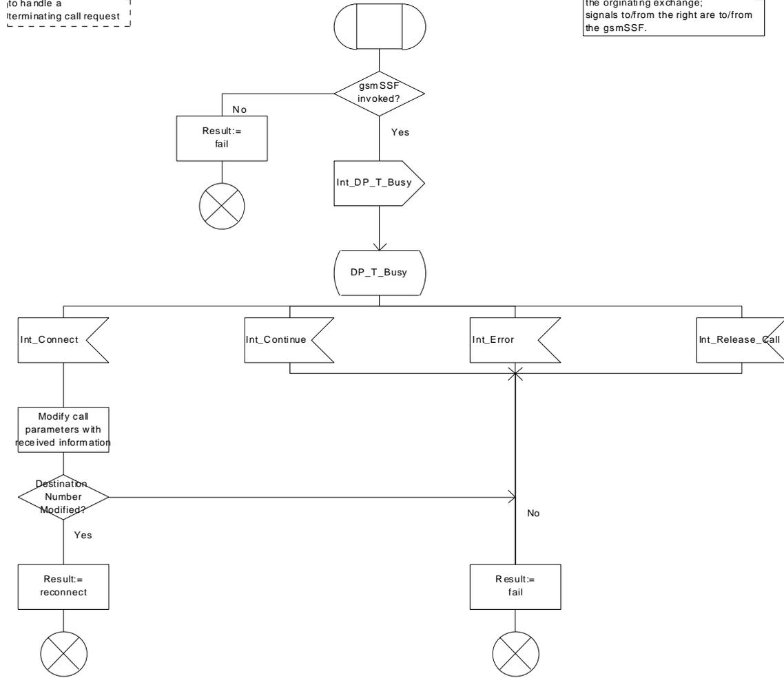
Figure 28a: Procedure CAMEL\_MT\_GMSC\_DISC4 (sheet 1)
