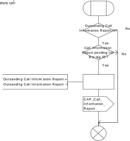
Figure 50a: Procedure Handle\_CIR\_leg (sheet 1)
