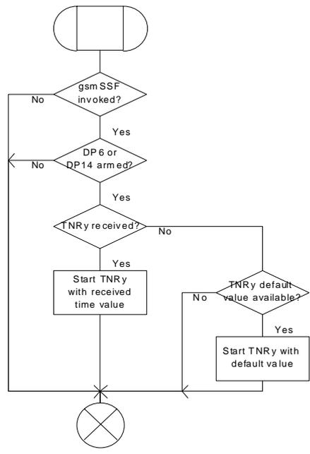
Figure 19a: Procedure CAMEL\_Start\_TNRy (sheet 1)
