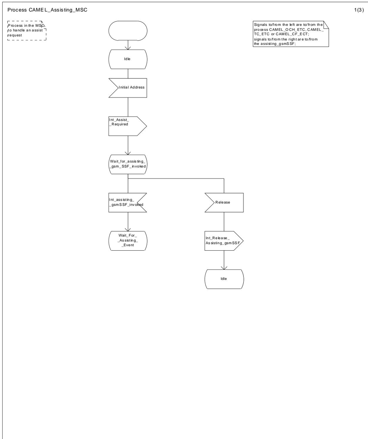
Figure 53a: Process CAMEL\_Assisting\_MSC (sheet 1)
