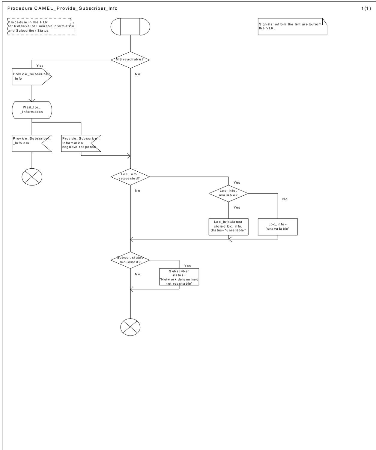
Figure 55a: Procedure CAMEL\_Provide\_Subscriber\_Info (sheet 1)
