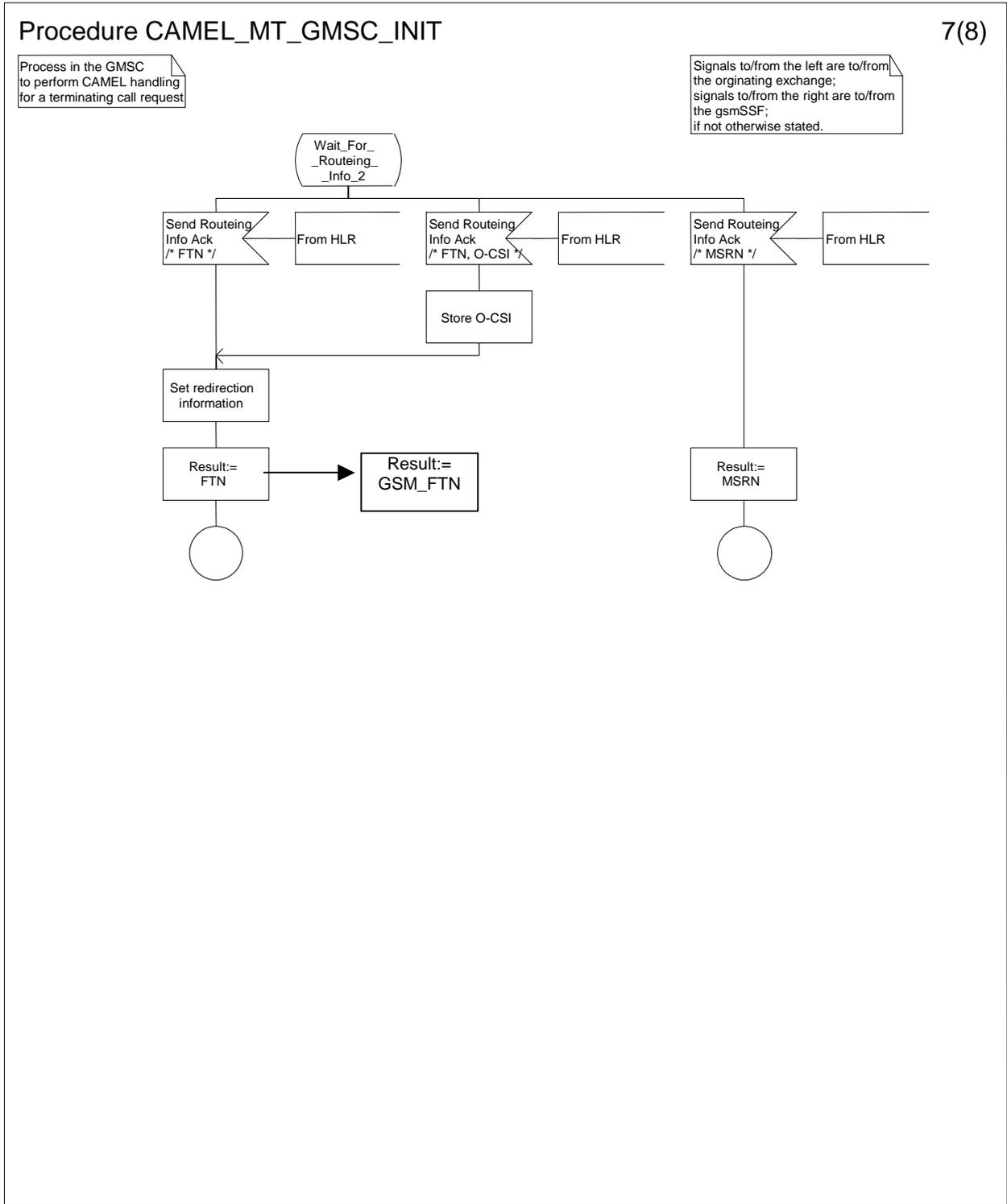
Figure 24g: Procedure CAMEL\_MT\_GMSC\_INIT (sheet 7)
