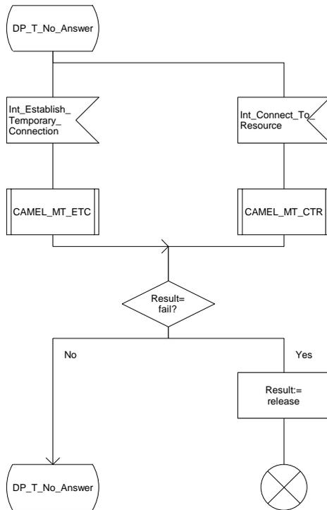
Figure 29b: Procedure CAMEL\_MT\_GMSC\_DISC5 (sheet 2)
