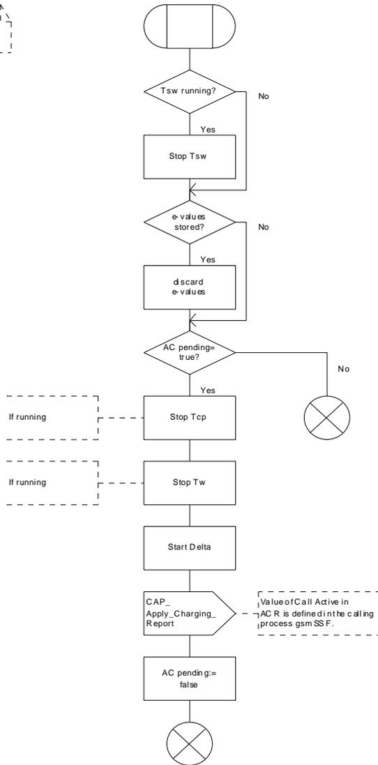
Figure 48a: Procedure Handle\_ACR (sheet 1)
