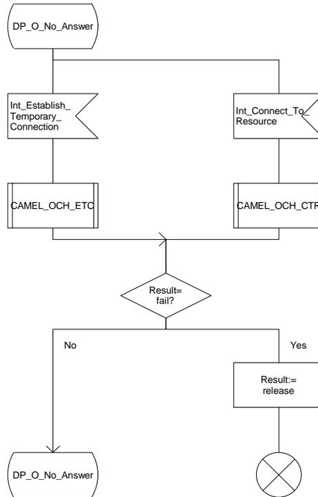
Figure 13c: Procedure CAMEL\_OCH\_MSC2 (sheet 3)
