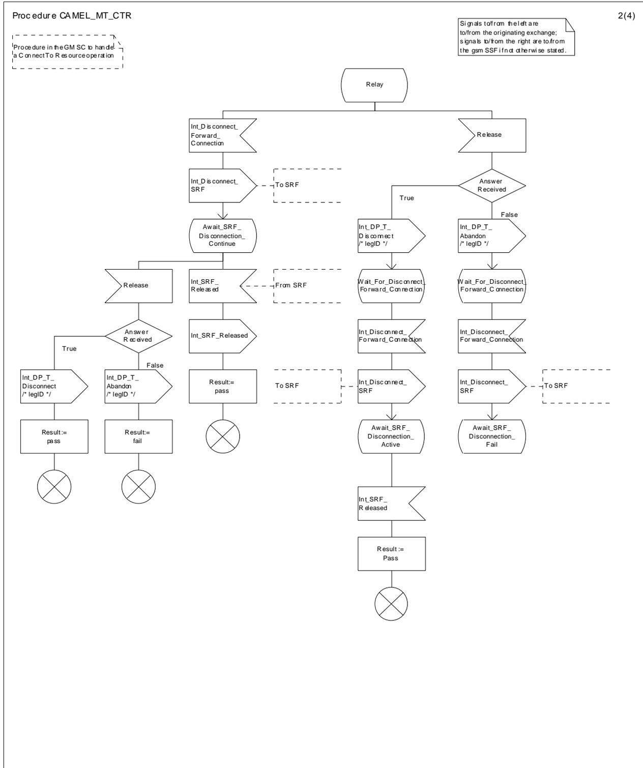
Figure 32b: Procedure CAMEL\_MT\_CTR (sheet 2)
