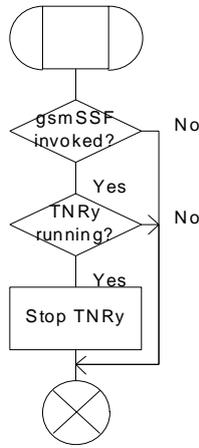
Figure 20a: Procedure CAMEL\_Stop\_TNRy (sheet 1)
