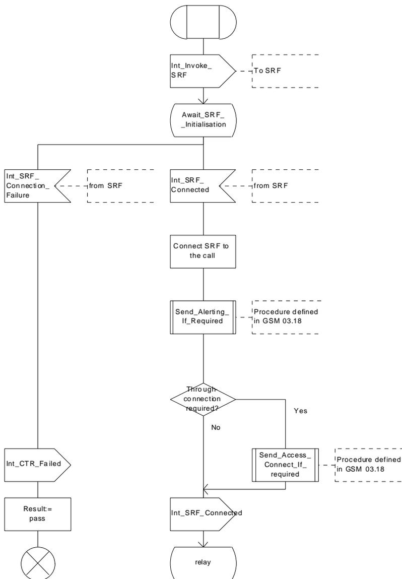
Figure 18a: Procedure CAMEL\_OCH\_CTR (sheet 1)
