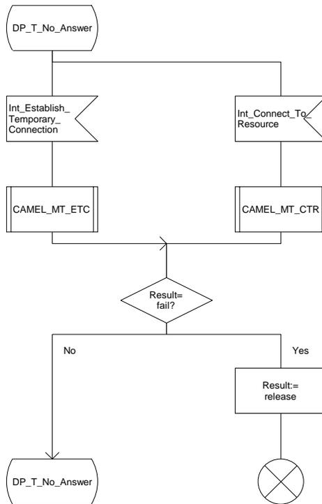
Figure 29b: Procedure CAMEL\_MT\_GMSC\_DISC5 (sheet 2)
