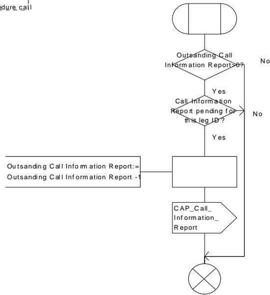
Figure 50a: Procedure Handle\_CIR\_leg (sheet 1)
