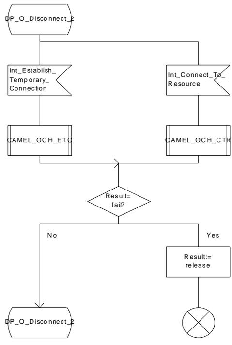
Figure 15b: Procedure CAMEL\_OCH\_MSC\_DISC2 (sheet 2)
