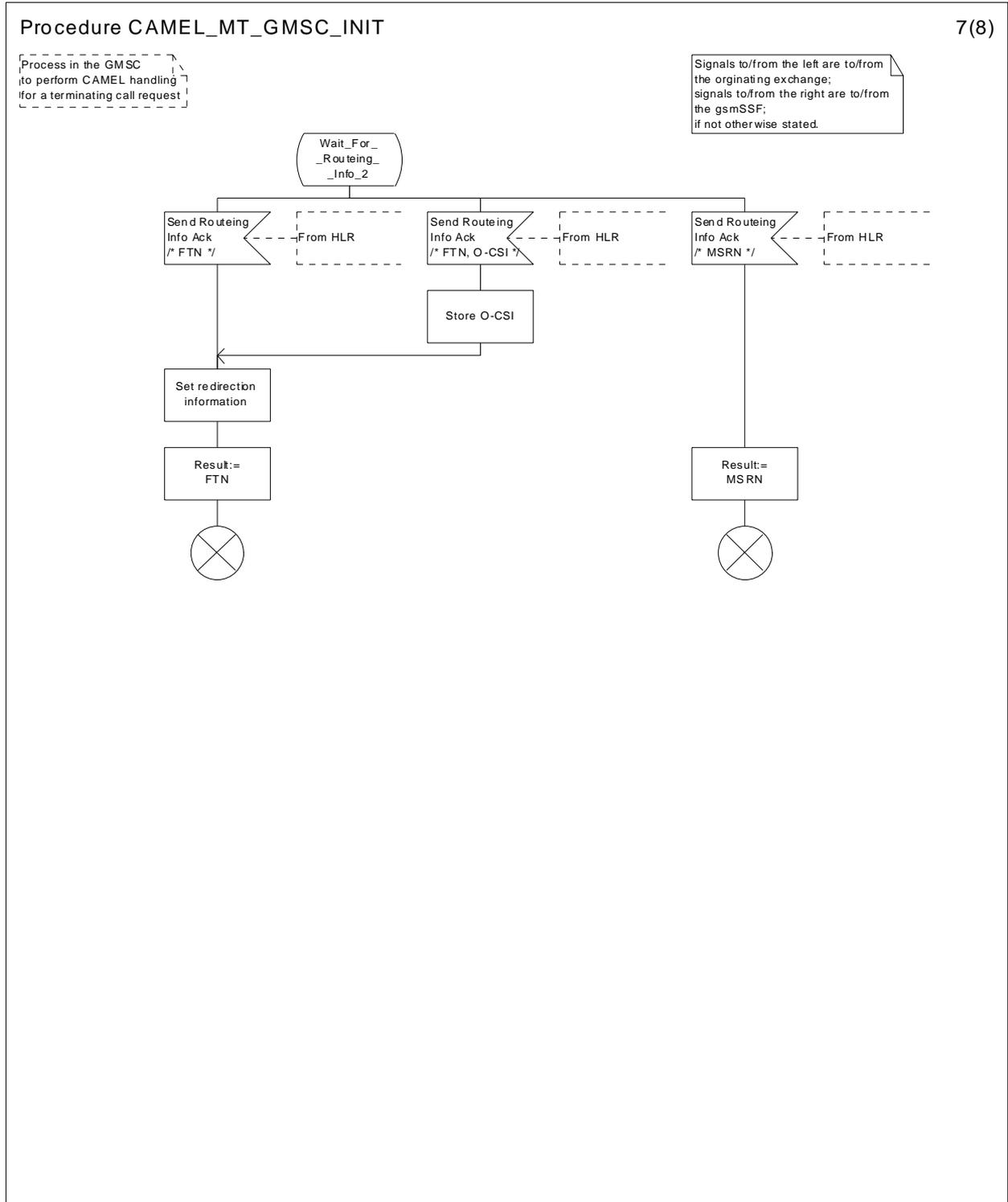
Figure 24g: Procedure CAMEL\_MT\_GMSC\_INIT (sheet 7)
