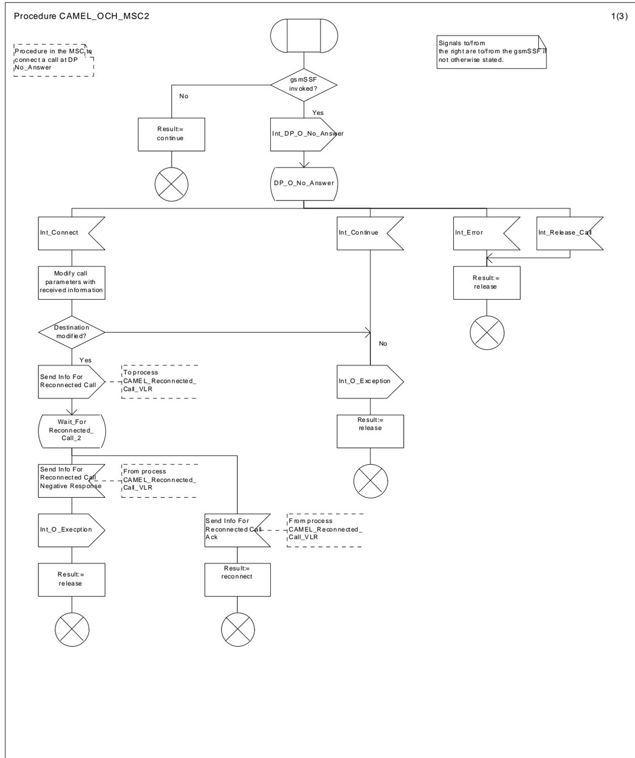
Figure 13a: Procedure CAMEL\_OCH\_MSC2 (sheet 1)
