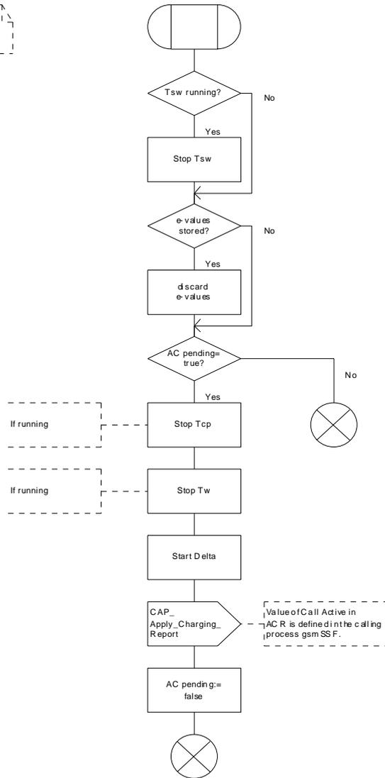
Figure 48a: Procedure Handle\_ACR (sheet 1)
