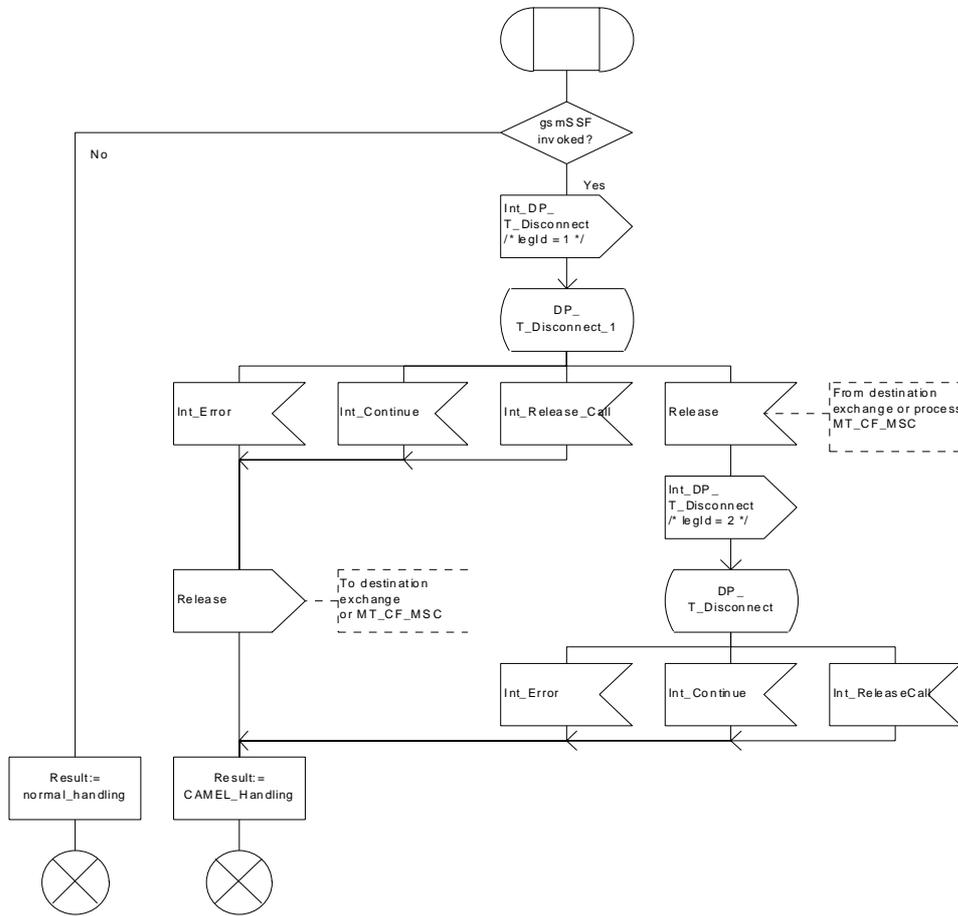
Figure 26a: Procedure CAMEL\_MT\_GMSC\_DISC1 (sheet 1)
