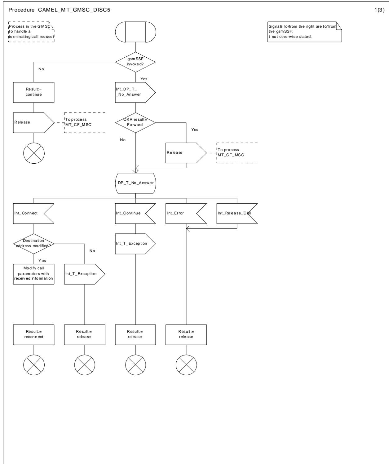
Figure 29a: Procedure CAMEL\_MT\_GMSC\_DISC5 (sheet 1)
