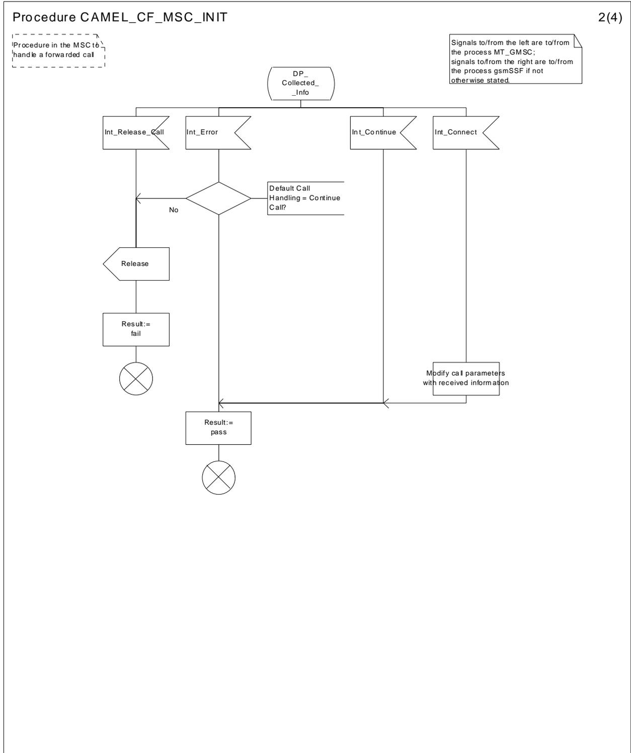
Figure 39b: Procedure CAMEL\_CF\_MSC\_INIT (sheet 2)
