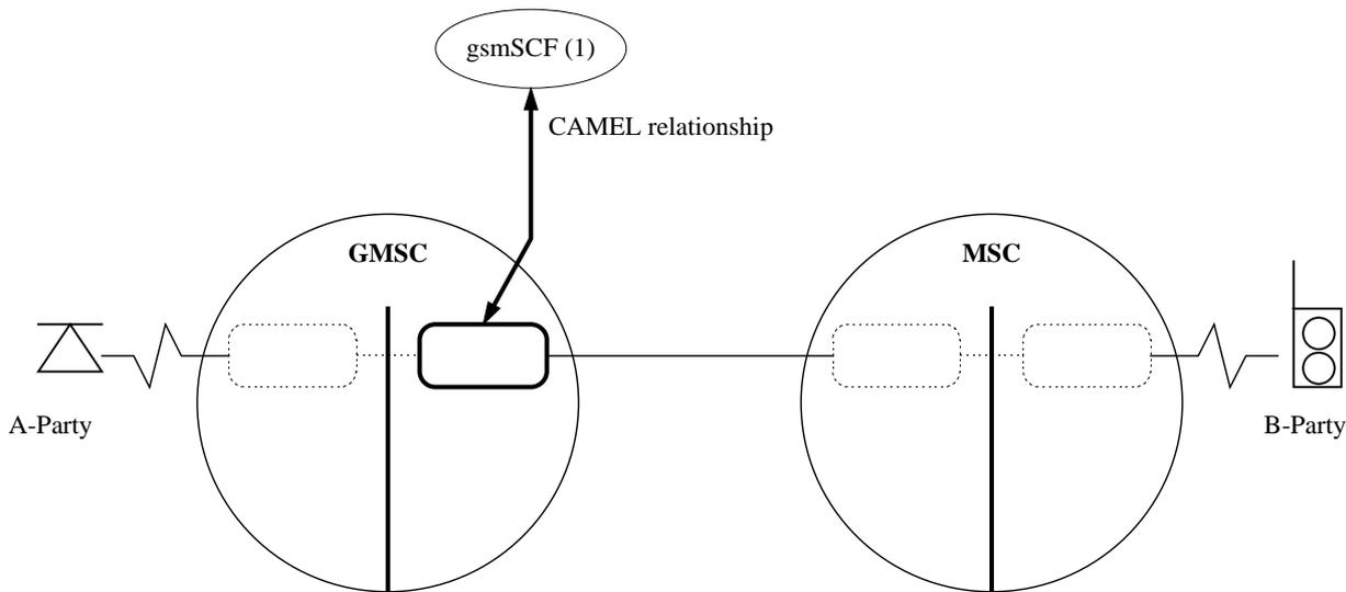
Figure 6: BCSM Scenario for Mobile Terminated Calls
