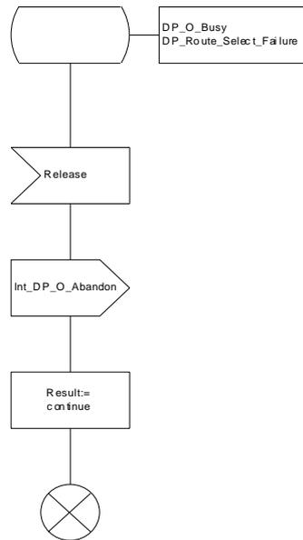
Figure 12b: Procedure CAMEL\_OCH\_MSC1 (sheet 2)
