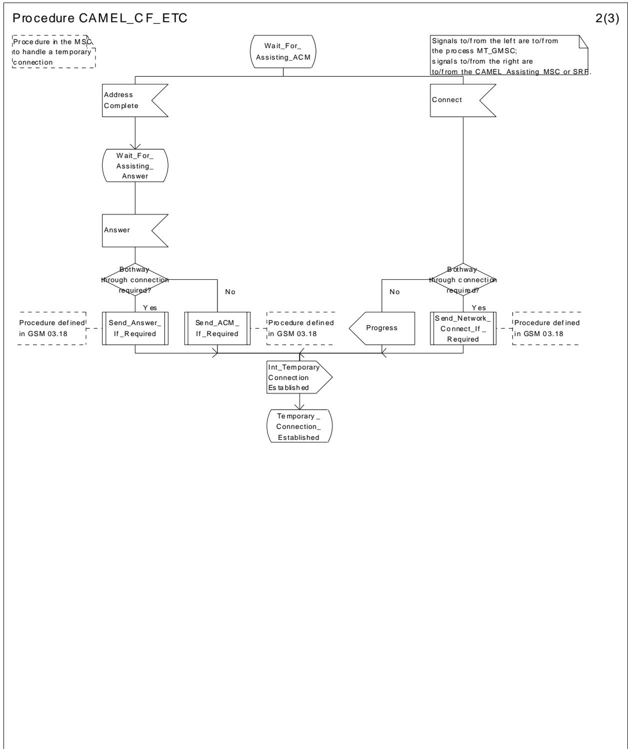
Figure 41b: Procedure CAMEL\_CF\_ETC (sheet 2)
