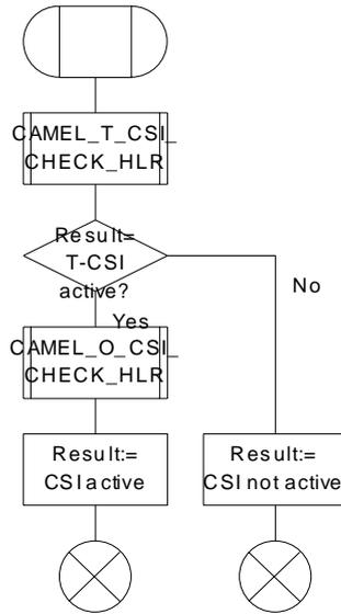
Figure 35a: Procedure CAMEL\_CSI\_Check\_HLR (sheet 1)
