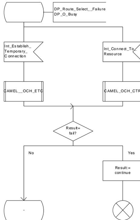
Figure 12c: Procedure CAMEL\_OCH\_MSC1 (sheet 3)
