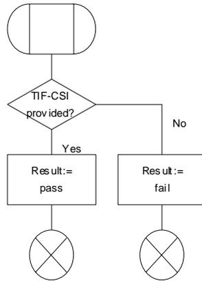
Figure 58a: Procedure CAMEL\_Check\_CF\_Interaction (sheet 1)
