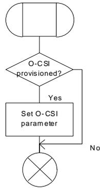
Figure 36a: Procedure CAMEL\_O\_CSI\_CHECK\_HLR (sheet 1)
