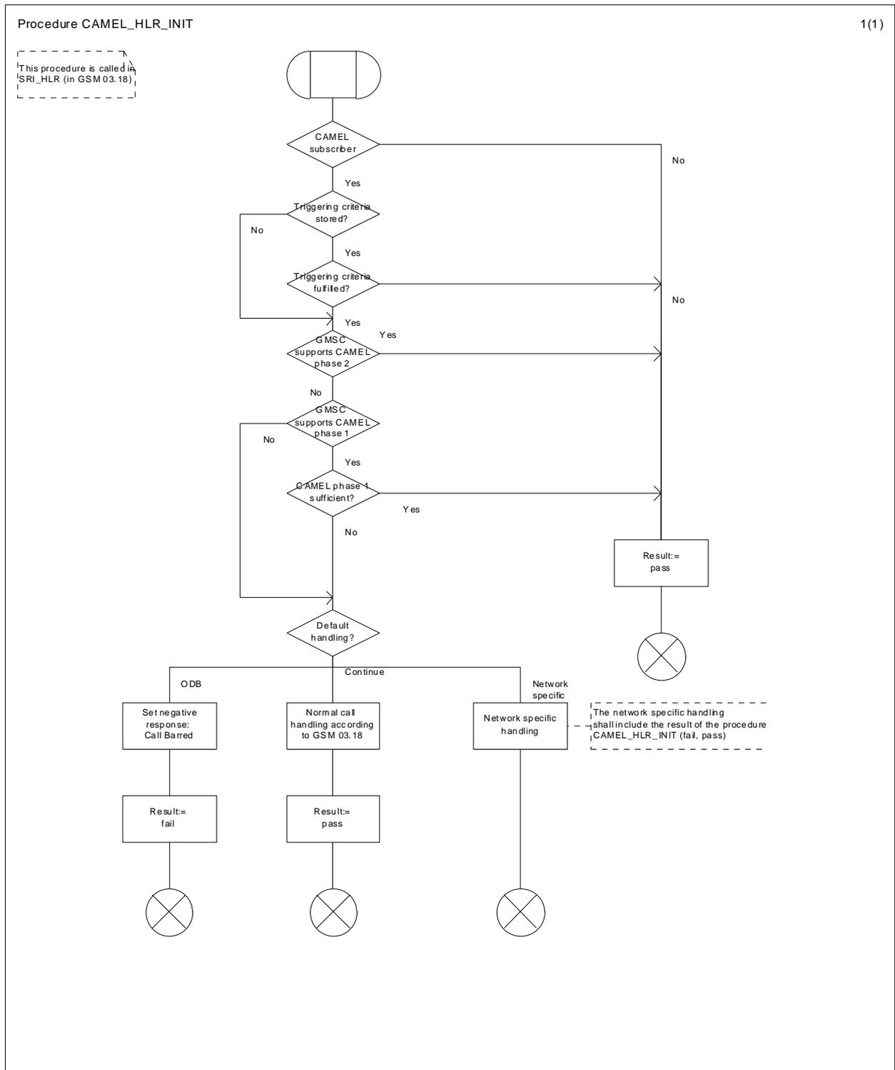
Figure 34a: Procedure CAMEL\_HLR\_INIT (sheet 1)
