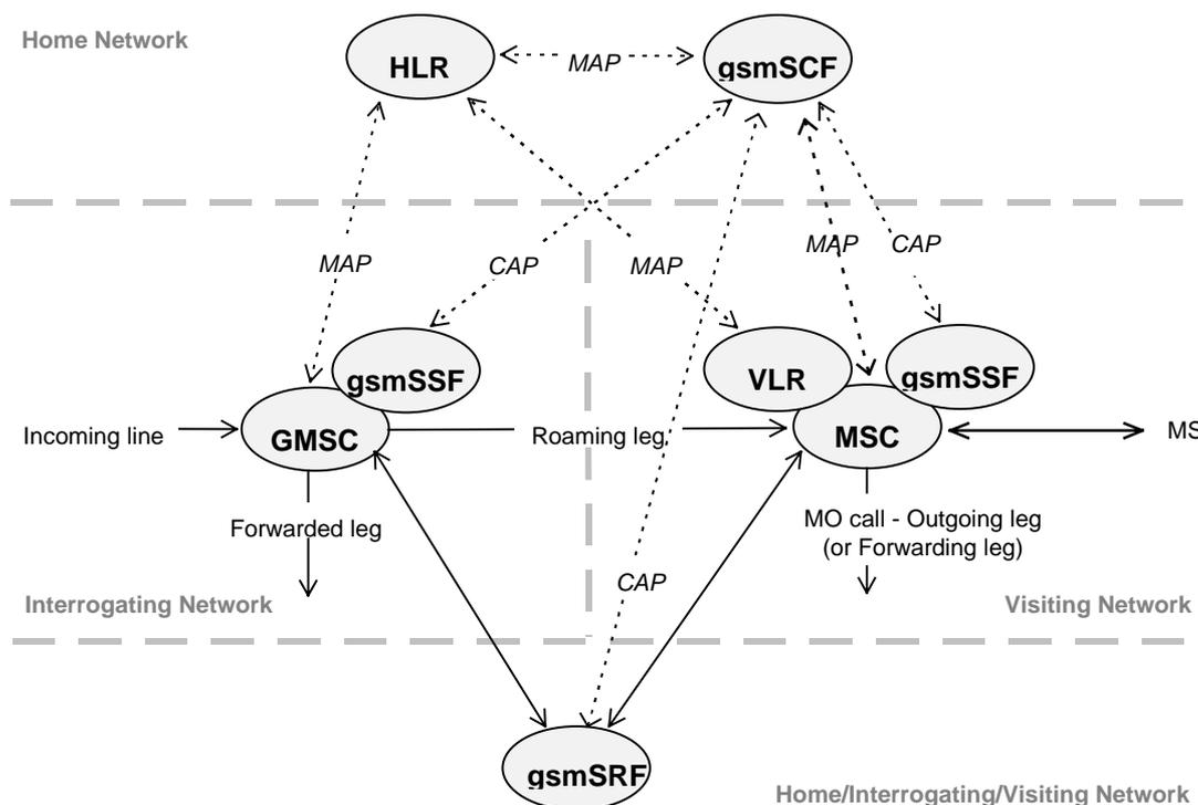
**Figure 1: Functional architecture for support of CAMEL**
