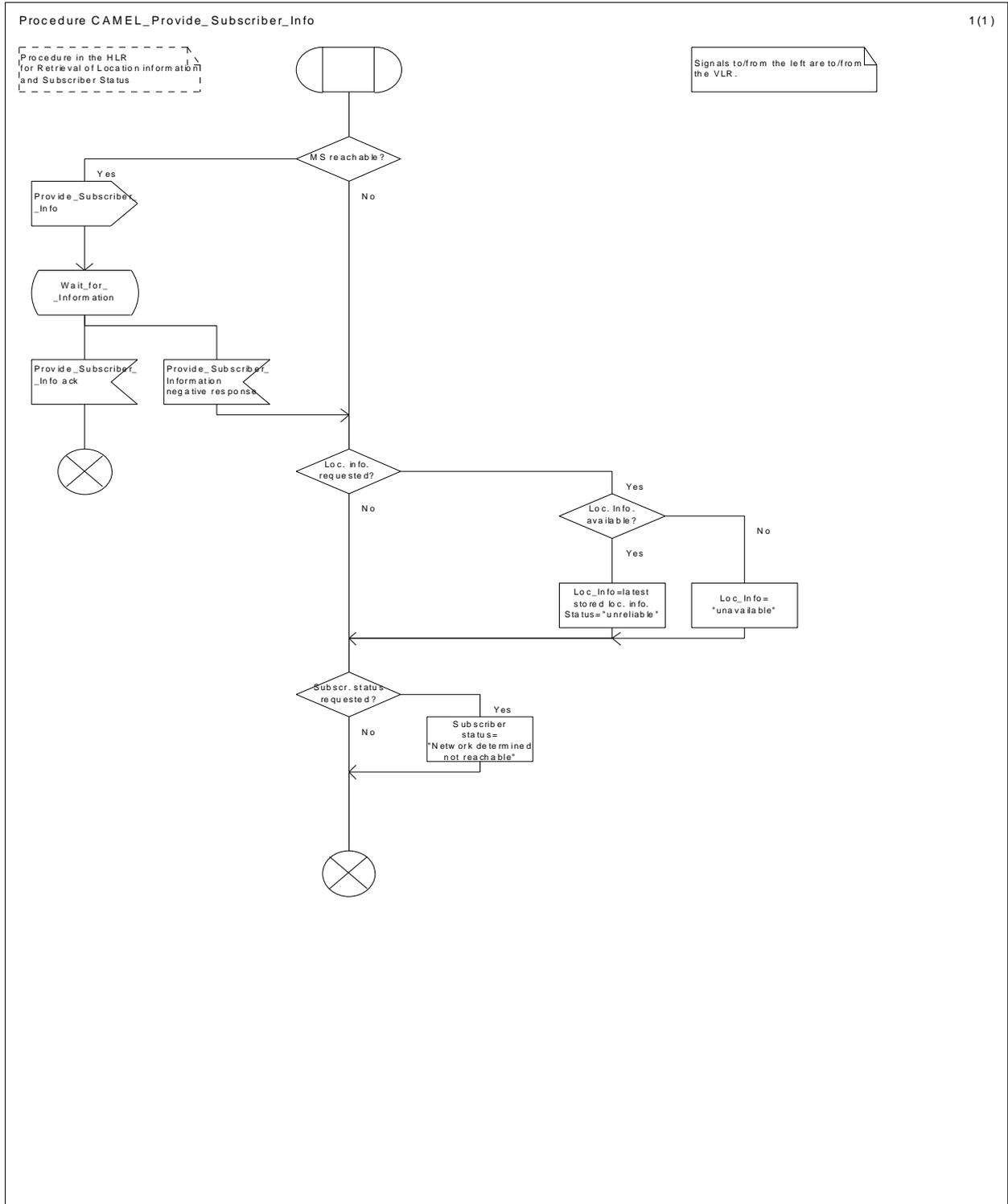
Figure 55a: Procedure CAMEL\_Provide\_Subscriber\_Info (sheet 1)
