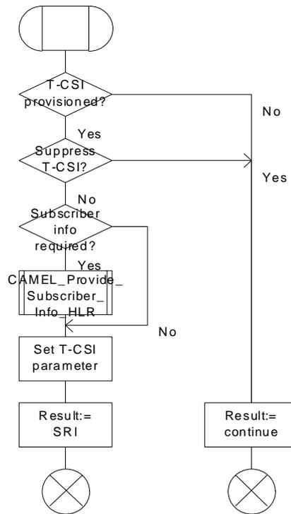
Figure 37a: Procedure CAMEL\_T\_CSI\_CHECK\_HLR (sheet 1)
