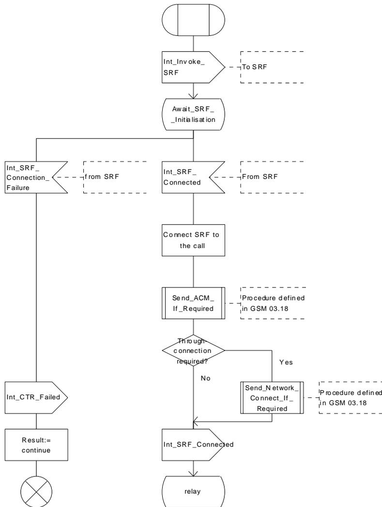
Figure 32a: Procedure CAMEL\_MT\_CTR (sheet 1)
