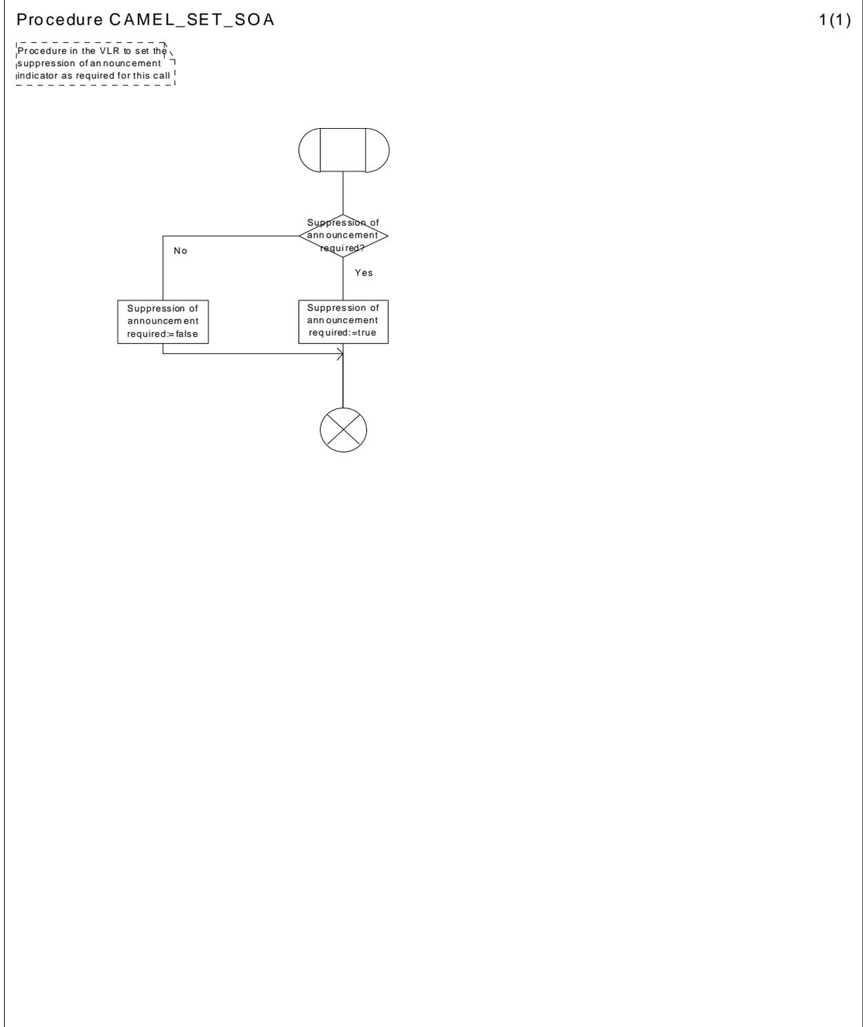
Figure 38a: Procedure CAMEL\_SET\_SOA (sheet 1)
