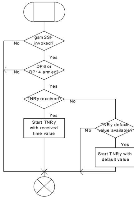
Figure 19a: Procedure CAMEL\_Start\_TNRy (sheet 1)
