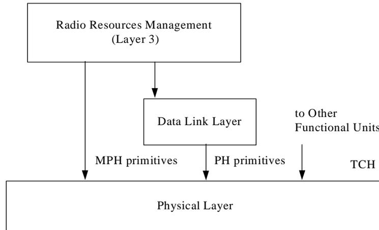
**Figure 4.1: Interfaces with the physical layer**
