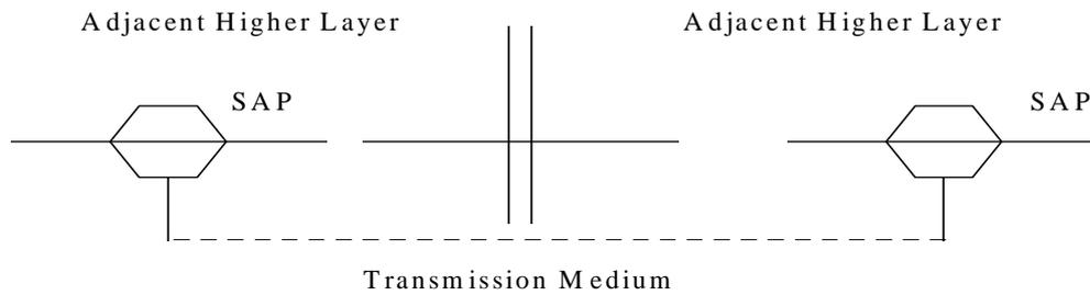
**Figure 5.1.1: Service access point concept**
