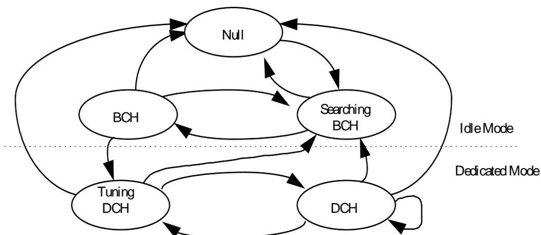
Figure 7.1: States of the physical layer in the MES
