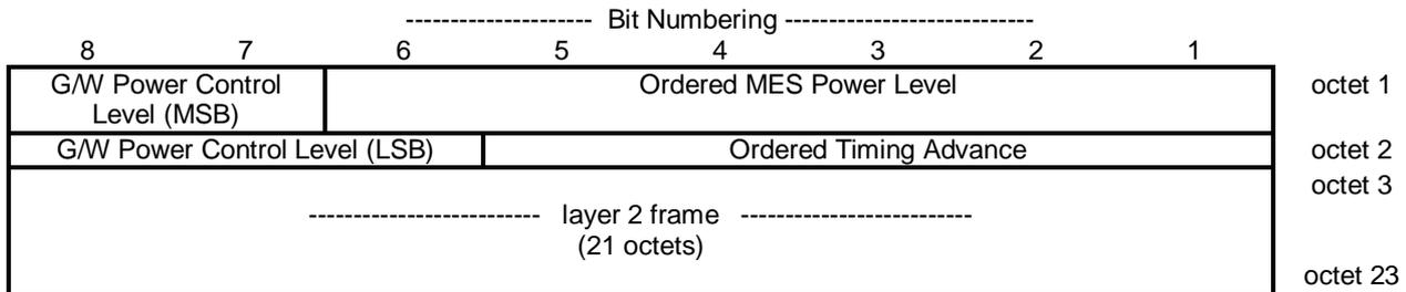
**Figure 9.1.1: S-SACCH forward block format**
