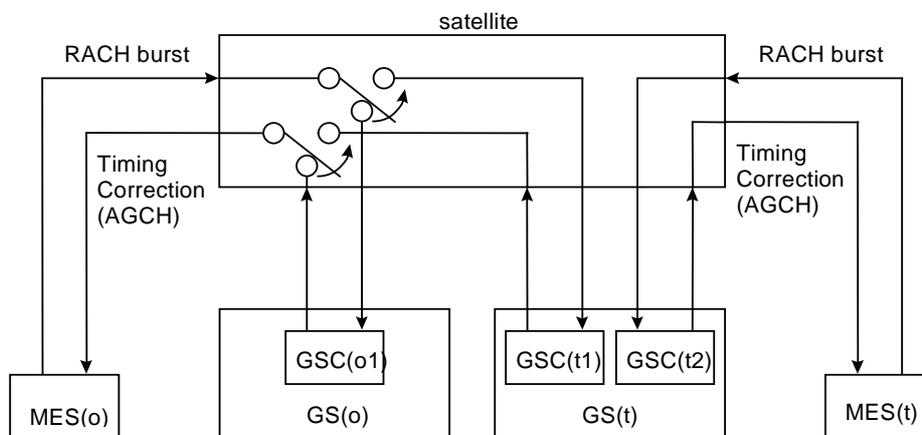
Figure 8.2: Initial timing synchronization for a TtT call
