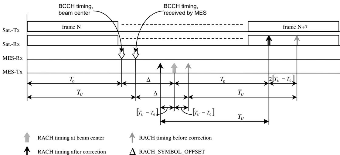
**Figure 5.1: Initial timing synchronization process**
