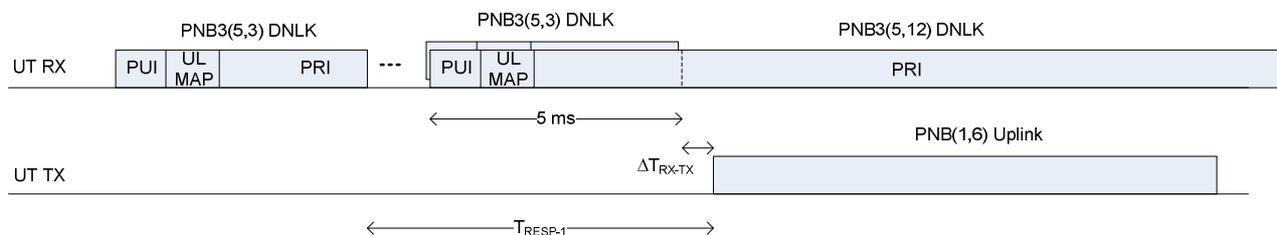
**Figure 5.4: Terminal can receive either a 5 ms or a 20 ms burst on the downlink prior to the start of its scheduled transmission on the uplink**
