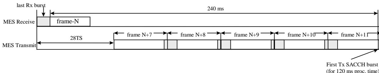
**Figure D.2: The longest available MES processing time, MES on subsatellite point, for SACCH message**
