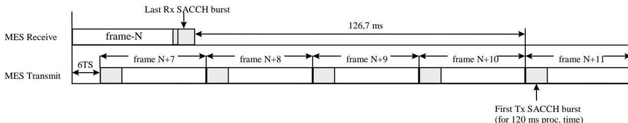
**Figure D.1: The worst-case available at processing time, MES with the lowest elevation, for SACCH message**
