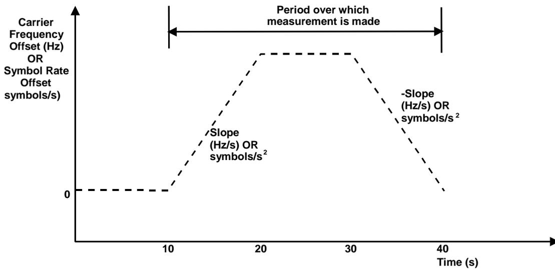
Figure 5.2: Frequency and symbol rate offset profile
