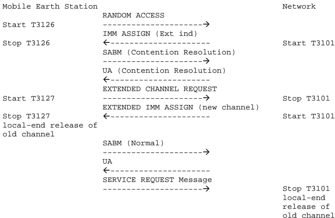
Figure 4.2: Extended immediate assignment procedure
