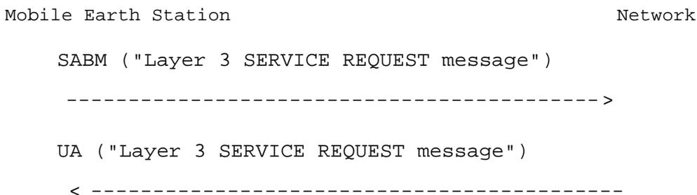
**Figure 4.1: Service request and contention resolution using layer 3 message**
