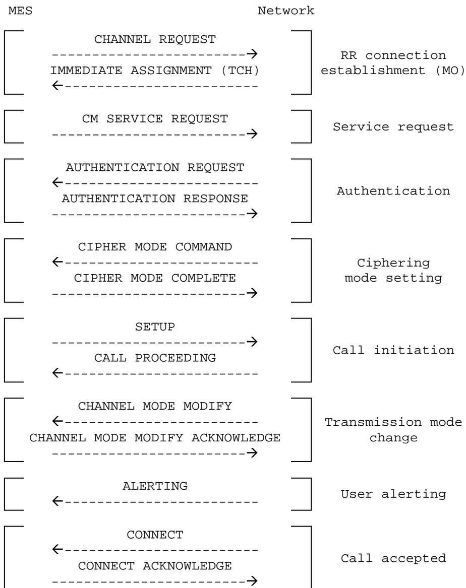
Figure 8.5: Mobile Originating Call Establishment with Very Early Assignment
