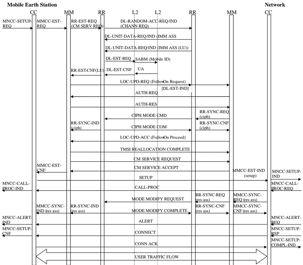
Figure A.8: Mobile-originated call setup with optimal routing. Successful case (see GMR-1 03.297[3])
