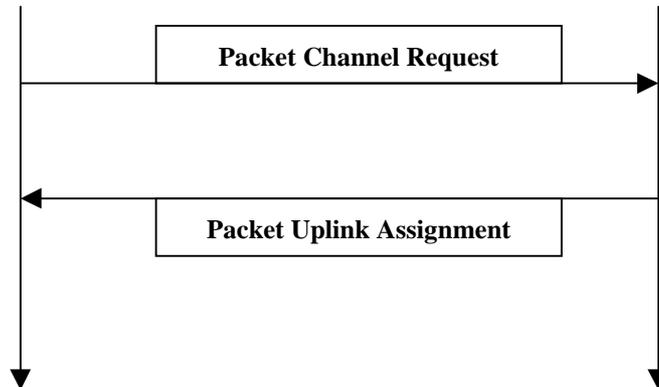
**Figure 7: Access and allocation for the packet access, uplink packet transfer**
