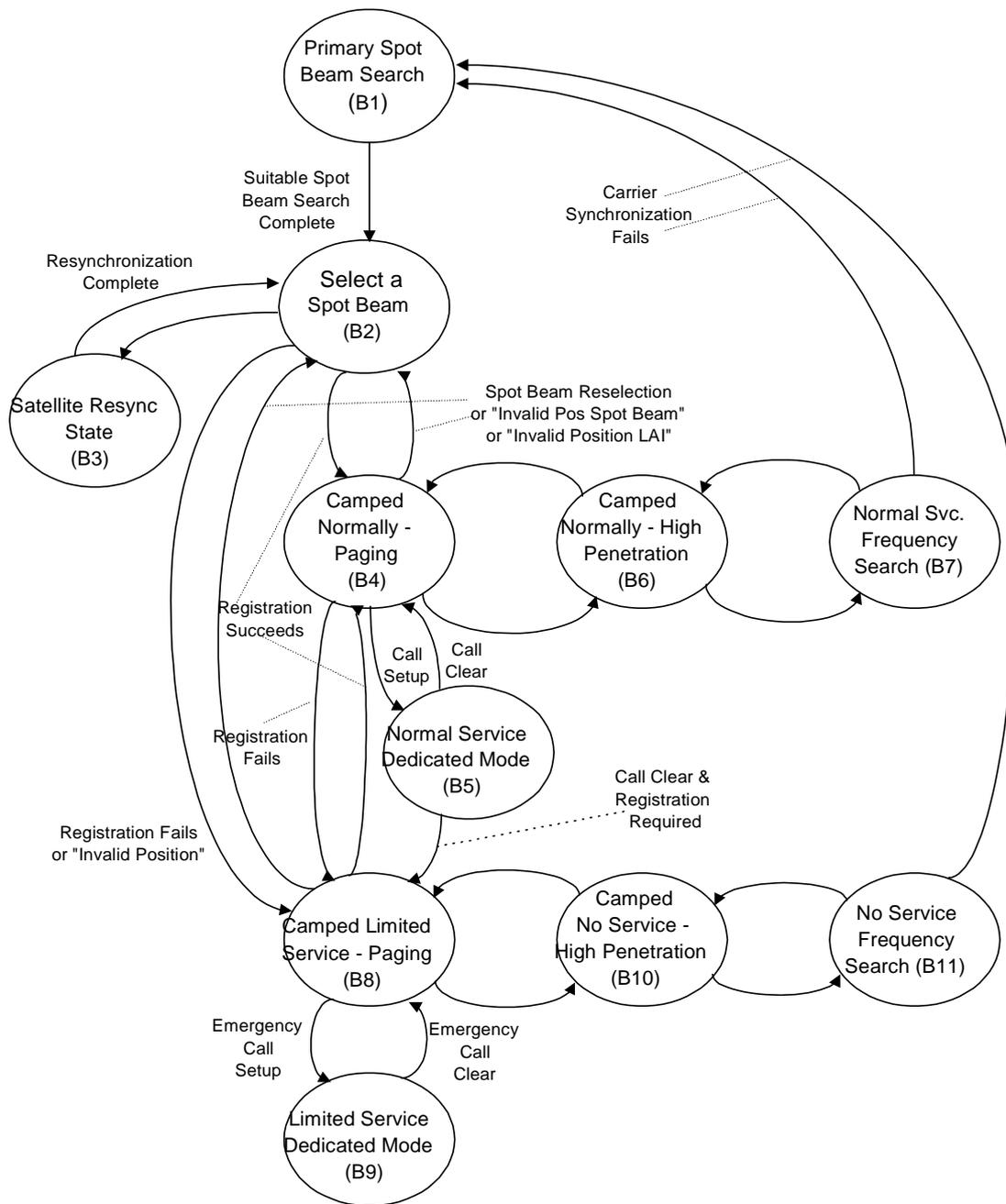
Figure 6.2: Spot beam selection process
