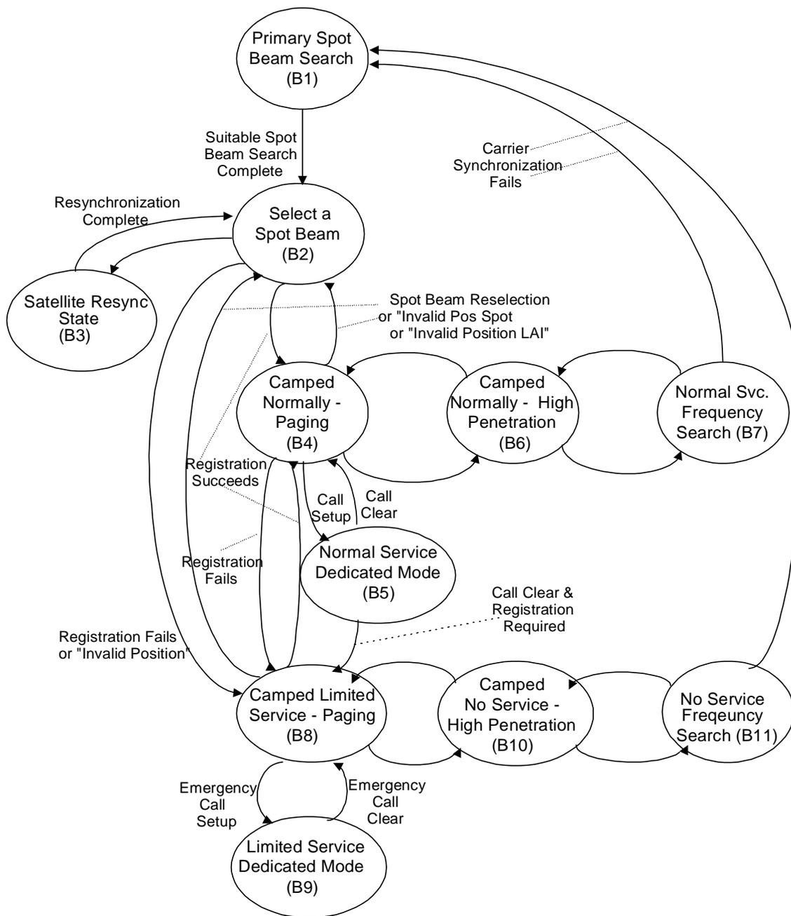
Figure 6.2: Spot beam selection process
