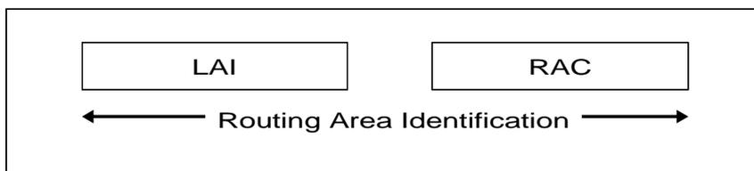
**Figure 8.2: Structure of Routing Area Identification (RAI)**
