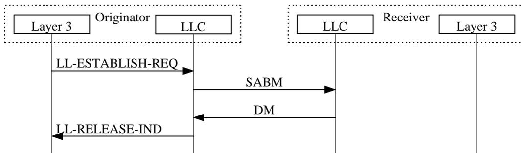
Figure 15: Layer 3-initiated ABM establishment procedure, unsuccessful
