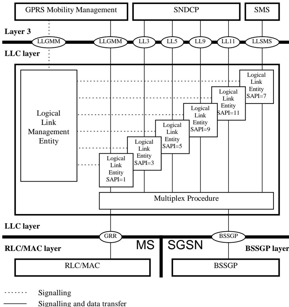
Figure 2: Functional model of the LLC layer
